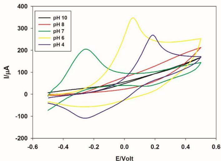
**Figure 2.** Cyclic voltammograms of GC/poly(ANI-co-PY)/Pd in 5 mM hydrazine/phosphate buffer solutions at different pH values, at a scan rate of  $50 \text{ mV}\cdot\text{s}^{-1}$ .
