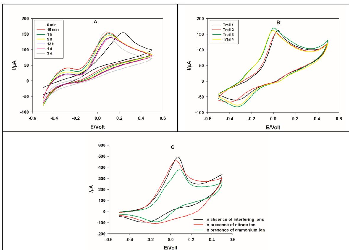
**Figure 5.** Cyclic voltammograms of GC/poly(ANI-co-PY)/Pd in 5 mM hydrazine/phosphate buffer at pH = 6, a scan rate of  $50 \text{ mV}\cdot\text{s}^{-1}$ , (A) at different test times, (B) using freshly prepared sensor each time before testing, and (C) in the absence and presence of interfering ions, and nitrate and ammonium ions.
