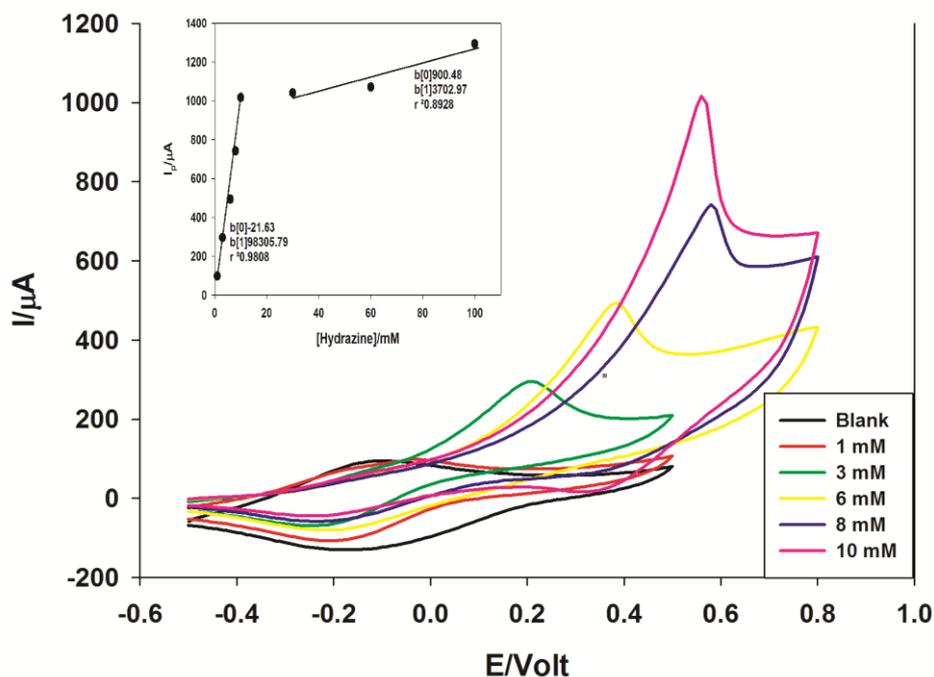
**Figure 4.** Cyclic voltammograms of GC/poly(ANI-co-PY)/Pd in the absence and presence of different hydrazine concentrations, 1 mM to 0.1 M, in phosphate buffer at pH = 6, a scan rate of  $50 \text{ mV} \cdot \text{s}^{-1}$ . The inset represents the calibration curve.
