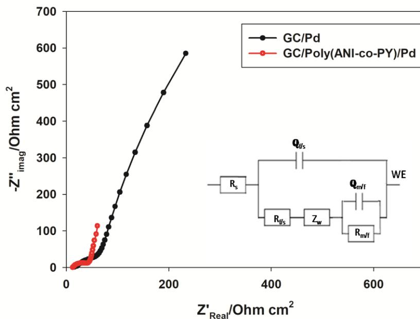
**Figure 6.** Nyquist plots in 5 mM hydrazine/phosphate buffer at pH = 6 for GC/Pd and GC/poly(ANI-co-PY)/Pd electrodes, for comparison.
