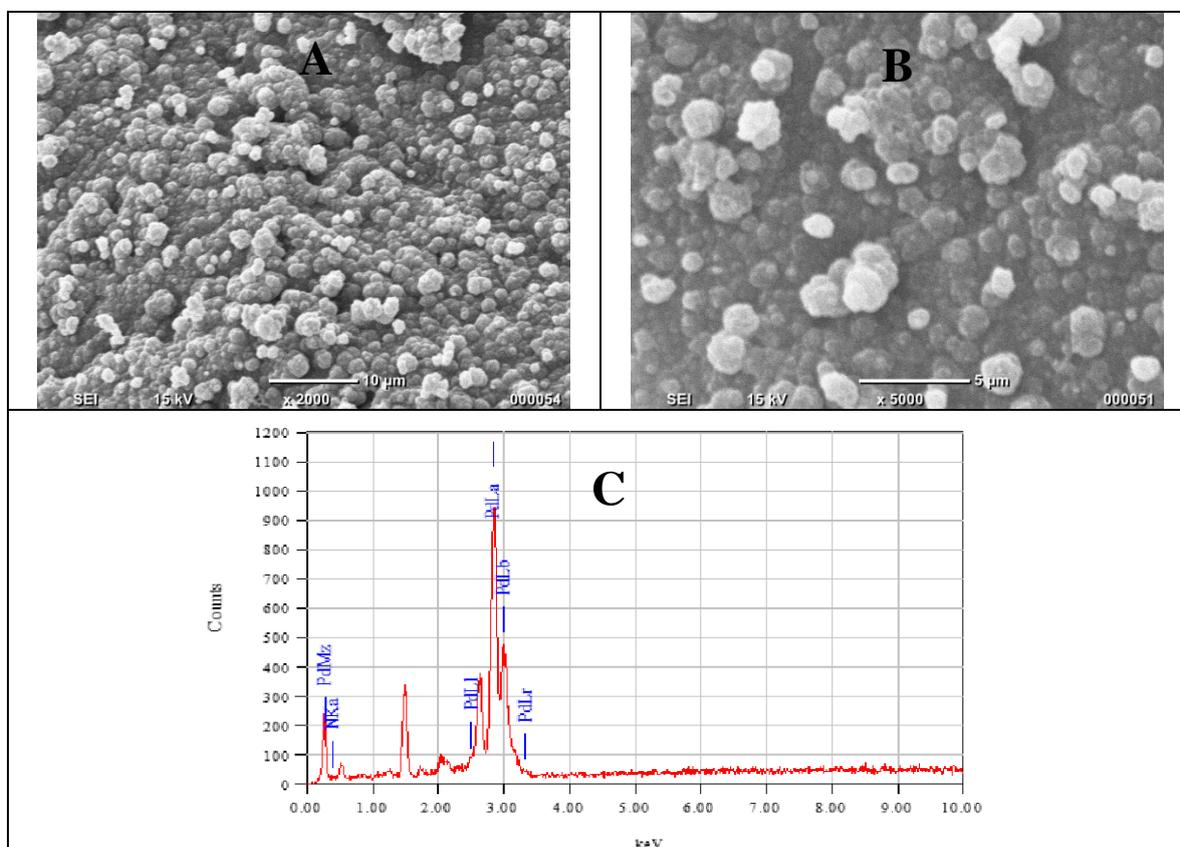
**Figure 7.** SEM images of the poly(ANI-co-PY)/Pd composite with a magnification of (A) 2000 $\times$  and (B) 5000 $\times$ ; and (C) EDXA spectrum of the composite.
