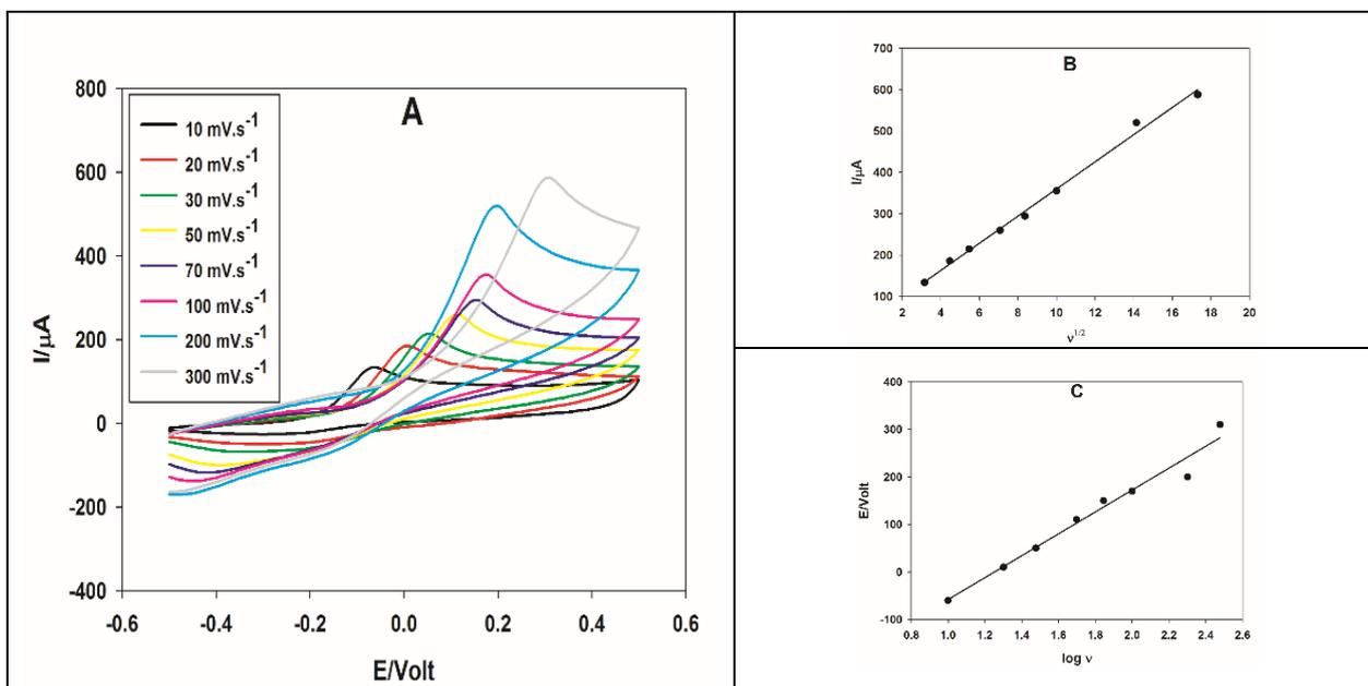
**Figure 3.** (A) Cyclic voltammograms of GC/poly(ANI-co-PY)/Pd in 5 mM hydrazine/phosphate buffer solutions at pH = 6 at different scan rates of 10–300  $\text{mV}\cdot\text{s}^{-1}$ ; (B) a plot of  $I_p$  vs.  $v^{1/2}$ ; and (C) a plot of  $E_p$  vs.  $\log v$ .
