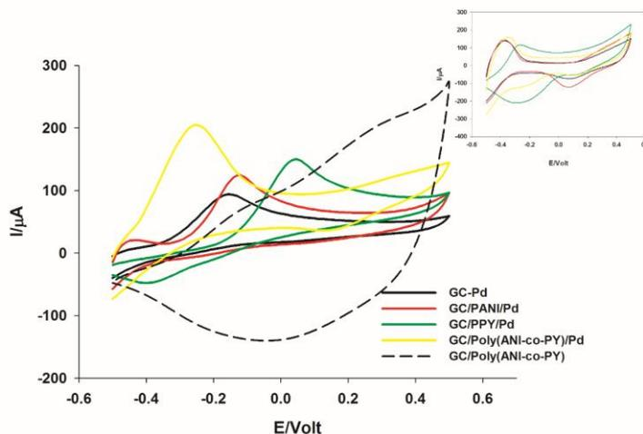
**Figure 1.** Cyclic voltammograms of different based-Pd catalysts in 5 mM hydrazine/phosphate buffer solution (pH = 7), a scan rate of  $50 \text{ mV}\cdot\text{s}^{-1}$ . The inset represents the response of different catalysts in the buffer.
