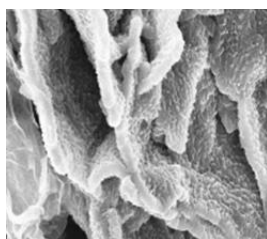
Figure 4. the SEM of PANI/MnO 2 /Graphene composites
