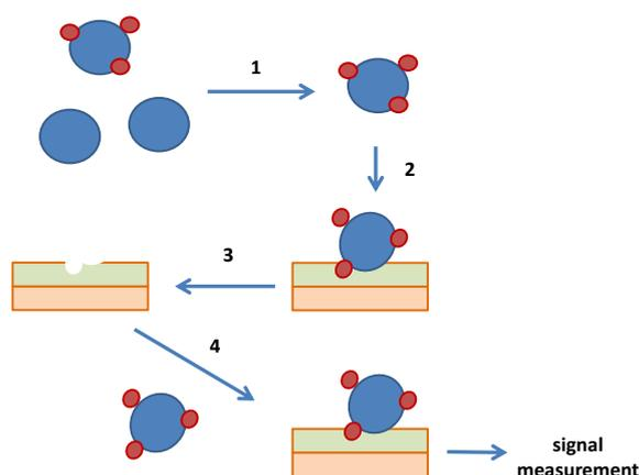
**Figure 1.** Description of imprinting procedure; 1 – isolation of target molecule; 2 – imprinting of fragments into polymer (light green) and anchoring of the polymer on a sensor surface (pink); 3 – remove of template molecule; 4 – interaction of MIP based sensor with analyte molecule.
