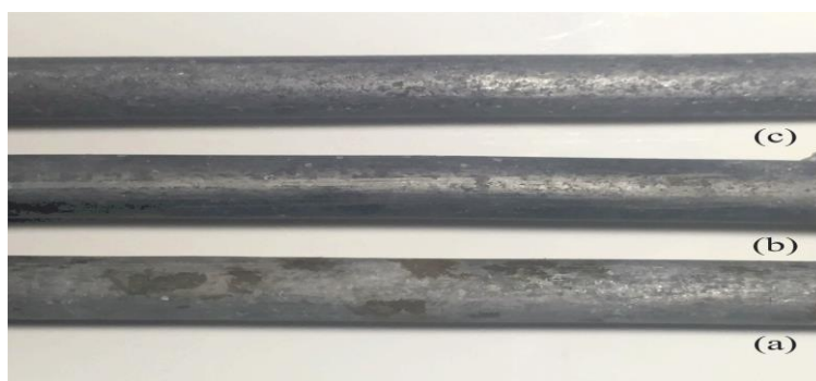
Figure 11. Visual inspection images of steels in the mortar before the ECE treatment (a), after the ECE treatment with the special electrode configuration (b) and after the ECE treatment with the traditional electrode configuration (c).
