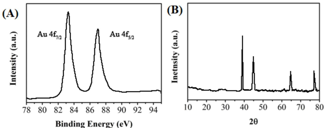
**Figure 2.** (A) High resolution Au 4f scan and (B) XRD image of the bioformed Au nanoparticles.
