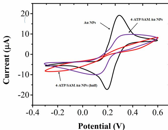
**Figure 3.** CV of an original Au electrode and SAMs onto it, indicating current ( $I/\mu\text{A}$ ) as a function of potential in 10 mM  $\text{K}_3\text{Fe}(\text{CN})_6/\text{K}_4\text{Fe}(\text{CN})_6$  in PBS with a pH of 7.0 and a scan rate of 50 mV/s.
