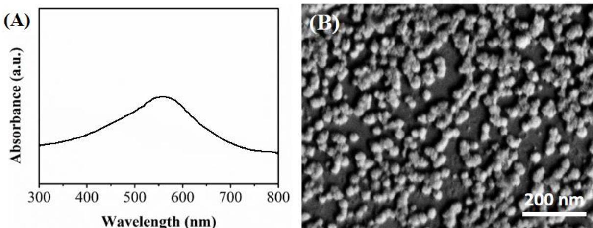
**Figure 1.** (A) UV-vis spectrum and (B) SEM pattern of biosynthesized AuNPs.
