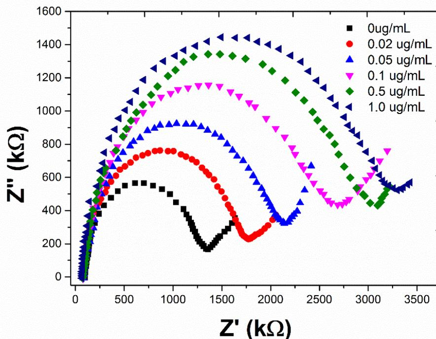
**Figure 5.** Faradaic impedance spectra of the antibody fragments/4-ATP SAM/Au electrode for various concentrations of myoglobin in PBS (pH 7.4) with 0.1 M KCl solution containing 2 mM  $[\text{Fe}(\text{CN})_6]^{3-/4-}$ .
