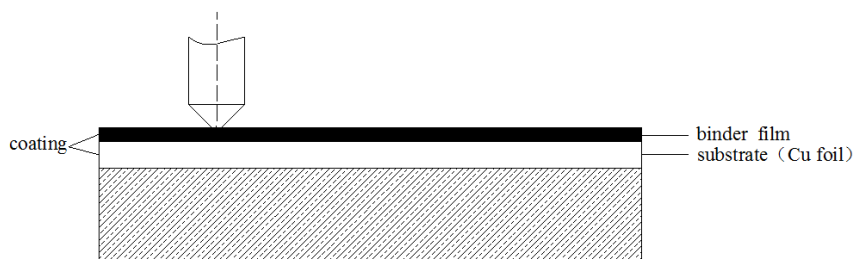
Figure 2. The mechanical model of coating scratch test.
