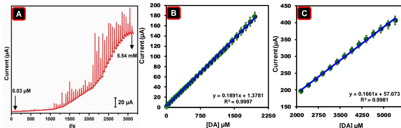
**Figure 3.** (A) amperometric response of the MWCNTs/MoS<sub>2</sub>-Co<sub>3</sub>O<sub>4</sub> modified electrode (rotation speed=1200 RPM) upon successive injections of DA into PB (pH 7) at a regular intervals of 50 s ( $E_{app} = +0.34$  V). Well-defined and quick responses were obtained and steady-state current was reached in less than 3 s. (B) and (C) [DA]/ $\mu$ M vs. current ( $\mu$ A).
