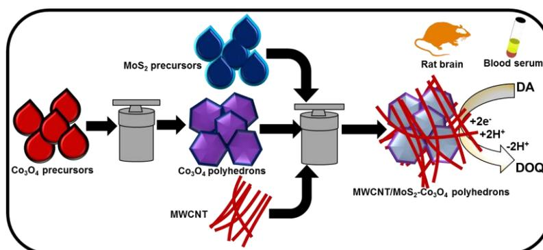
**Figure 1.** Schematic representation for selective detection of dopamine using MWCNTs/ $\text{MoS}_2$ - $\text{Co}_3\text{O}_4$  PHs
