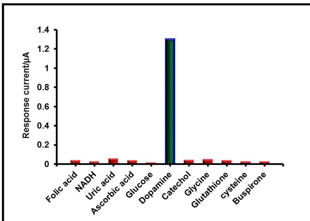
**Figure 4.** (A) Amperometric response of MWCNTs/MoS<sub>2</sub>-Co<sub>3</sub>O<sub>4</sub> PHs film modified electrode towards 2 μM of 4-NP (a), and 0.5 mM of 0.5 mM of folic acid, NADH, uric acid, ascorbic acid, glucose, catechol, glycine, glutathione, cysteine, and buspirone into 0.1 M PB (pH 7.0) electrode rotation speed = 1200 RPM and applied potential = +0.34 V.
