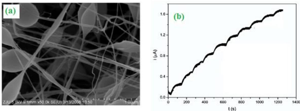
**Figure 4.** (a) SEM images of electrospun nanofibrous membranes of MWCNT filled PANCAA and (b) Chronoamperometric curves with glucose concentrations on the MWCNT-filled PANCAA (PANCAA/MWCNT) nanofibrous membrane deposited electrode. ("Reprinted with permission from (*J. Phys. Chem. C* 113 (2009) 2955-2960). Copyright (2009) American Chemical Society").
