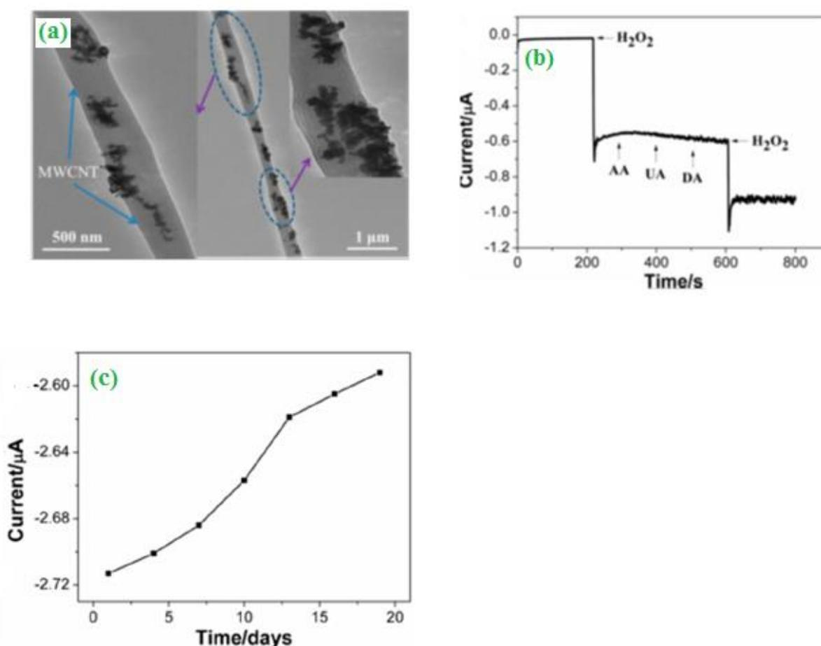
**Figure 5.** (a) TEM photographs of PVDF–MWCNT–PtNP hybrid nanofibers (b) Electrochemical H<sub>2</sub>O<sub>2</sub> selectivity of biosensor and (c) Electrochemical long-term storage stability in response to 5 mM H<sub>2</sub>O<sub>2</sub>. ("Reprinted with permission from *ACS Appl. Mater. Interface* 6 (2014) 7563-7571). Copyright (2014) American Chemical Society").
