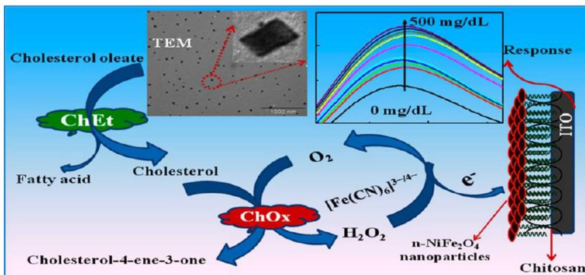
**Figure 2.** Shows the schematic representations of hybrid nanocomposite based on hydrothermally synthesized nanostructured  $\text{NiFe}_2\text{O}_4$  ( $n\text{-NiFe}_2\text{O}_4$ ) and chitosan (CH) has been explored for bienzyme (cholesterol esterase (ChEt) and cholesterol oxidase (ChOx)) immobilization. ("Reprinted with permission from (*J. Phys. Chem. C* 117 (2013) 8491-8502). Copyright (2013) American Chemical Society").
