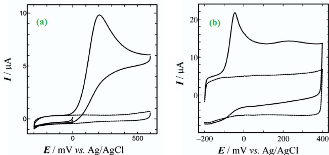
**Figure 3.** Shows typical cyclic voltammogram obtained (a) Graphite-modified and (b) Heat-treated SWNT modified electrodes in 0.10 M phosphate buffer (pH 7.0) in the absence (dotted lines) and presence (solid lines) of 0.5 mM ascorbate. Scan rate, 50 mV s<sup>-1</sup>. ("Reprinted with permission from (*Anal. Chem.*, 77 (2005) 6234-6242). Copyright (2005) American Chemical Society").
