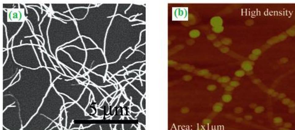
**Figure 1.** (a) and (b) shows SEM and AFM images of carbon nanotubes after exposure to streptavidin. ("Reprinted with permission from (*ACS.Nano* 4 (2010) 6914-6922). Copyright (2010) American Chemical Society").
