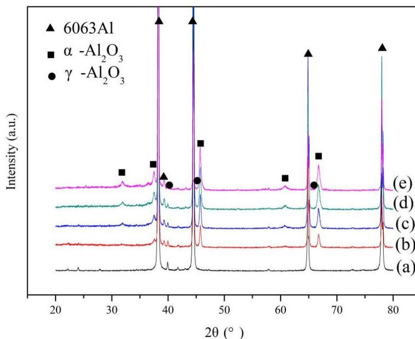
**Figure 4.** X-ray diffraction patterns of (a) bare alloy and PEO coatings formed under the current density of (b) 5; (c) 10; (d) 15; (e) 20 A/dm<sup>2</sup> for 25 min.
