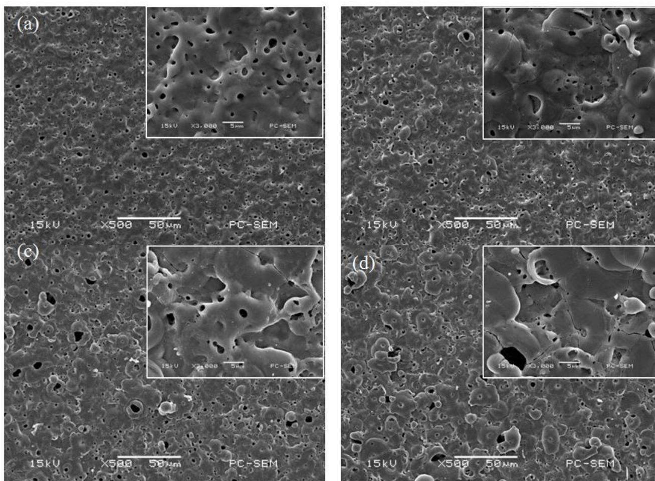
**Figure 1.** Surface morphology of PEO coatings formed under the current density of (a) 5; (b) 10; (c) 15; (d)  $20 \text{ A/dm}^2$  for 25 min.
