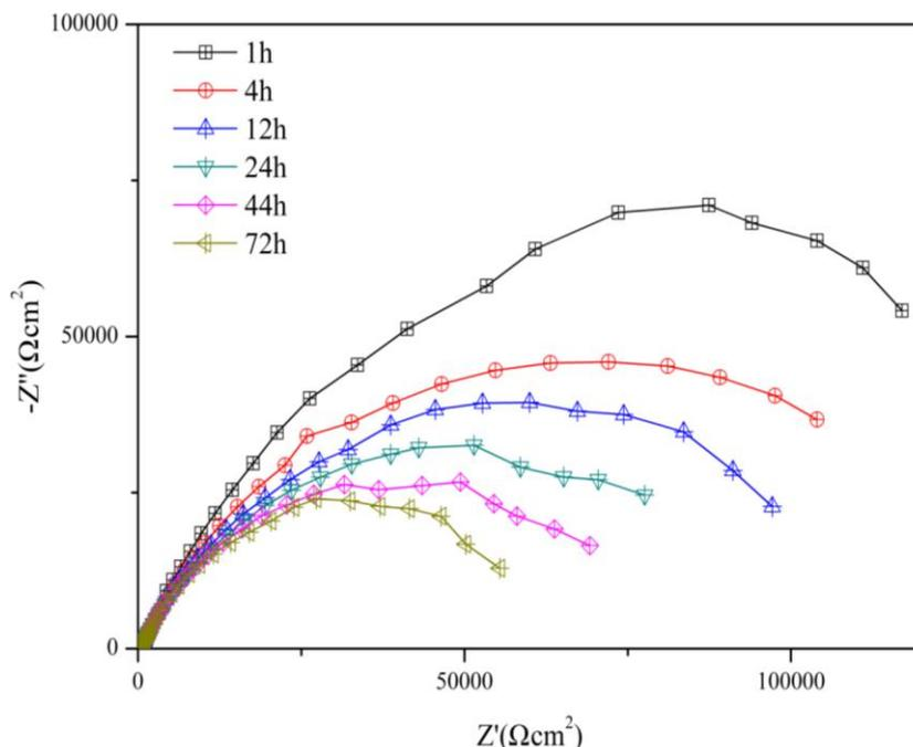
**Figure 6.** Nyquist plots of PEO coated aluminum alloy substrate formed under the current density of 10 A/dm<sup>2</sup> immersed in 0.59 M NaCl solution for different times. The fitting equivalent circuits is shown in Fig. 8b and symbols correspond to the experimental values.
