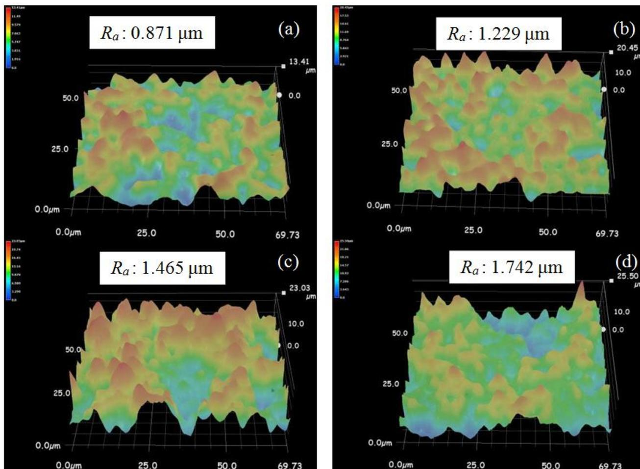
**Figure 2.** 3D image of PEO coatings formed under the current density of (a) 5; (b) 10; (c) 15; (d) 20 A/dm<sup>2</sup> for 25 min.
