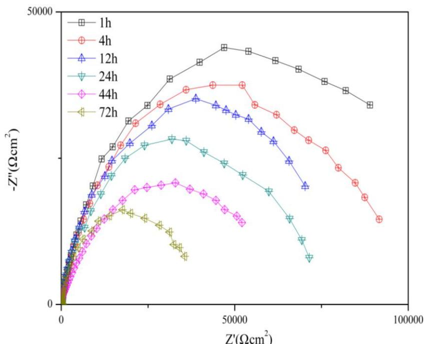
**Figure 7.** Nyquist plots of uncoated aluminum alloy immersed in 0.59 M NaCl solution for different times. The fitting equivalent circuits is shown in Fig. 8a and symbols correspond to the experimental values.
