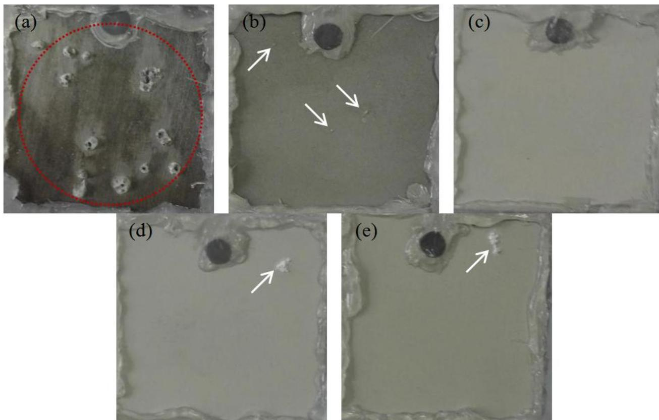
**Figure 9.** The optical appearance of specimens after salt solution immersion test in 2 M NaCl solution for 10 days: (a) uncoated aluminum alloy and PEO coatings produced under the current density of (b) 5; (c) 10; (d) 15; (e) 20 A/dm<sup>2</sup> for 25 min. The obvious corrosion area are marked by red circles.
