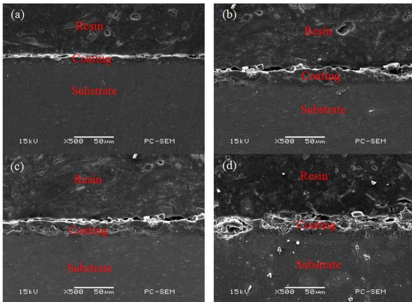
**Figure 3.** Cross-sectional morphology of PEO coatings formed under the current density of (a) 5; (b) 10; (c) 15; (d)  $20 \text{ A/dm}^2$  for 25 min.
