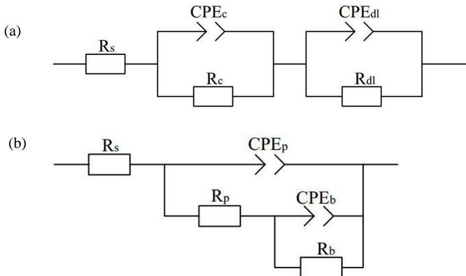
**Figure 8.** Corresponding equivalent circuits for fitting the impedance data of (a) uncoated and (b) PEO coated aluminum alloy.
