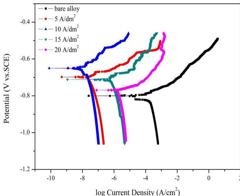
**Figure 5.** Potentiodynamic polarization curves of uncoated and PEO coated aluminum alloy in 0.59 M NaCl solution. PEO coatings were formed under the current density of 5, 10, 15, 20 A/dm<sup>2</sup>.
