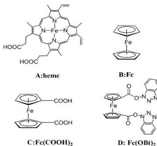
**Figure 1.** Structure diagram of heme, ferrocene and its derivatives
