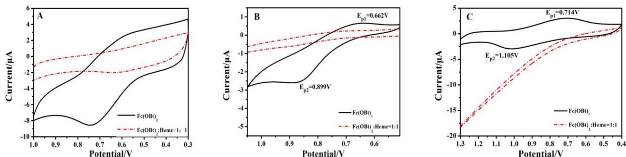
**Figure 4.** CV graphs for  $\text{Fc(OBt)}_2$  before and after the reactions with heme solution in various organic solvents. (A: DMF; B: ethanol; C: dichloromethane)
