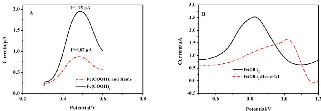
**Figure 5.** DPV graphs for  $\text{Fc(COOH)}_2$  (A) and  $\text{Fc(OBt)}_2$  (B) before and after their reactions with heme. (A: NaOH; B: dichloromethane)
