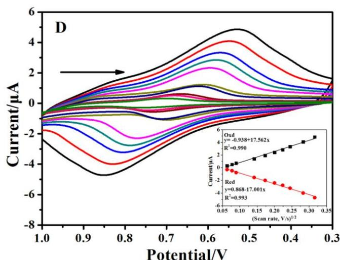
**Figure 2.** CV graph of  $\text{Fc}(\text{COOH})_2$  solution with different scanning rates. Insert: Square root of relationship between current and scanning rate (A: NaOH; B: acetonitrile; C: ethanol; D: dichloromethane).
