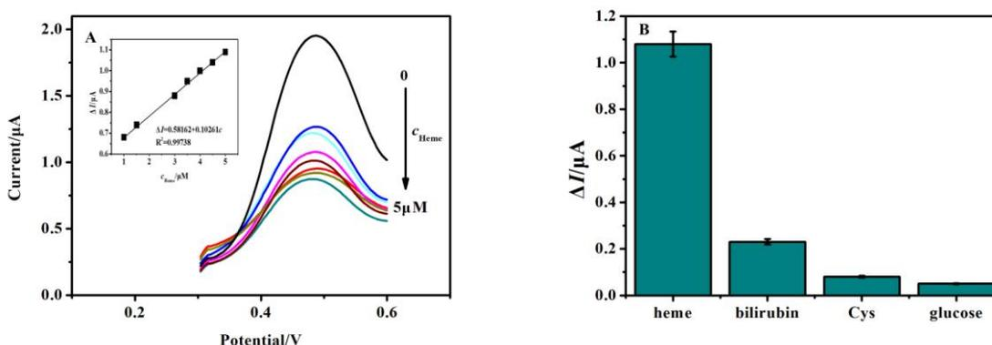
**Figure 6.** **A** Current responses of electrode with various concentrations of heme. Insert: Dependence of  $\Delta I$  on the heme concentration. **B** Selectivity of Fc(COOH)<sub>2</sub> to heme. The concentration of analyte was 5.0  $\mu\text{M}$ .
