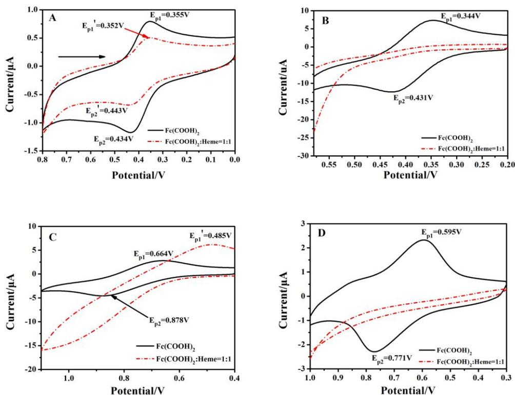
**Figure 3.** CV graphs for  $\text{Fc}(\text{COOH})_2$  before and after reactions with heme in various solvents. (A: NaOH; B: acetonitrile; C: ethanol; D: dichloromethane)
