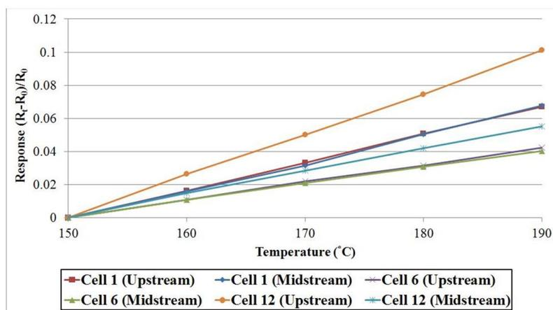
**Figure 3.** Temperature correction curves of micro temperature sensor.
