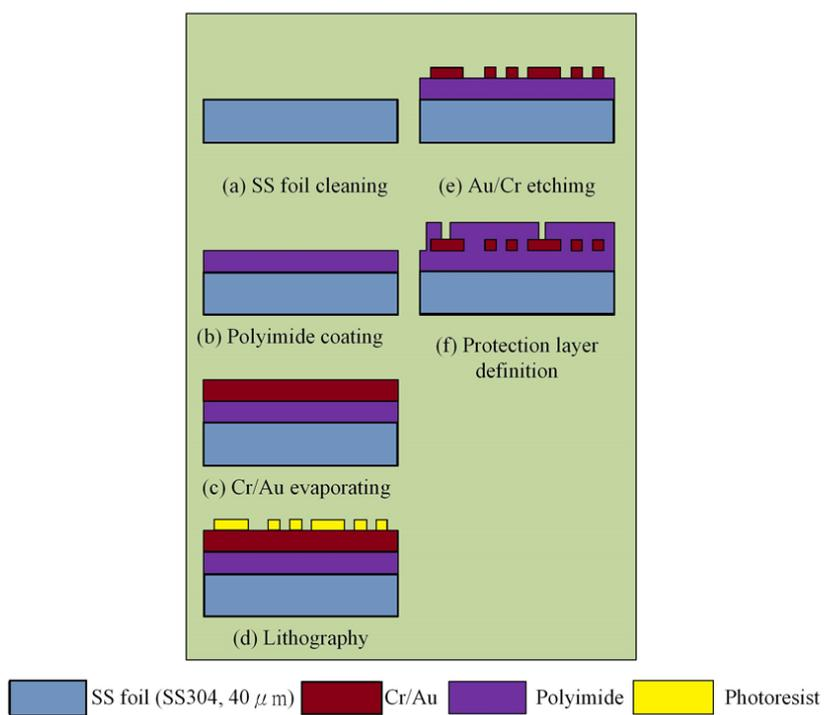
Figure 2. Production process of flexible multiple micro sensor.
