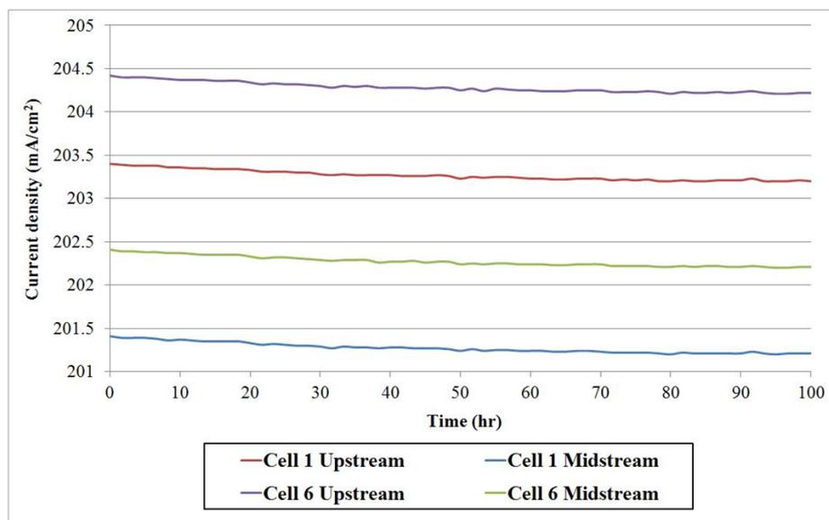
Figure 5. Persistent effect test chart of local current density of high temperature fuel cell stack.
