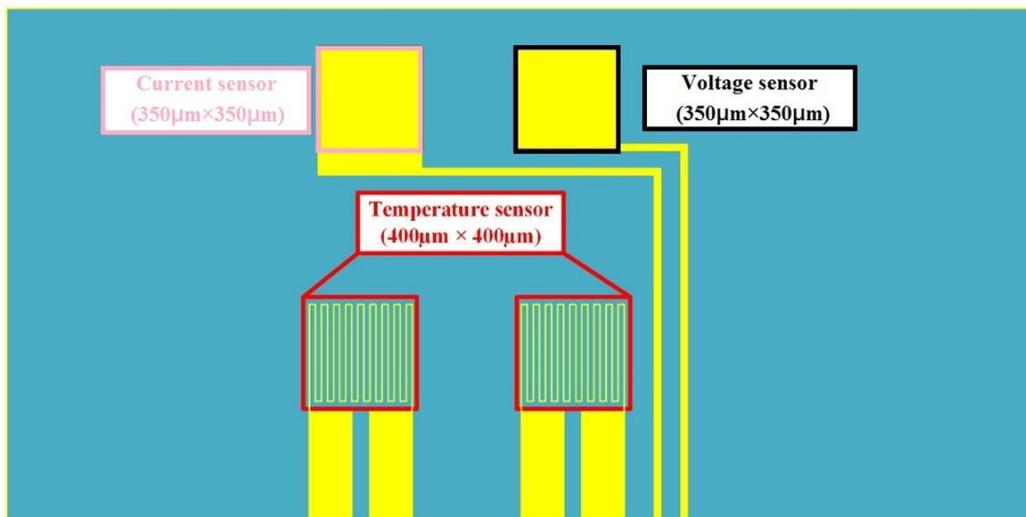
**Figure 1.** Design drawing of flexible multiple micro sensor.
