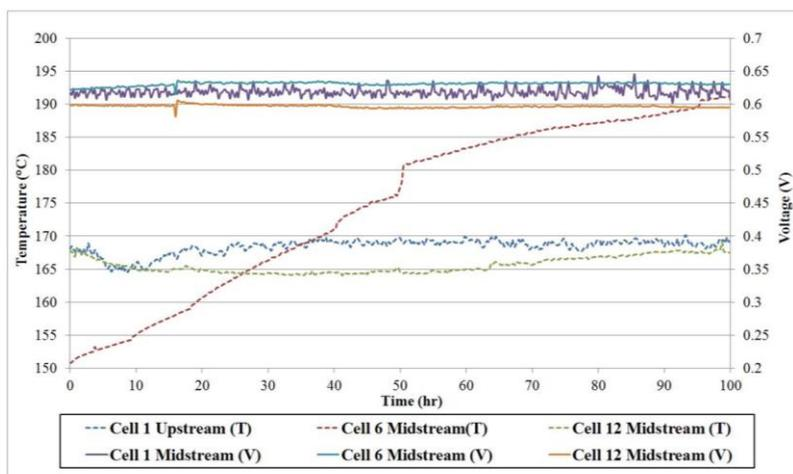
**Figure 4.** Persistent effect test chart of local temperature and voltage of high temperature fuel cell stack.
