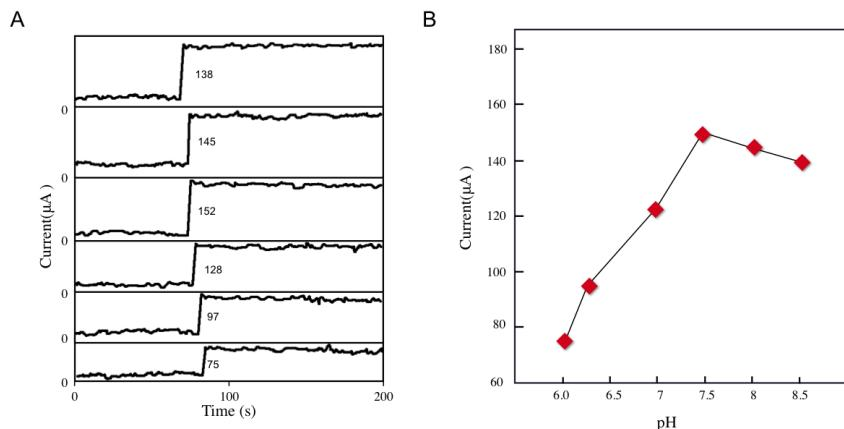
**Figure 3.** Influence of the pH of the solution on the response of the immunosensor incubated with 20 ng/ml MMP-9 in 5 mM  $\text{Fe}(\text{CN})_6^{4-/\text{3}-}$  solution containing 0.1 M KCl. All potentials are given vs. SCE and the scan rate was 50 mV/s. (A) Amperometric response curves. (B) Current response trend.
