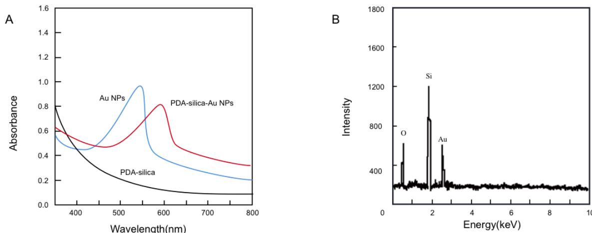
**Figure 1.** (A) UV-vis spectra of colloidal Au NPs, PDA/silica and the as-prepared Au NPs functionalized PDA/silica nanocomposite. (B) EDX spectrum of the as-fabricated Au NPs functionalized PDA/silica nanocomposite.
