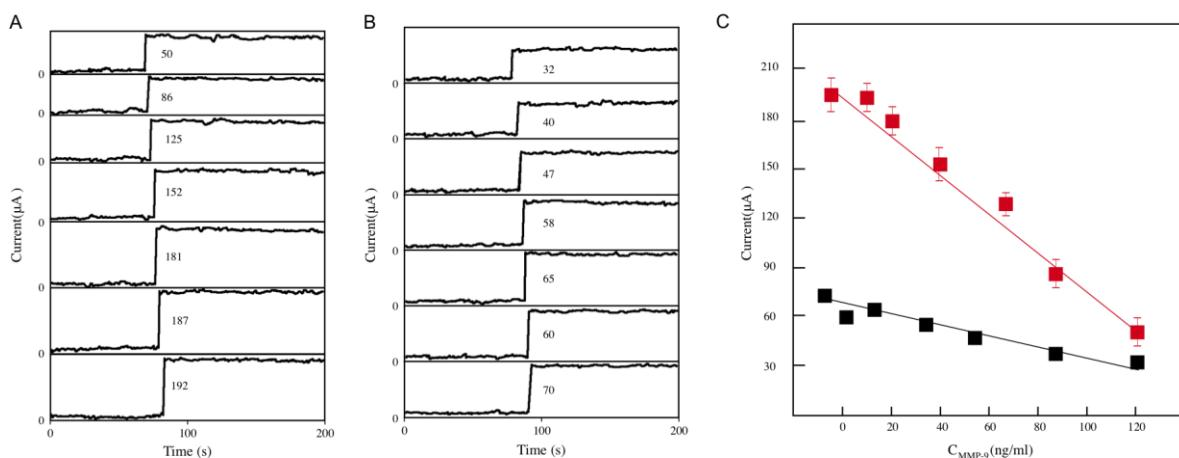
**Figure 4.** (A) Amperometric response curves of anti-MMP-9/GCE and (B) anti-MMP-9/Au NPs-silica/GCE. (C) Calibration plots of the anodic peak current response vs. concentration of anti-MMP-9/GCE and anti-MMP-9/Au NPs-silica/GCE with the different immunosensors under optimal conditions.
