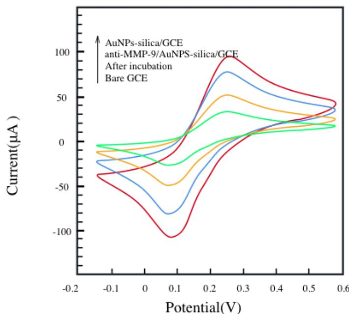
**Figure 2.** CVs of the electrode at diverse phases: bare GCE, Au NPs-silica/GCE, anti-MMP-9/Au NPs-silica/GCE and after incubated in the solution containing MMP-9 for 20 min. Supporting electrolyte: 5 mM  $\text{Fe}(\text{CN})_6^{4-}/^{3-}$  solution containing 0.1 M KCl; scan rate, 50 mV/s.
