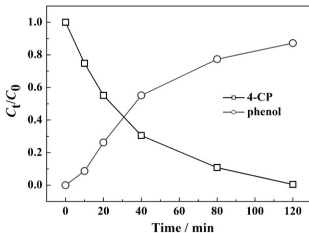
**Figure 8.** Dechlorination process analysis (4-CP 100 mg/L,  $\text{PdCl}_2$  7 mmol/L, pH 2.08,  $\text{Na}_2\text{SO}_4$  0.1 mol/L, current 1.0  $\text{mA}/\text{cm}^2$ ).
