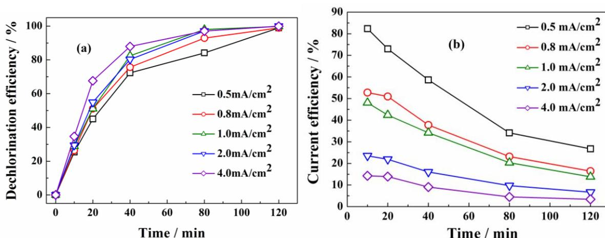
Figure 6. Effects of current density on the dechlorination efficiency (a) and the current efficiency (b) (4-CP 100 mg/L, PdCl<sub>2</sub> 7 mmol/L, pH 2.08, Na<sub>2</sub>SO<sub>4</sub> 0.1 mol/L).
