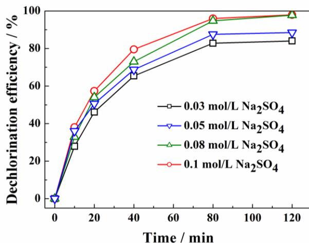
**Figure 7.** Effects of  $\text{Na}_2\text{SO}_4$  concentration on the dechlorination of 4-CP (4-CP 100mg/L,  $\text{PdCl}_2$  7 mmol/L, pH 2.08, current 1.0  $\text{mA}/\text{cm}^2$ ).
