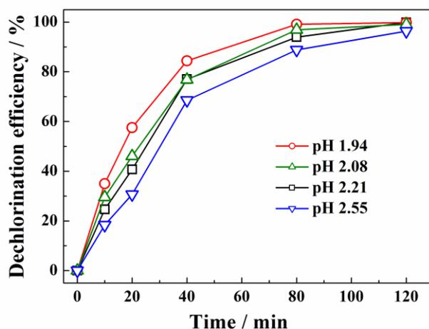
Figure 5. Dechlorination efficiency at different initial pH values using the Pd/PPy-MWCNTs/Ti electrode (4-CP 100 mg/L, PdCl<sub>2</sub> 7 mmol/L, Na<sub>2</sub>SO<sub>4</sub> 0.1 mol/L, current 1.0 mA/cm<sup>2</sup>).
