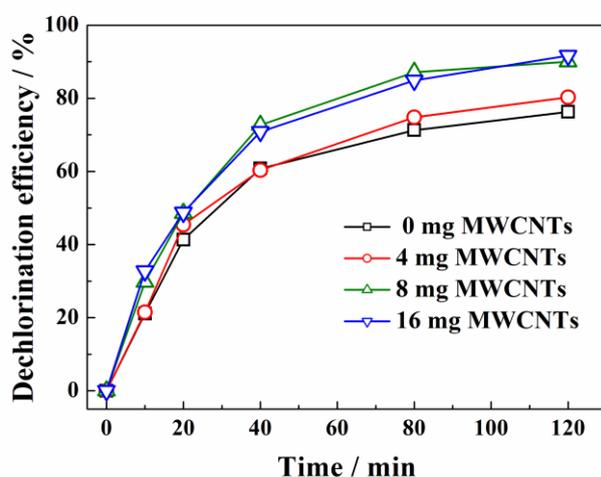
**Figure 3.** Effects of MWCNTs dosage on the dechlorination efficiency using the Pd/PPy-MWCNTs/Ti electrode (4-CP 100 mg/L, PdCl<sub>2</sub> 5 mM, pH 2.2, Na<sub>2</sub>SO<sub>4</sub> 0.1 mol/L, current 1.0 mA/cm<sup>2</sup>).
