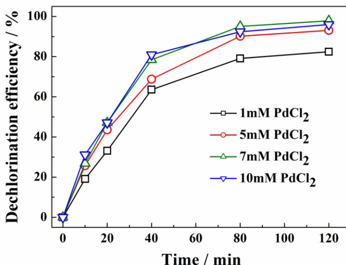
**Figure 4.** Effects of the concentration of PdCl<sub>2</sub> on the dechlorination efficiency (4-CP 100 mg/L, pH 2.2, Na<sub>2</sub>SO<sub>4</sub> 0.1 mol/L, current 1.0 mA/cm<sup>2</sup>).
