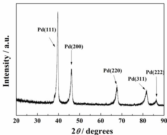
**Figure 1.** XRD pattern of the Pd/PPy-MWCNTs/Ti electrode.
