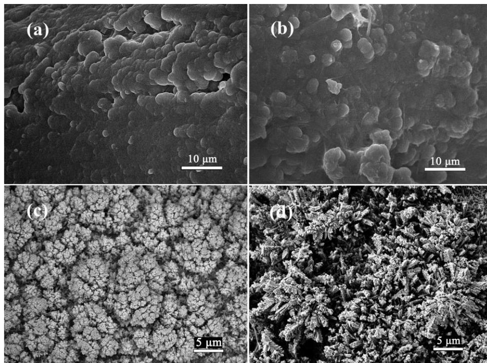
**Figure 2.** SEM images of the PPy/Ti electrode (a), the PPy-MWCNTs/Ti electrode (b), the Pd/PPy-MWCNTs/Ti electrode (c) and the Pd/PPy-MWCNTs/Ti electrode after being used for eight cycles (d).
