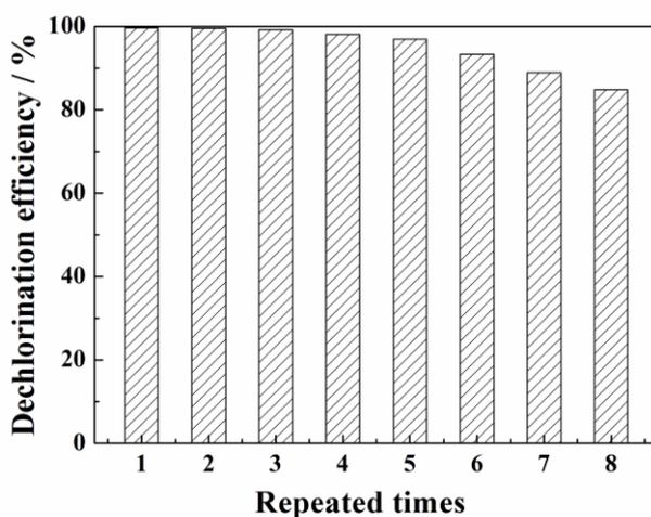
**Figure 9.** The dechlorination of 4-CP in eight reaction cycles using the Pd/PPy-MWCNTs/Ti electrode.
