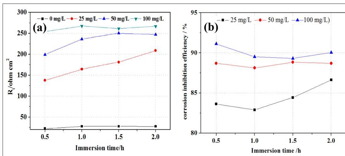
**Figure 5.** The charge transfer resistance  $R_t$  (a) and corrosion inhibition efficiency (b) of inhibitor in 1M HCl solution of after in different immersion time.
