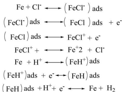
**Scheme 2.** The reaction Ep of carbon steel in hydrochloric acid
