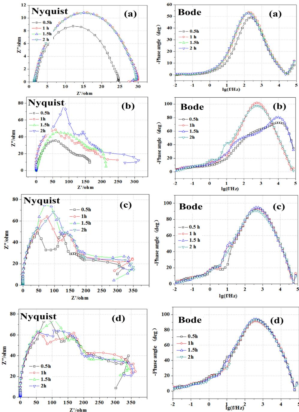
**Figure 3.** The Nyquist and Bode curves for different concentrations of inhibitor in 1M HCl solution: 0 mg/L (a), 25 mg/L (b), 50 mg/L (c), and 100 mg/L (d).
