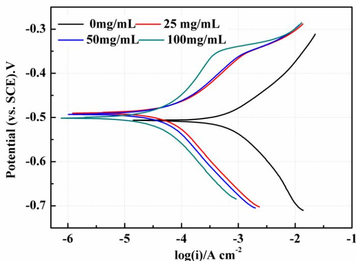
**Figure 6.** Polarization curves of inhibitor in 1M HCl solution: 0 mg/L (a), 25 mg/L (b), 50 mg/L (c), and 100 mg/L (d).
