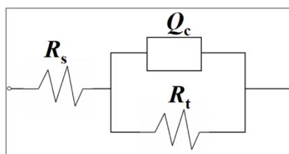
**Figure 4.** Equivalent electrical circuit used to fit the EIS data.
