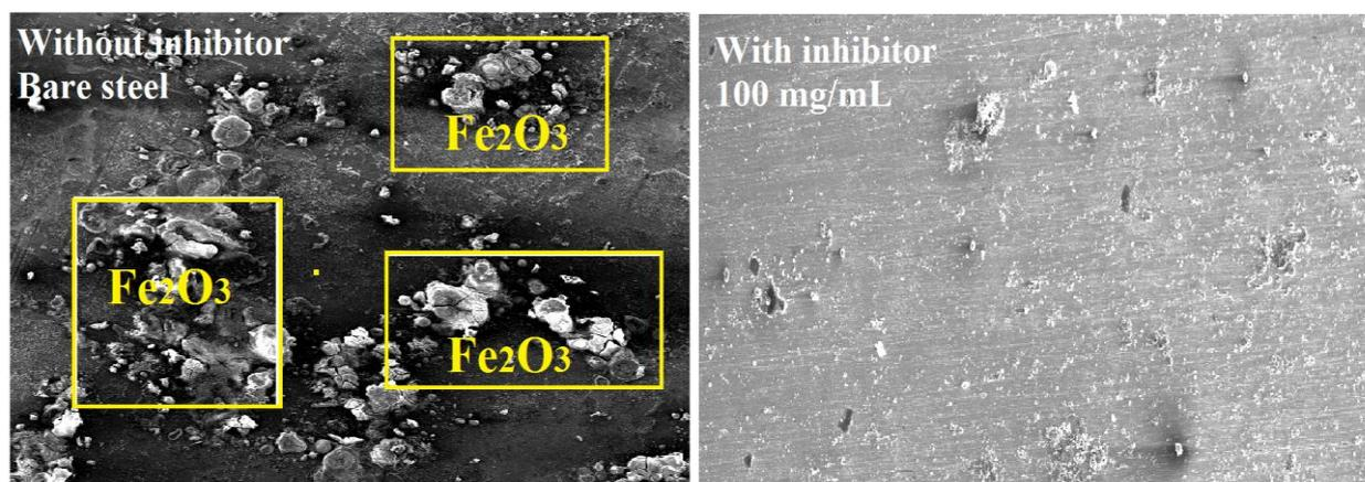
**Figure 7.** The SEM image of Q235 carbon steel surfaces without any inhibitor and with 100mg/ml inhibitor after immersion in HCl solution for 24h.
