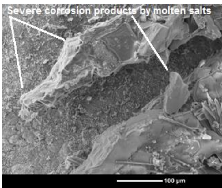
Figure 6. Micrograph of the coating worn by the effect of the corrosive salts after prolonged exposure and at a temperature of 700 ° C.
