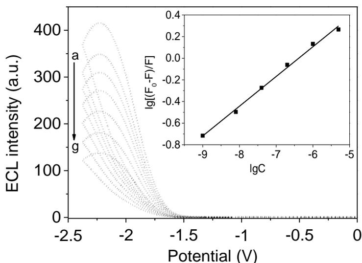
**Figure 10.** Effect of hemoglobin with different concentrations on ECL spectra of CdTe quantum dots, and the inset was the relationship of difference ECL intensity with the concentration of hemoglobin
