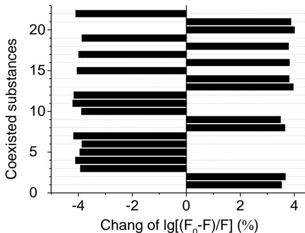
**Figure 9.** Effects of potential coexistence substances on the measurement of  $5.0 \times 10^{-7}$  mol/L hemoglobin were investigated.
