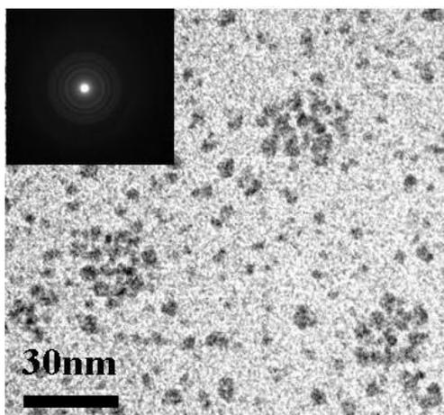
**Figure 3.** TEM image of CdTe quantum dots for heating 220 min
