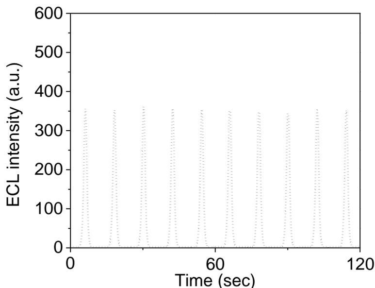
**Figure 8.** The results of repeated ECL of CdTe quantum dots in 0.1 mol/L PBS with 0.02 mol/L tripropylamine, and Nafion-GCE was used as the working electrode.
