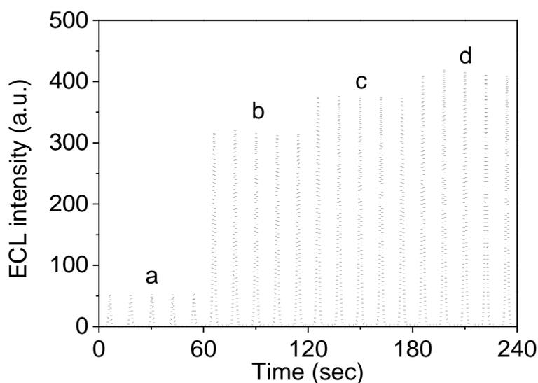
Figure 5. ECL curves of CdTe quantum dots with four sized on Nafion-GCE
