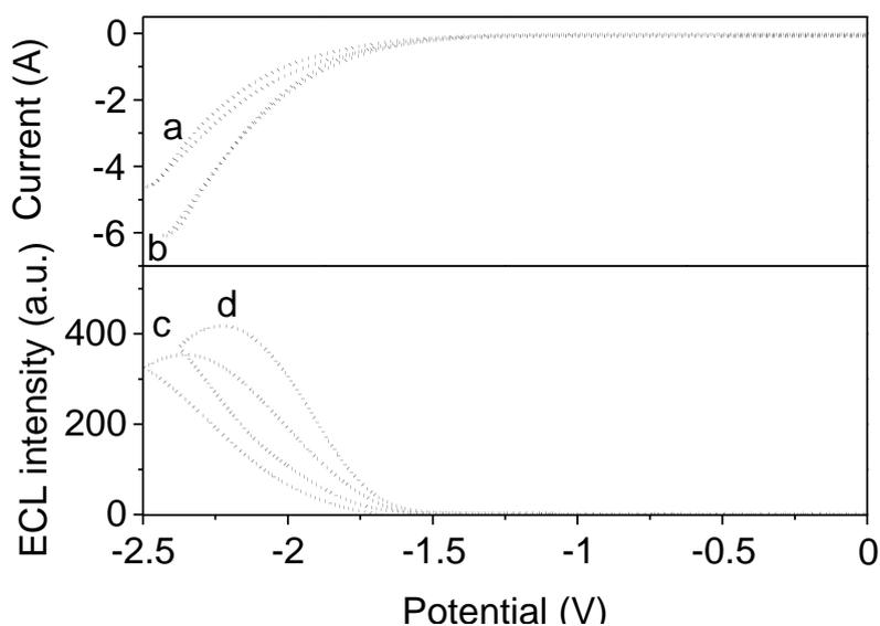
**Figure 7.** The direct cyclic voltammetric and ECL behavior of CdTe quantum dots was investigated in bared GCE and Nafion-GCE. (a, c was performed in bared GCE, and b, d was obtained in Nafion- GCE).
