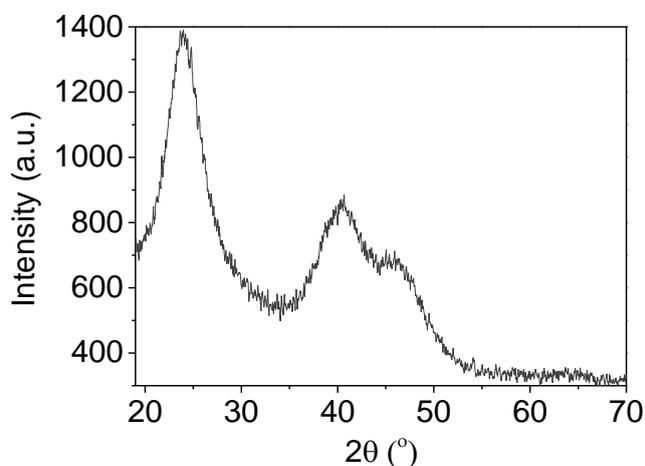
**Figure 4.** The XRD diagram of CdTe quantum dots powder
