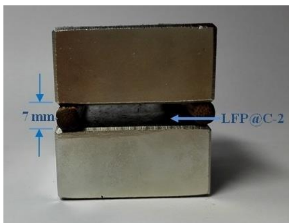
Figure 1. Digital photo of the magnetization of LFP@C-2.
