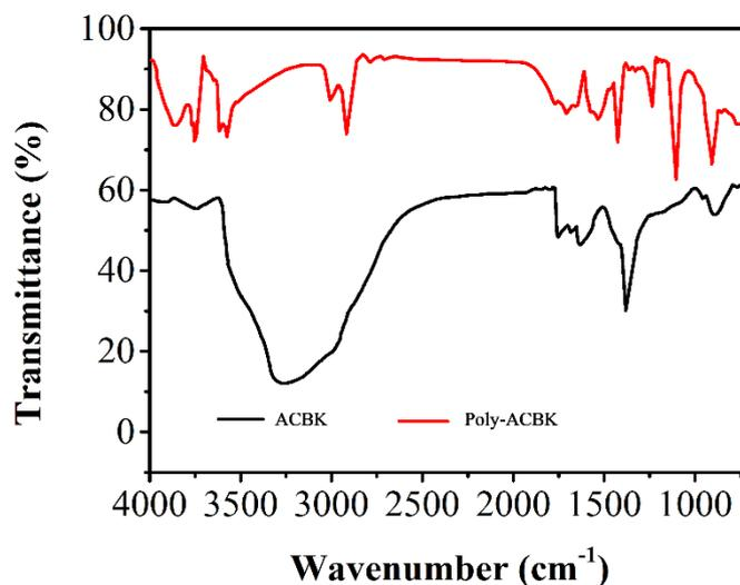
**Figure 2.** FTIR spectra of ACBK and poly-ACBK on GCE surface.
