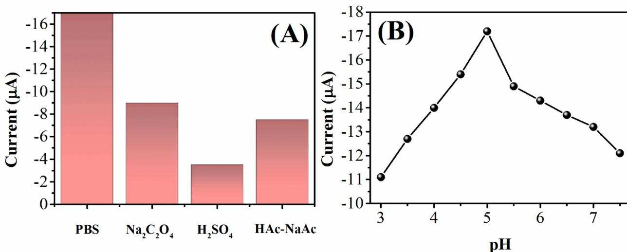
**Figure 5.** Effects of (A) electrolyte types and (B) pH values of PBS on the oxidation performance of proline on poly-ACBK/GCE.
