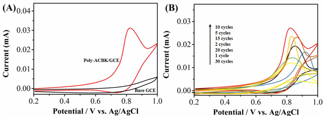
**Figure 4.** Cyclic voltammograms of proline solution (1 mM, pH 7.0) obtained on (A) bare GCE and poly-ACBK/GCE (B) poly-ACBK/GCE prepared with various polymerization cycles (1, 2, 5, 10, 15, 20 and 30) with scan rate of 50mV/s.
