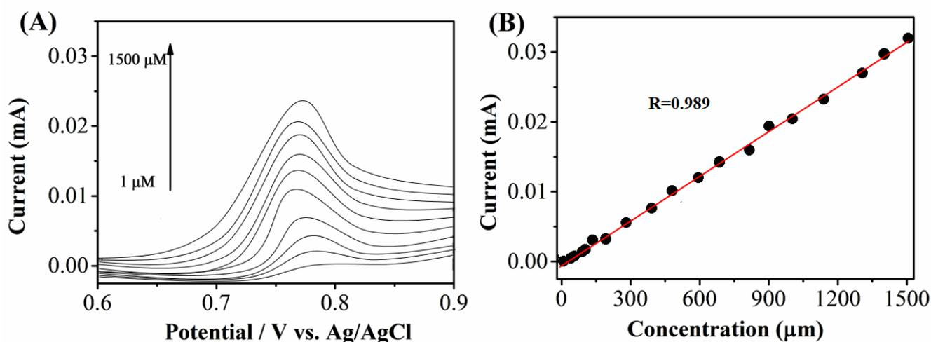
**Figure 6.** (A) DPV curves of proline at various concentrations on the proposed poly-ACBK/GCE electrodes. (B) The plot of  $I_{pa}$  in function of proline concentration.
