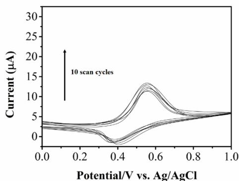
**Figure 1.** Cyclic voltammograms for polymerization of ACBK (0.5 mM) in phosphate buffer solution (0.05 M, pH 7.0) on GCE with the potential range from 0 to 1.0 V at a scan rate of 100 mV/s.
