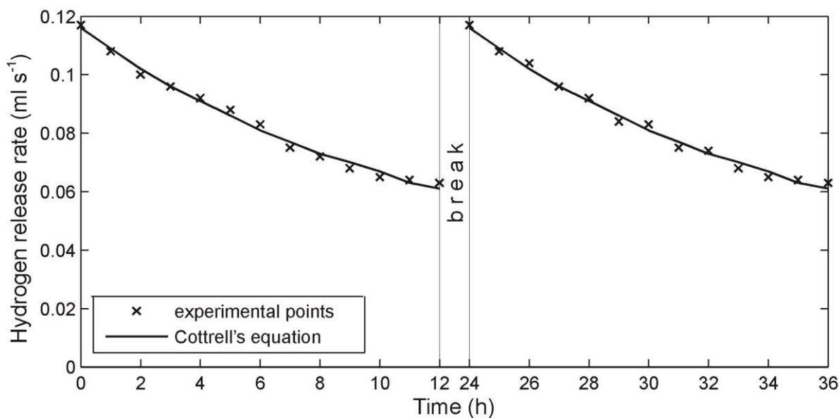
**Figure 1.** Process of hydrogen release relaxation at thermal decomposition of an oxide-nickel electrode of a battery K SX-25 at the temperature 800°C.
