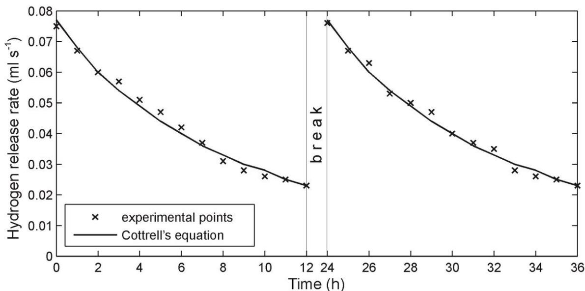
**Figure 2.** Process of hydrogen release relaxation at thermal decomposition of a cadmium electrode of a battery KSX-25 at the temperature 800<sup>0</sup>C.
