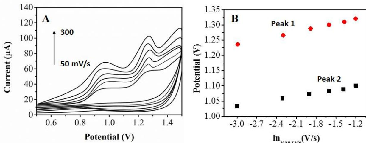
**Figure 4.** The cyclic voltammograms of apigenin under different scan rates (A). Relationship between the anodic peak potential ( $E_p$ ) and the natural logarithm of the scan rate ( $\ln v$ ) for P1 and P2 (B). Condition: 0.1 M B-R buffer solution (50% ethanol, pH=3.0) (25 °C, scan rate 0.05 V/s)
