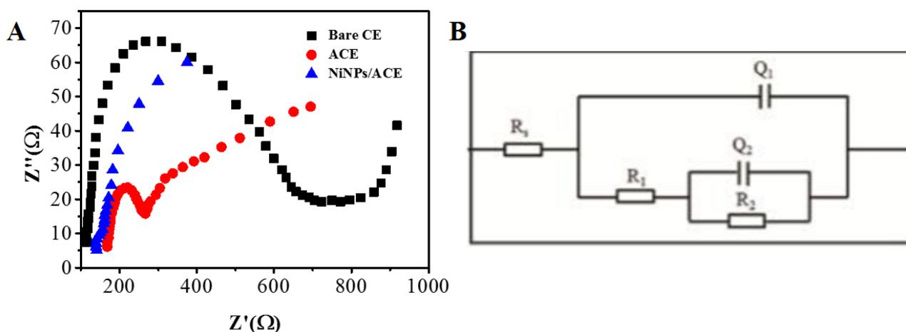
**Figure 2.** (A) EIS of bare CE, ACE and NiNPs/ACE in PBS containing  $\text{K}_3\text{Fe}(\text{CN})_6/\text{K}_4\text{Fe}(\text{CN})_6$  (1:1) with a concentration of 10 mM in the presence of KCl (0.1 M). (B) Randles equivalent circuit model used for EIS analysis.
