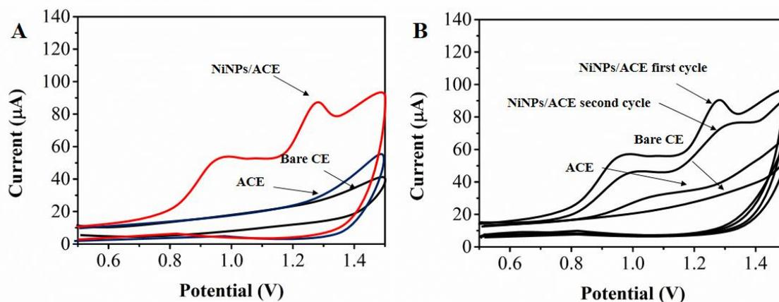
**Figure 3.** (A) The voltammograms of the CE, ACE and NiNPs/ACE under the condition of 10  $\mu$ M apigenin. Condition: 0.1 M B-R buffer solution (50% ethanol, pH=3.0) (25 °C, scan rate 0.05 V/s); (B) The voltammograms with multi-cycles under the condition of 10  $\mu$ M apigenin in 0.1 M B-R buffer solution (Same condition as Figure 3A).
