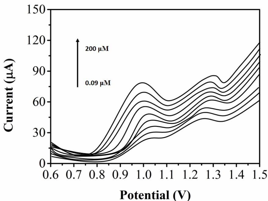
**Figure 5.** Typical differential pulse voltammograms of apigenin with different concentrations under test conditions. Condition: 0.1 M B-R buffer solution (50% ethanol, pH=3.0) (25 °C, scan rate 0.05 V/s)
