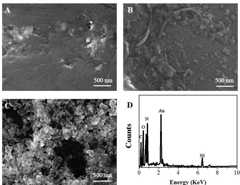
**Figure 1.** SEM images of CE (A), ACE (B) and NiNPs/ACE (C) and EDX result of NiNPs/ACE (D).
