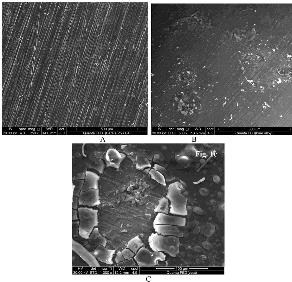
**Figure 1.** SEM images of the bare AA2024-T3 alloy before (a) and after (b) electrochemical exposure to the corroding 3.5% NaCl medium. (C) Titania sol-gel coated alloy after exposure to the corroding medium (and after partially scratching the surface to reveal the underlying surface)
