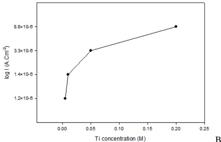
**Figure 5.** (a) Tafel linear polarization measurements showing the effect of TiO<sub>2</sub> concentration in the sol-gel matrix coating over Al2024 in 3.5% NaCl; (b) The dependence of the corrosion current on TiO<sub>2</sub> loading in the sol-gel matrix coating (from data of Figure 5(a)).
