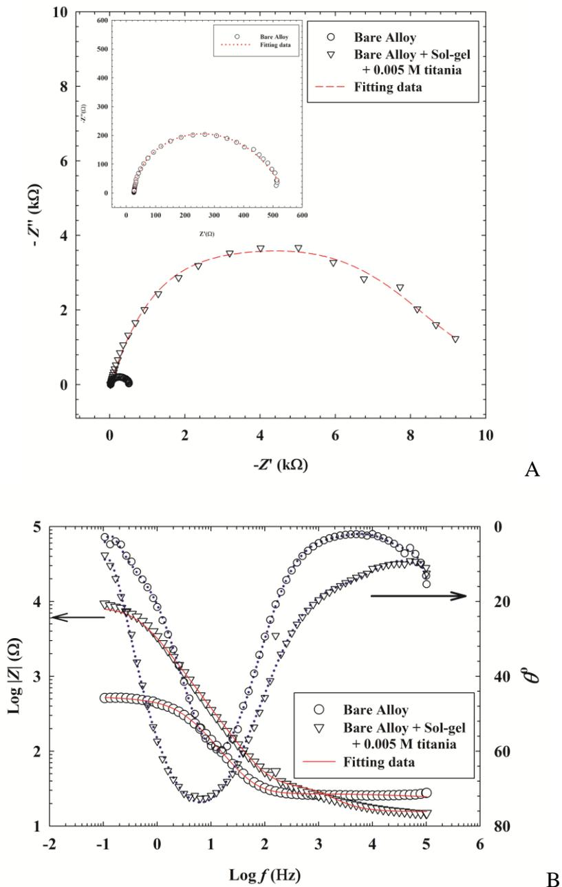
**Figure 4.** Nyquist (4a) and Bode (4b) plots obtained for bare AA2024-T3 alloy and titania (0.005 mol L<sup>-1</sup>) sol-gel coated alloy in 3.5% NaCl solution
