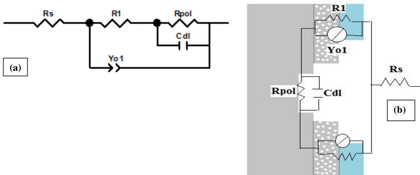
**Figure 3.** (a) Equivalent circuit used for data fitting of the experimental results of EIS measurements, (b) Physical model of the corrosion processes at the alloy coated with sol gel containing titania nanoparticles.
