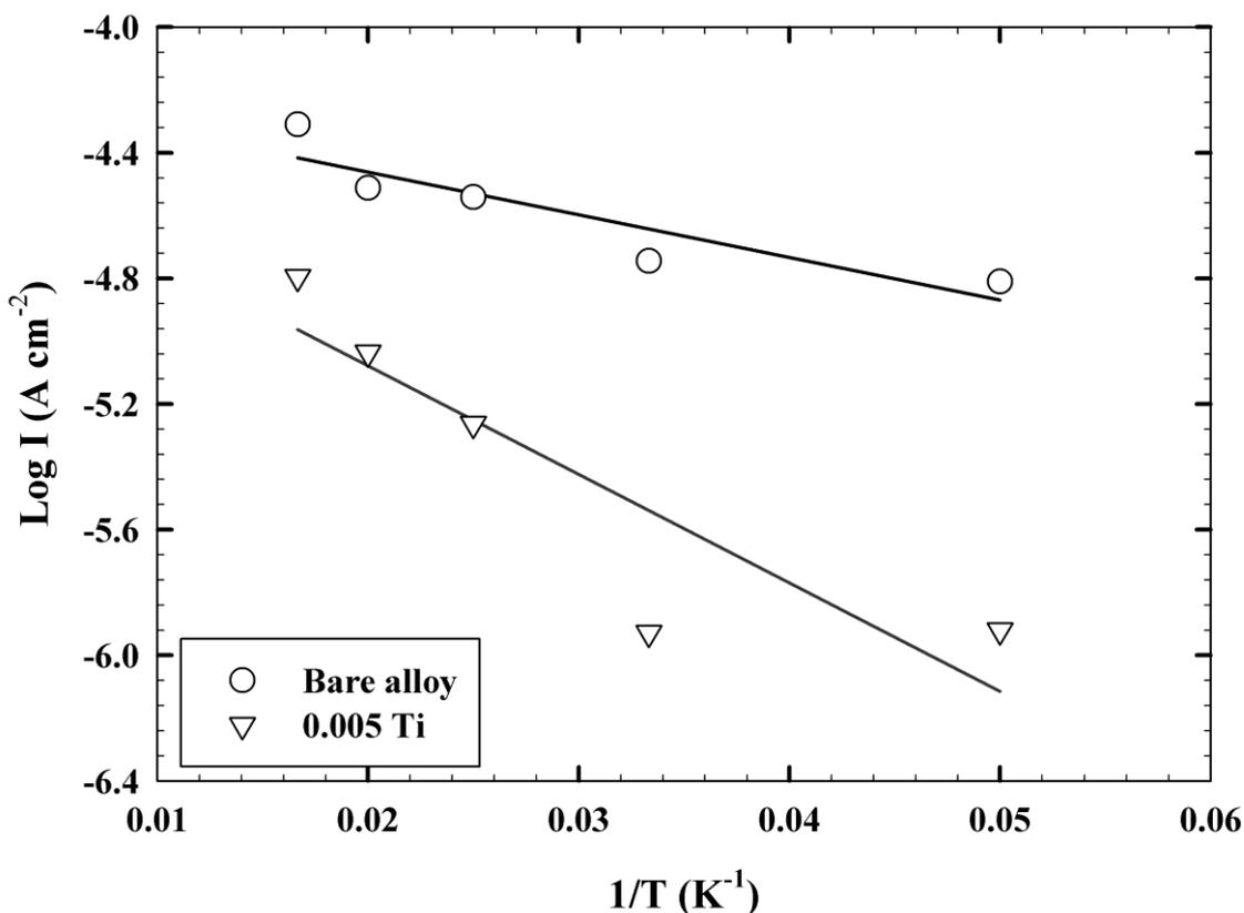
**Figure 7.** Arrhenius plots of corrosion currents of bare and titania-containing sol gel coatings at different temperatures for AA2024-T3 alloy in 3.5% NaCl
