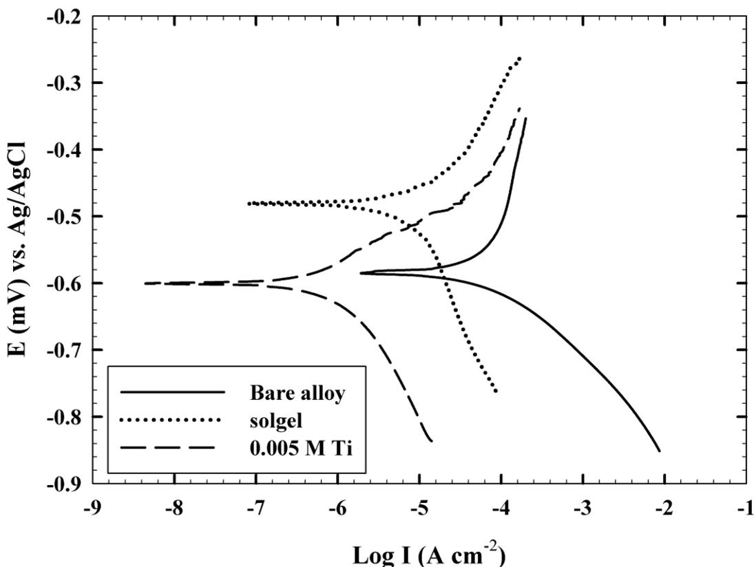
**Figure 2.** Tafel polarization curves of bare AA2024-T3 alloy, sol-gel coated and 0.005 M titania/sol-gel coated alloy in 3.5% NaCl
