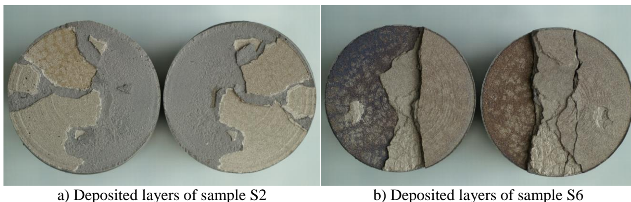
Figure 1. Fracture surface appearance of the samples after the adhesion test
