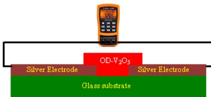
Figure 2. Schematic illustration of sample with surface-type silver electrodes and OD- V_2O_5 film
