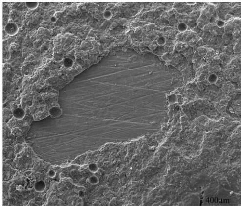
**Figure 5.** SEM photographs of the fractured surface after bond strength test
