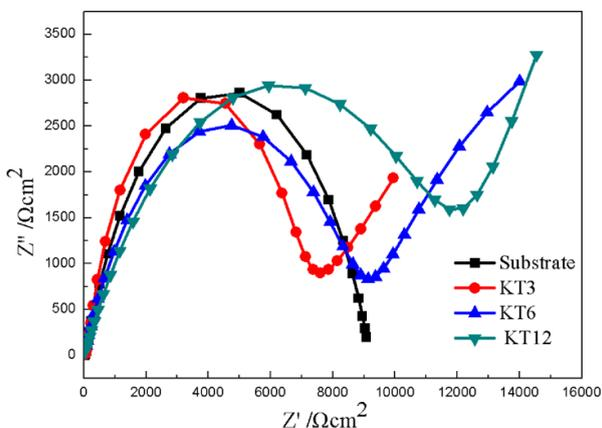
Figure 7. EIS spectra of bare magnesium alloy and the films
