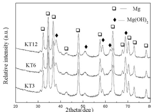
**Figure 3.** XRD patterns of the films under different treatment time
