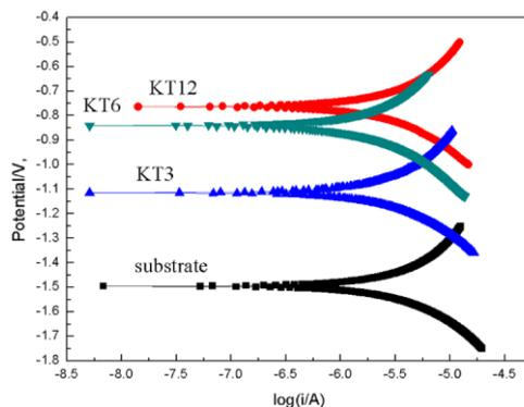
Figure 6. Potentiodynamic polarization tests of the samples in SBF solution
