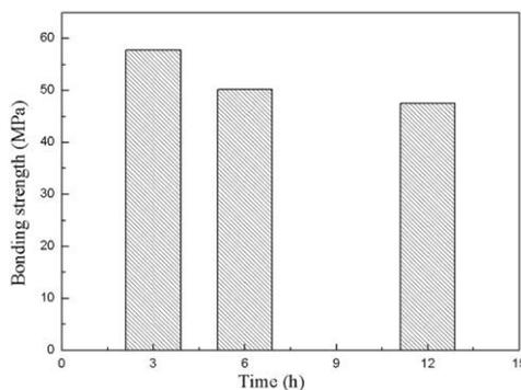
**Figure 4.** Bonding strength of the films prepared under different treatment time
