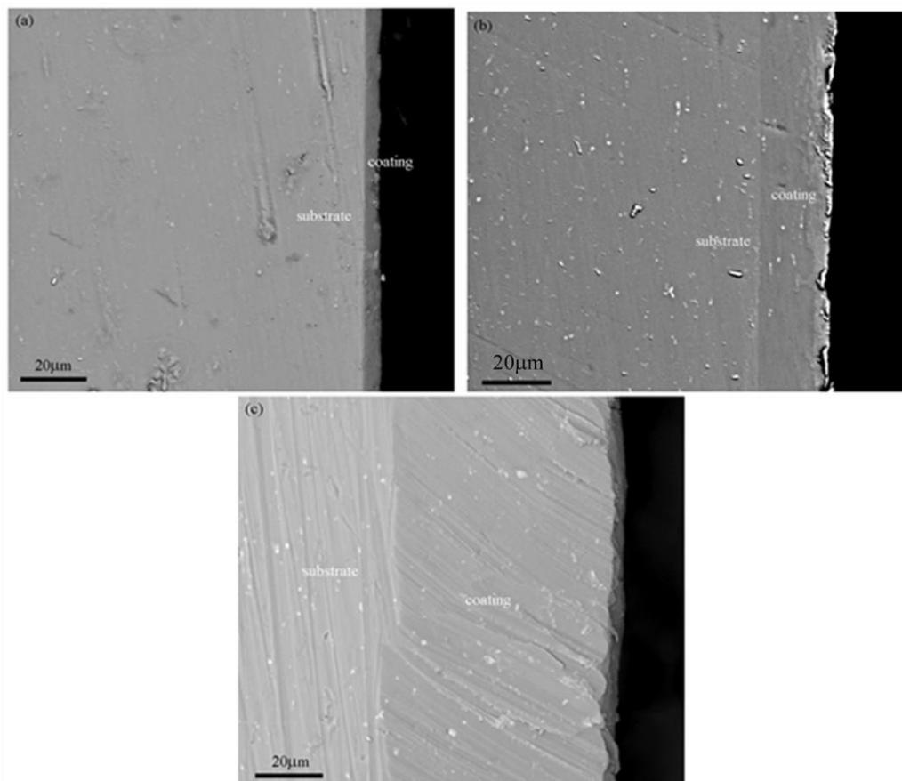
**Figure 2.** Cross-section morphologies of the films formed in different treatment time
