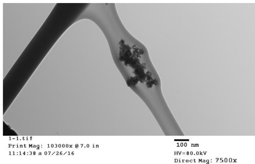
Figure 6. TEM image of ceria NPs embedded in-situ with PVC nanofibers.
