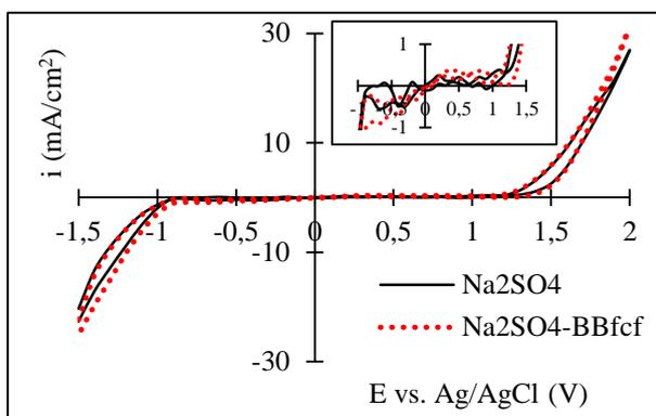
**Figure 2.** Cyclic voltammograms of Pt electrode recorded in: 0.1 mol·L<sup>-1</sup> Na<sub>2</sub>SO<sub>4</sub> (black solid lines) and in 0.1 mol·L<sup>-1</sup> Na<sub>2</sub>SO<sub>4</sub> in the presence of 2·10<sup>-5</sup> mol·L<sup>-1</sup> BBfcf (red dotted lines).
