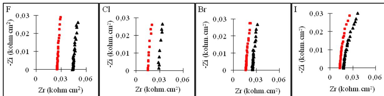
**Figure 5.** The Nyquist diagrams of Pt electrode obtained in: a -  $10^{-1}$  mol·L<sup>-1</sup> NaX (X – F, Cl, Br, I) solution in the absence and in the presence of  $2 \cdot 10^{-5}$  mol·L<sup>-1</sup> BBfcf.
