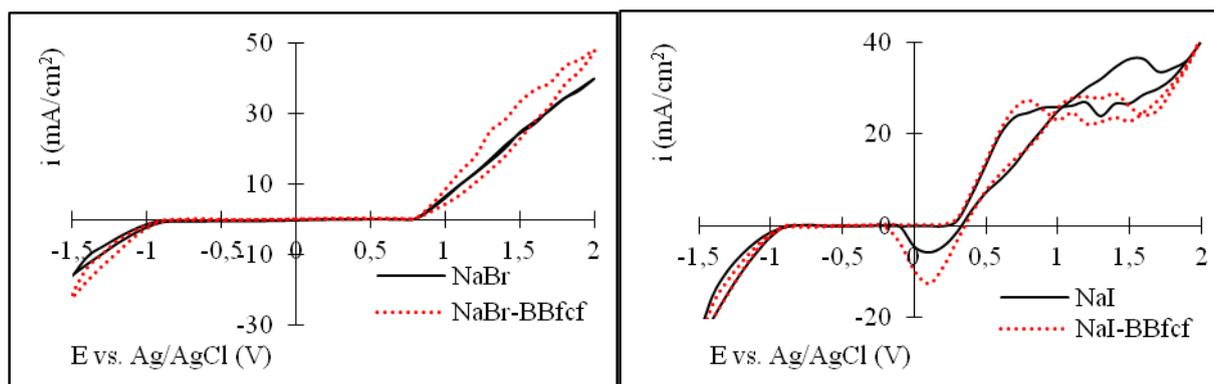
**Figure 3.** Cyclic voltammograms of Pt electrode recorded in:  $0.1 \text{ mol}\cdot\text{L}^{-1}$  NaX (black solid lines) and in  $0.1 \text{ mol}\cdot\text{L}^{-1}$  NaX in the presence of  $2\cdot 10^{-5} \text{ mol}\cdot\text{L}^{-1}$  BBfcf (red dotted lines), (X= F, Cl, Br, I).
