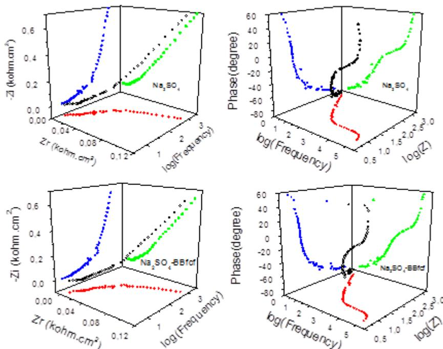
**Figure 4.** 3D Nyquist and 3D Bode diagrams of Pt electrode obtained in  $10^{-1} \text{ mol}\cdot\text{L}^{-1} \text{ Na}_2\text{SO}_4$  solution in the absence and in the presence of  $2\cdot 10^{-5} \text{ mol}\cdot\text{L}^{-1} \text{ BBfcf}$ .
