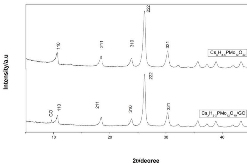
**Figure 2.** XRD spectra of CsPOMo and CsPOMo /GO
