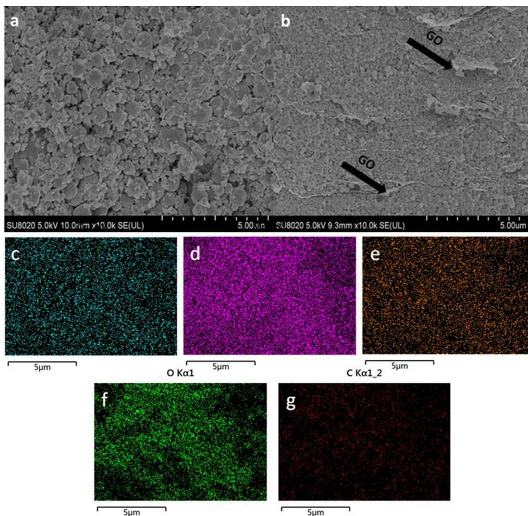
**Figure 1.** SEM images of membrane cross-sections: a) CsPOMo, b) CsPOMo /GO, and c-g) EDX image of Cs, Mo, P, O and C mapping for the cross-section of CsPOMo/GO
