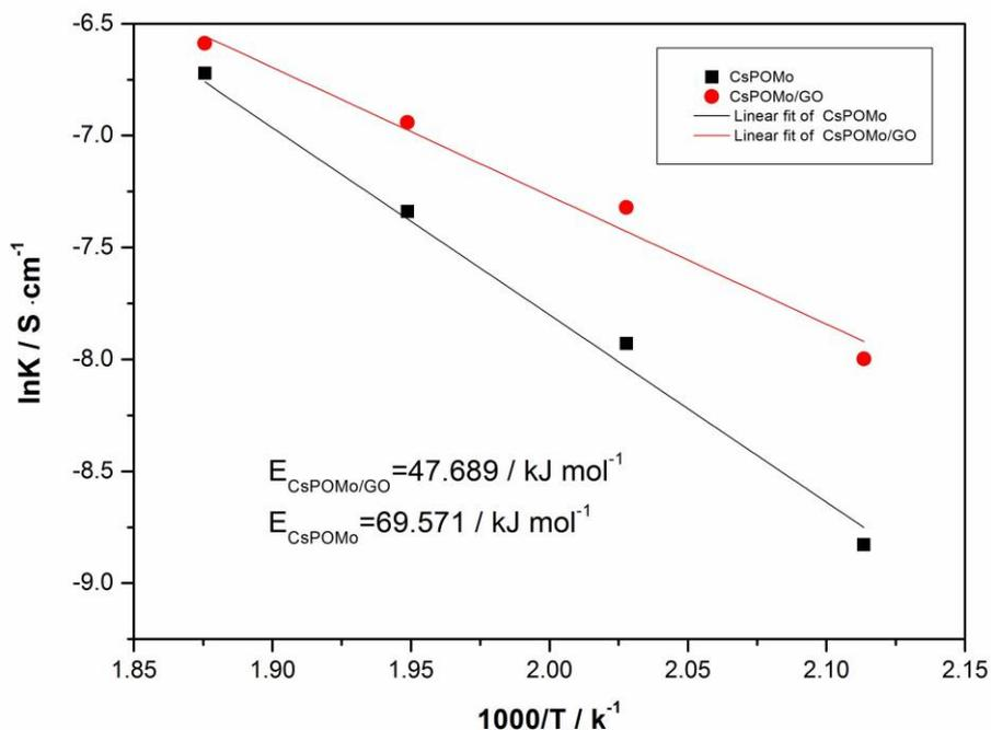
**Figure 5.** Arrhenius plots of CsPOMo and CsPOMo/GO membrane
