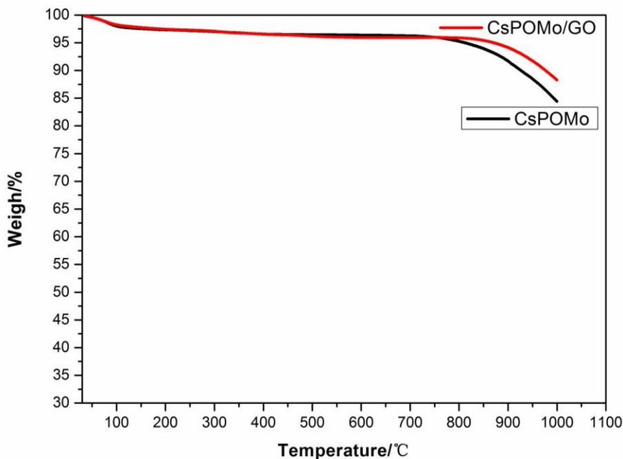
**Figure 3.** TGA of the CsPOMo and CsPOMo /GO from room temperature to 1000 °C
