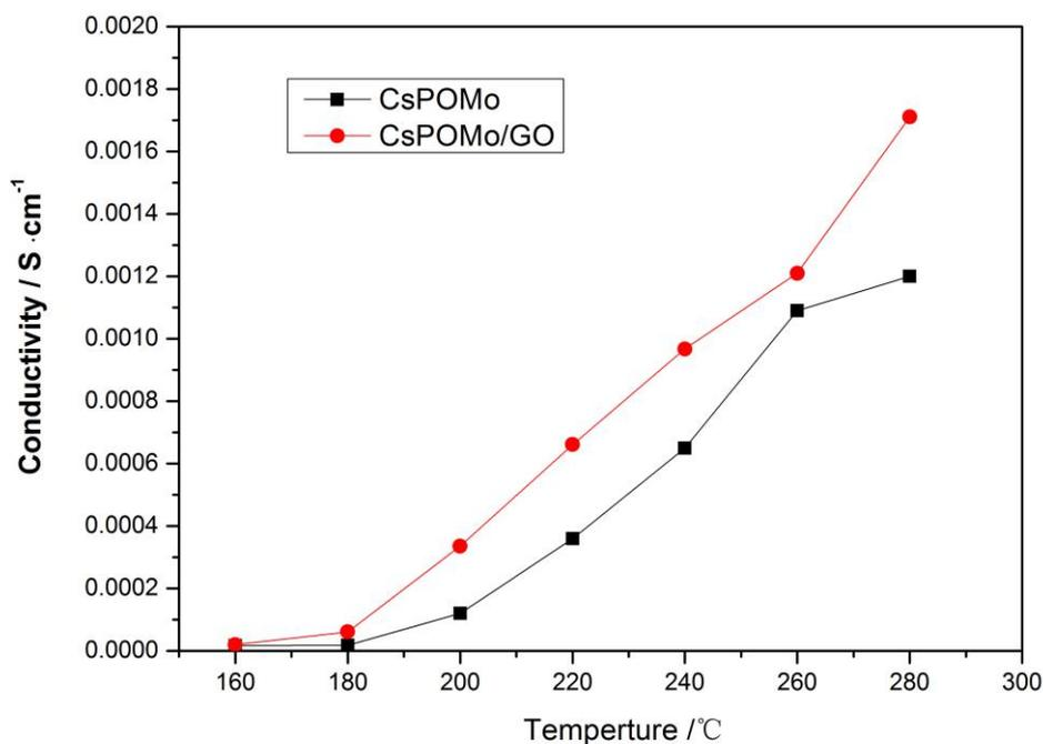
**Figure 4.** The conductivities of CsPOMo and CsPOMo/GO membranes under anhydrous conditions
