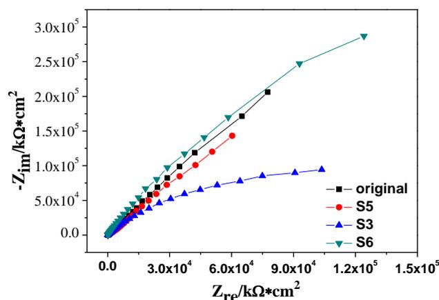
**Figure 5.** Nyquist plots for Electrochemical Impedance Spectrum (EIS) of 316L ASS samples at 240 h immersion before and after laser surface modification.
