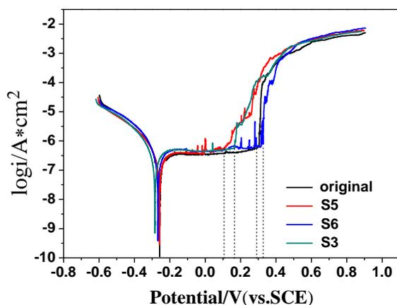
**Figure 4.** Polarization curves for the effects of laser surface treatment on the potentiodynamic behaviour of 316 L orthodontic bracket samples in artificial saliva. The corrosion potential ( $E_{corr}$ ) and breakdown potential ( $E_b$ ) were calculated from the polarization curves via Tafel extrapolation method.
