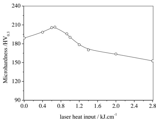
**Figure 3.** Variation of microhardness (HV) as a function of laser heat input on the cross-sectional plane of samples subjected to laser surface heat treatment with power 300-700 W.
