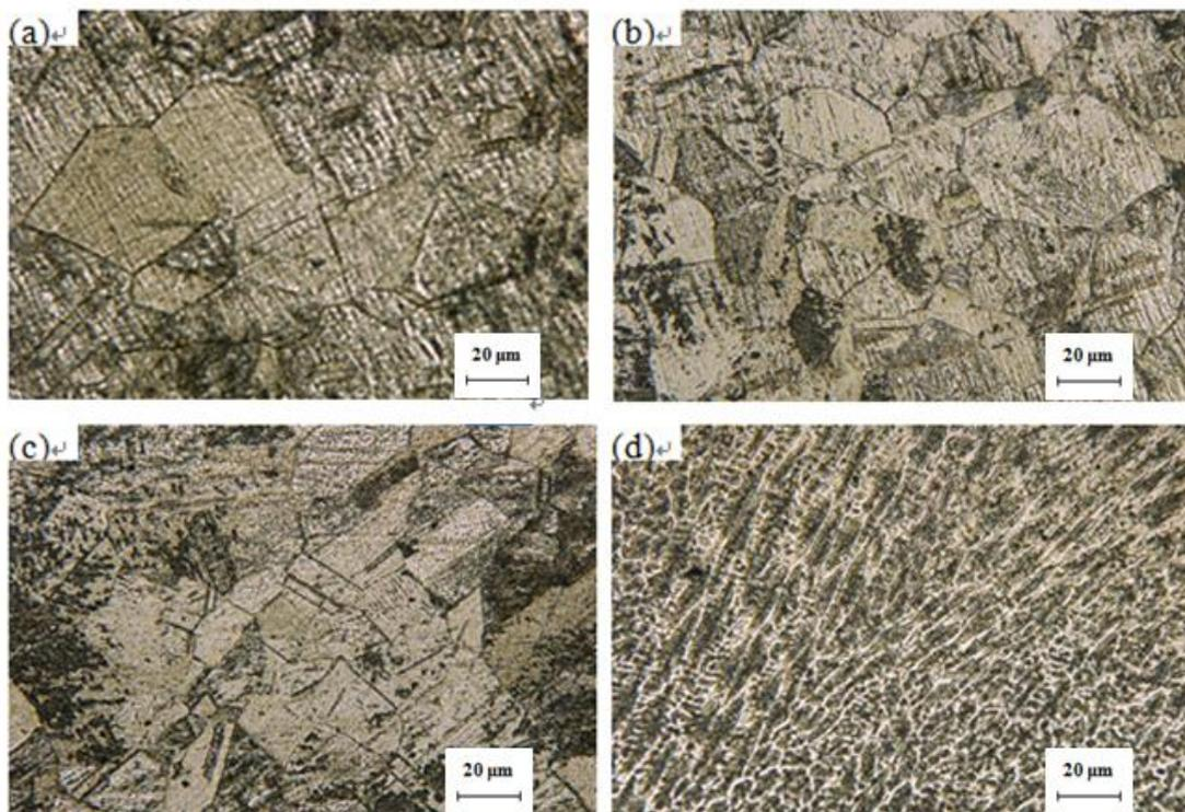
**Figure 1.** Microstructure of the austenitic stainless steel 316 L orthodontic bracket before and after laser heated: (a) Original; (b) S3; (c) S6; (d) S5.
