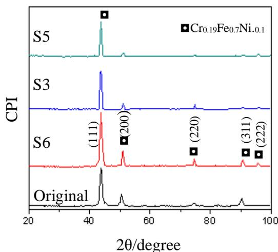
**Figure 2.** X-ray diffraction patterns obtained using Cu-K $\alpha$  radiation (wavelength, 1.54 Å) from the 316 L ASS orthodontic bracket: (Original) without laser heat treatment; (S3, S6, S5) with laser heat (power  $P = 300-700$  W and scanning speed  $v = 2-6$  mm/s).
