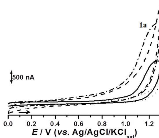
**Figure 2.** Cyclic voltammograms obtained for 0.1% BGT (—), 2  $\mu\text{M}$  Bp (- . -) and 1  $\mu\text{M}$  Ps (- - -) at CP in pH 7.0 0.1 M PBS.
