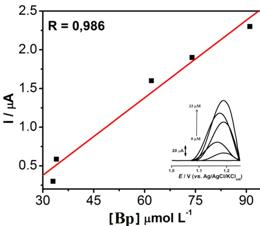
**Figure 5.** Calibration graph and DP voltammograms for incremental Bp concentrations (0.3 to 33 μM).
