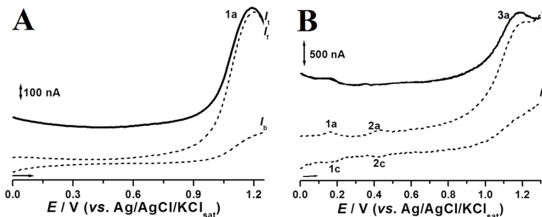
**Figure 4.** SW voltammograms obtained for 1  $\mu$ M Bp (A) and 0.05% BGT (B) at GC in pH 7.0 0.1 M PBS.
