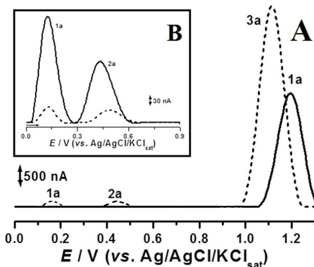
**Figure 3.** A) Baseline corrected DP voltammograms obtained for 1  $\mu$ M Bp (—) and 0.05% BGT (---). B) Successive Baseline corrected DP voltammograms for BGT, 1<sup>st</sup> scan (—) and 2<sup>nd</sup> scan (- - -) all at CP in pH 7.0 0.1 M PBS.
