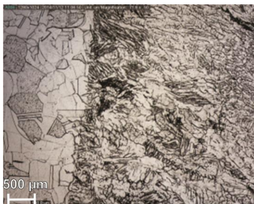
Figure 5. Interphase between the HAZ and weld metal al at 100X obtained by optical microscopy.
