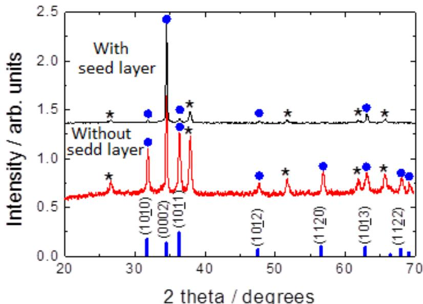
**Figure 2.** X-ray diffraction patterns of ZnO nanorod array samples that were electrochemically grown on a bare FTO/glass substrate and a ZnO thin film seed layer/FTO/glass substrate. The diffraction planes are indicated for ZnO. The hexagonal wurtzite ZnO JCPDS pattern is also shown for comparison (ZnO JCPDS: thick black bars). (\* indicates the peaks originating from the SnO<sub>2</sub>:F substrate).
