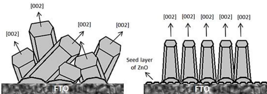
**Scheme 1.** Representation of the growth of ZnO nanorods onto a naked FTO/glass substrate and a ZnO thin film seed layer/FTO/glass substrate.
