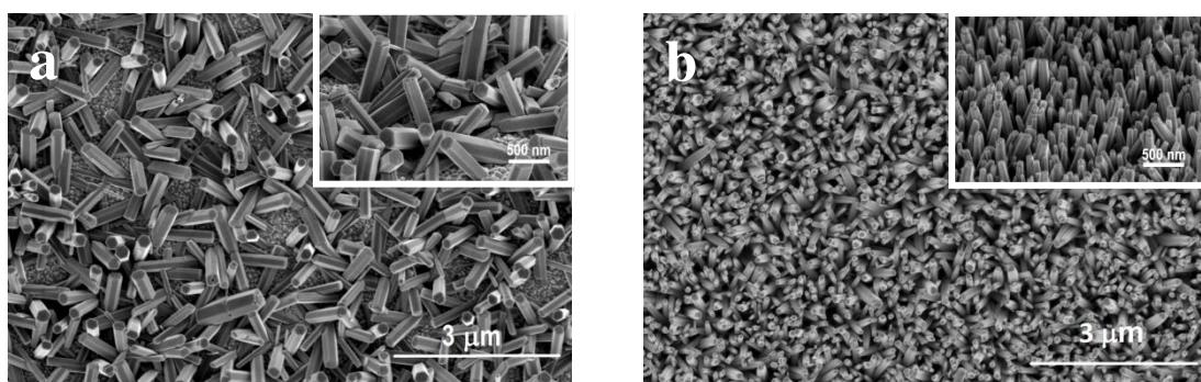
**Figure 1.** (a) Plan-view FE-SEM micrograph images of ZnO nanorod arrays electrochemically grown on a bare FTO/glass substrate. Inset: high-magnification SEM micrograph view of the same sample and with a tilt angle of 45°. (b) SEM plan-view micrograph image of ZnO nanorod arrays electrochemically grown on a ZnO seed layer/FTO/glass electrode substrate. Inset: high-magnification SEM micrograph view of the same sample and with a tilt angle of 45°.
