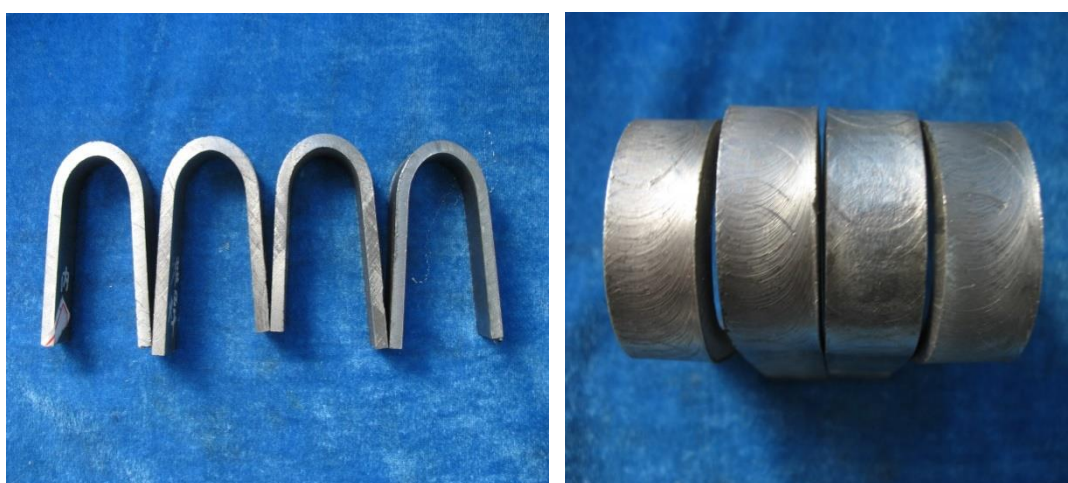
Figure 5. Optical images of the detected samples after bending tests
