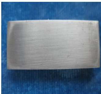
Figure 1. Optical image of the sample surface after corrosion test
