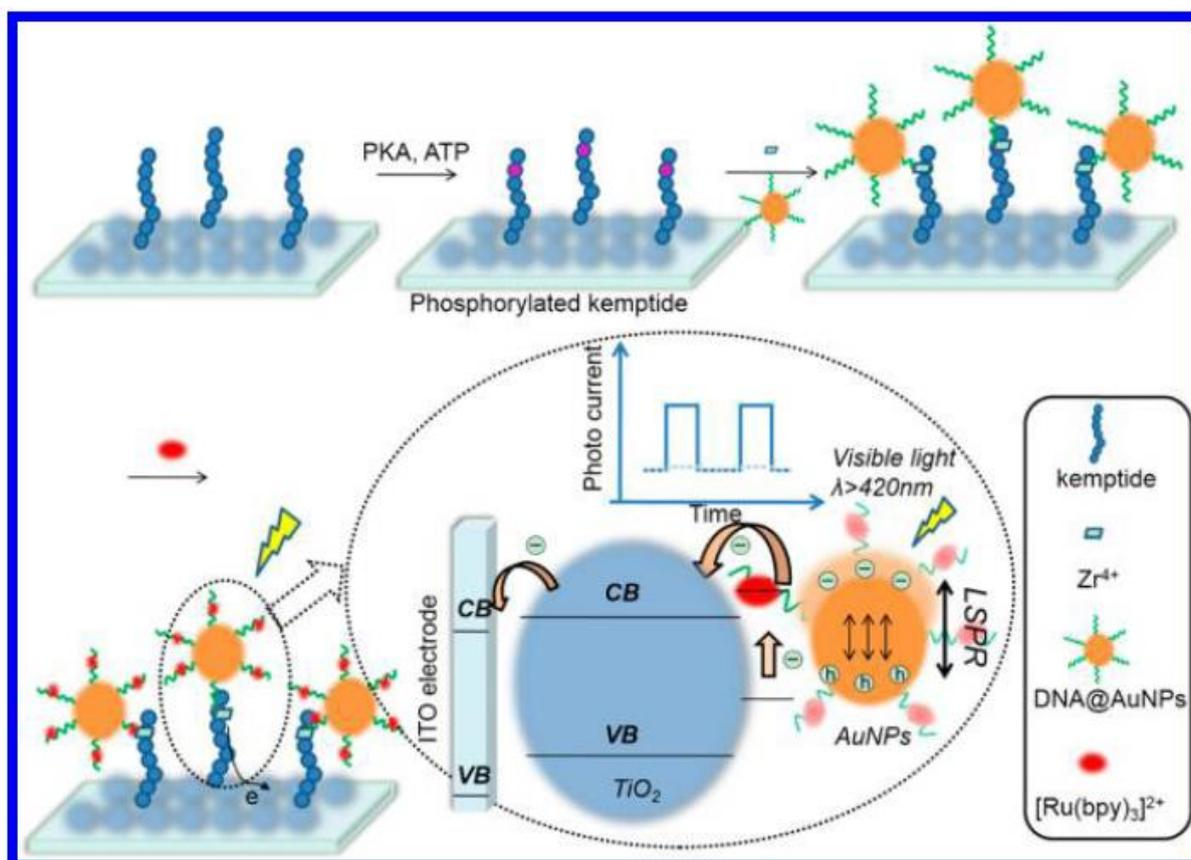
**Figure 6.** Configuration of photoelectrochemical biosensor for kinase activity detection. Reprinted with permission from [40]. Copyright 2016 American Chemical Society.
