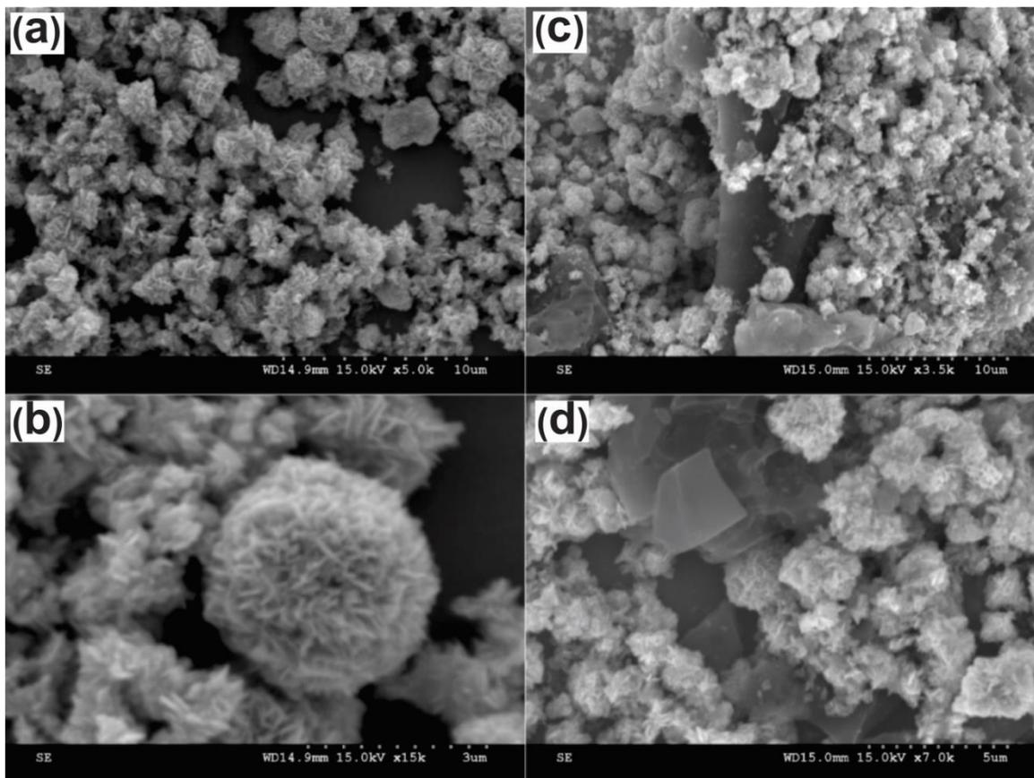
**Figure 1.** SEM images of ZnO (a, b) and AC-ZnO (c,d) at different magnification.
