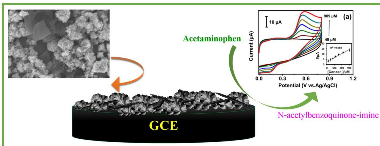
**Scheme 1.** Schematic illustration for electrochemical detection of ACP at AC-ZnO.
