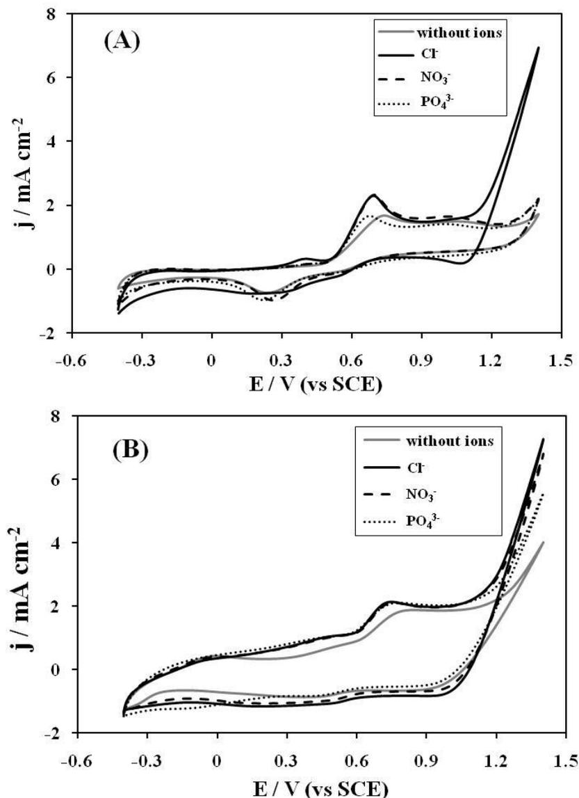
**Figure 8.** Cyclic voltammetry curves recorded on (A) Pt and (B) RuO<sub>2</sub> electrodes in 2 g/L of paracetamol containing 0.1 M KClO<sub>4</sub> electrolyte in the absence and in the presence of 0.1 M Cl<sup>-</sup>, 0.1 M NO<sub>3</sub><sup>-</sup> or 0.1 M PO<sub>4</sub><sup>3-</sup>, CE: Pt, RE: SCE, potential scan rate: 20 mV/s, T = 25°C
