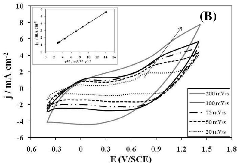
**Figure 5.** Cyclic voltammety curves recorded on (A) Pt and (B) RuO<sub>2</sub> electrodes in 2 g/L paracetamol containing 0.1 M KClO<sub>4</sub> electrolyte at several potential scan rates (20-200 mV/s), CE: Pt, T= 25 °C, RE: SCE. In the inset: Evolution of the peak of current density against the square root of the potential scan rates.
