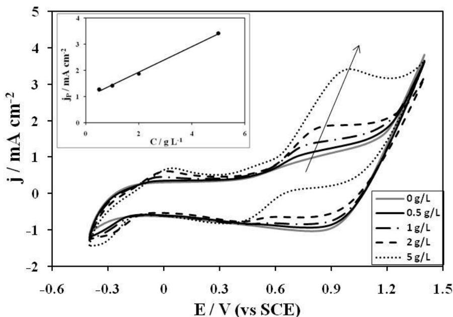
**Figure 4.** Cyclic voltammetry curves recorded on RuO<sub>2</sub> electrode in several concentration of paracetamol containing 0.1 M KClO<sub>4</sub> electrolyte at the potential scan rate: 20 mV/s, CE: Pt, T= 25 °C, RE: SCE. Inset: Plot of current density of the paracetamol oxidation peak versus paracetamol concentrations.
