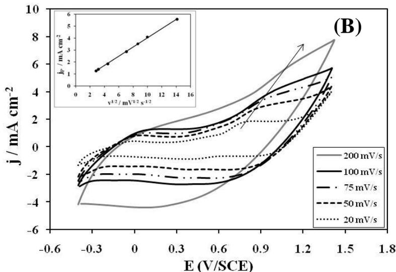
**Figure 5.** Cyclic voltammograms recorded on (A) Pt and (B) RuO<sub>2</sub> electrodes in 2 g/L paracetamol containing 0.1 M KClO<sub>4</sub> electrolyte at several potential scan rates (20-200 mV/s), CE: Pt, T= 25 °C, RE: SCE. In the inset: Evolution of the peak of current density against the square root of the potential scan rates.
