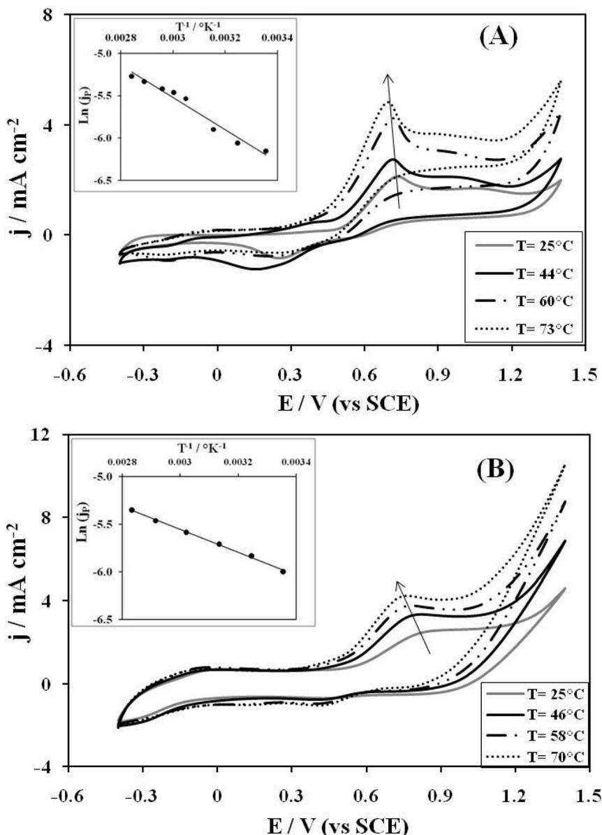
**Figure 7.** Cyclic voltammetry curves recorded on Pt and RuO<sub>2</sub> electrodes in 2 g/L of paracetamol containing 0.1 M KClO<sub>4</sub> electrolyte at several temperatures, CE: Pt, potential scan rate: 20 mV/s, RE: SCE. In the inset: Evolution of the current density peak against reciprocal of electrolyte temperature for the prepared electrodes.
