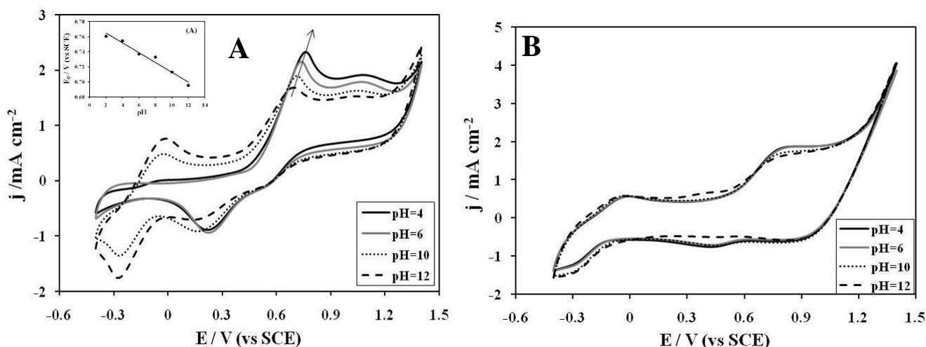
**Figure 9.** Cyclic voltammetry curves recorded on Pt electrode (A) and on RuO<sub>2</sub> electrode (B) in 2 g/L paracetamol containing 0.1 M KClO<sub>4</sub> electrolyte at various pH, potential scan rate: 20 mV/s, CE: Pt, RE: SCE, T = 25°C. In the inset (A) of figure 9 A: The first oxidation potential peak in KClO<sub>4</sub> 0.1 M containing 2 g/L paracetamol against the electrolyte pH (A) against the electrolyte pH.
