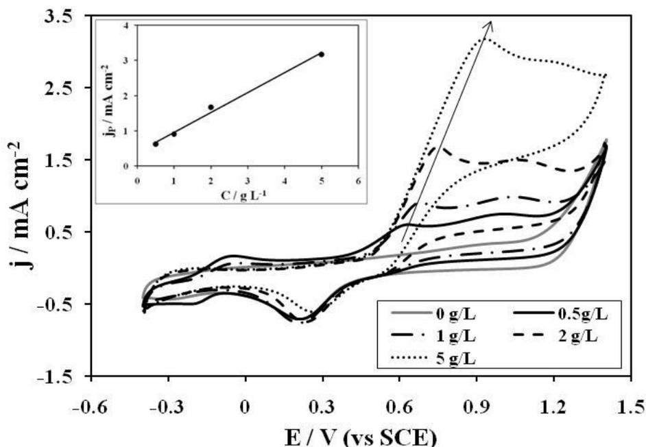
**Figure 3.** Cyclic voltammetry curves recorded on Pt electrode in several concentrations of paracetamol containing 0.1 M KClO<sub>4</sub> electrolyte under the potential scan rate: 20 mV/s, CE: Pt, RE: SCE, T= 25 °C. Inset: plot of current density of the first paracetamol oxidation peak versus paracetamol concentrations
