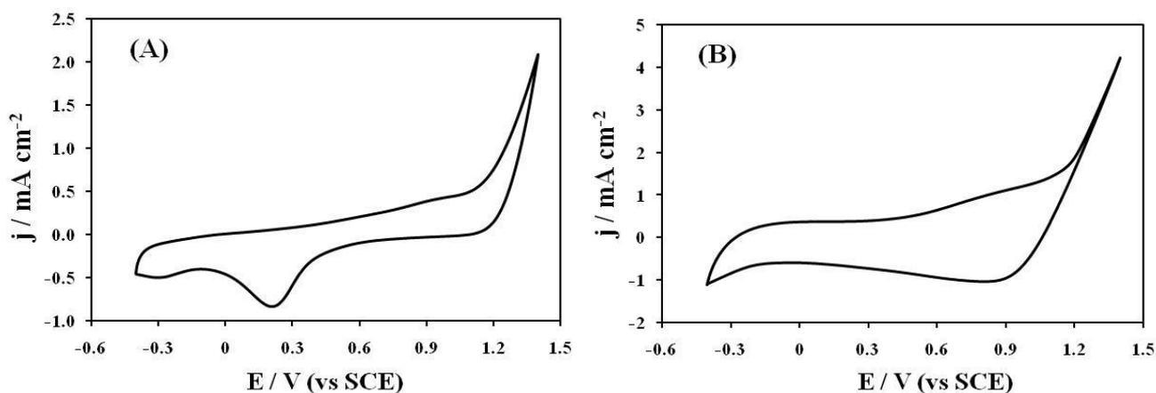
**Figure 2.** Cyclic voltammograms of (A) Pt and (B)  $\text{RuO}_2$  in 0.1 M  $\text{KClO}_4$  at the potential scan rate: 20 mV/s, CE: Pt, RE: SCE,  $T = 25^\circ\text{C}$
