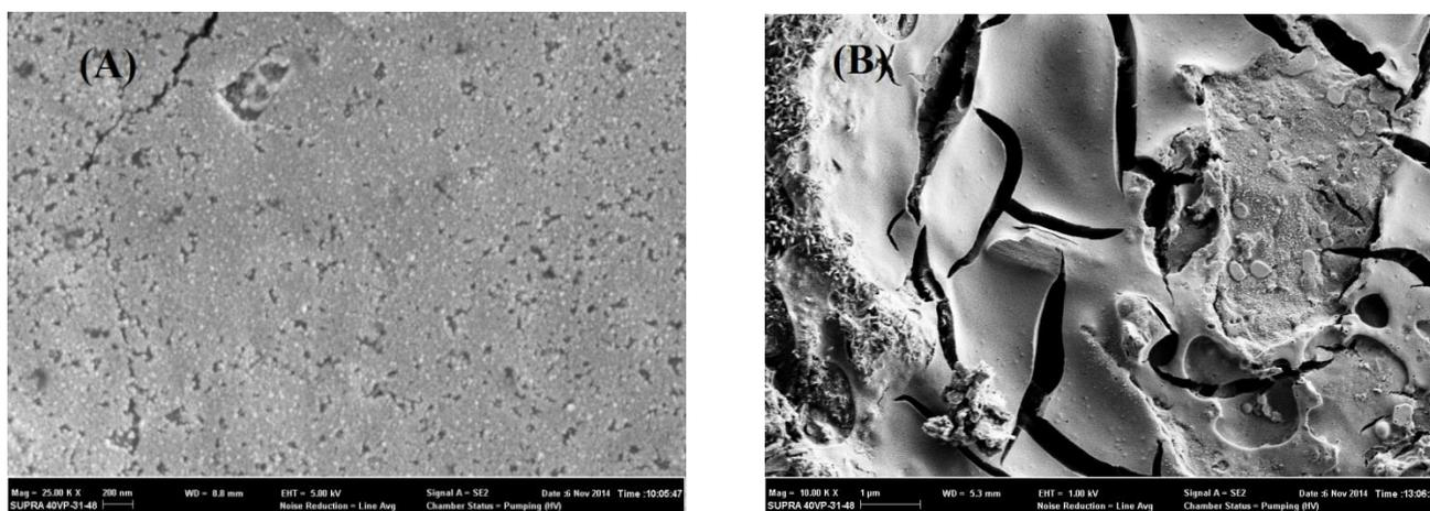
**Figure 1.** Scanning electron micrographs of (A) Pt and (B)  $\text{RuO}_2$  electrodes
