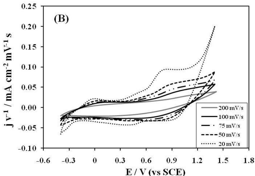
**Figure 6.** Normalized current density of the cyclic voltammetry measurement recorded on (A) Pt and (B) RuO<sub>2</sub> in 0.1 M KClO<sub>4</sub> containing 2 g/L paracetamol with the potential scan rates (20-200 mV/s) versus applied potential (j/v vs. E); CE: Pt, RE: SCE, T = 25 °C.
