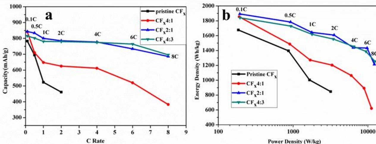
**Figure 4.** Comparison of (a) specific capacities of all the four cells vs. discharge current rate; (b) Energy density vs. power density (Ragone plot).
