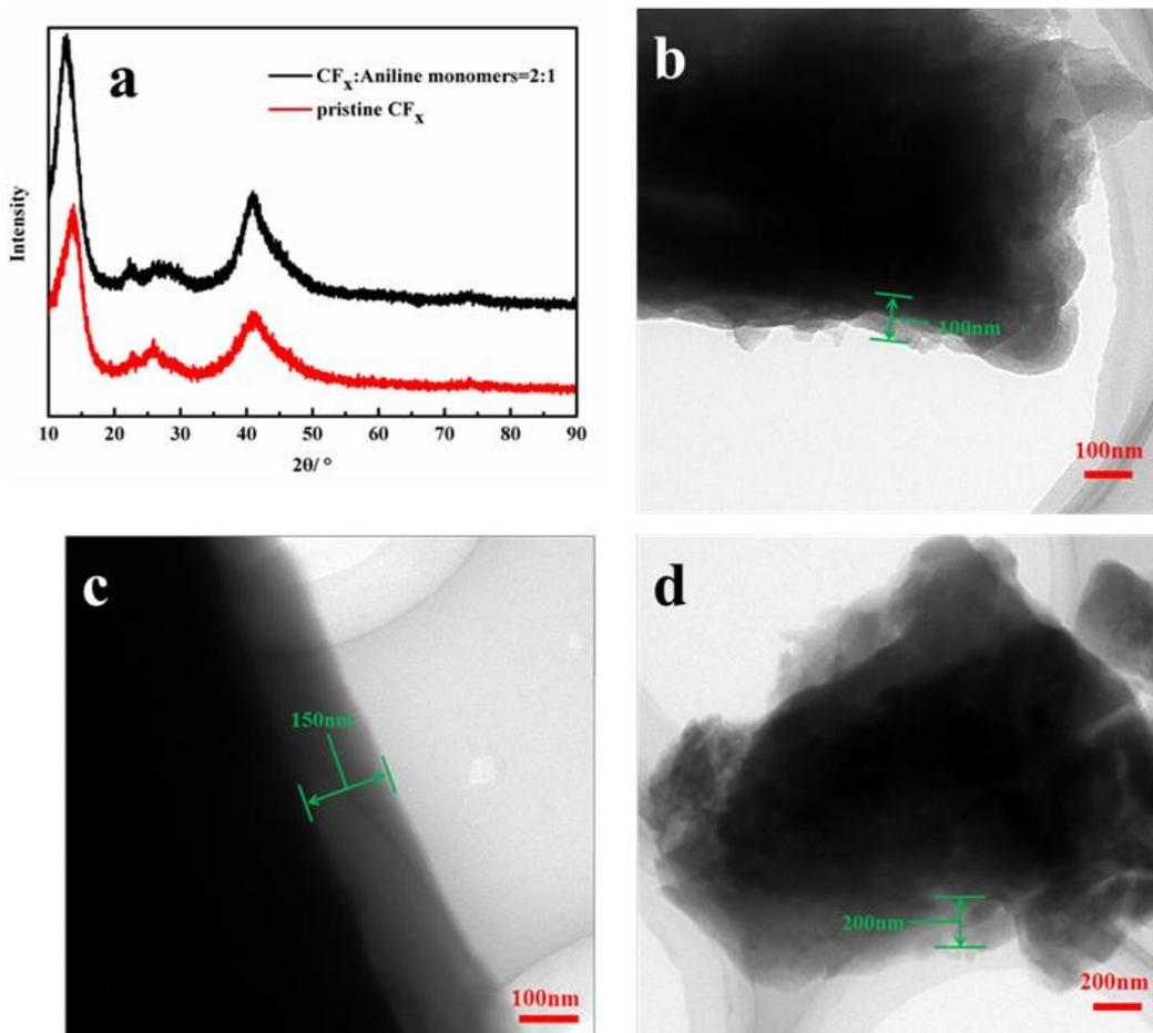
**Figure 2.** (a) XRD patterns of pristine  $\text{CF}_x$  and  $\text{CF}_x/\text{PANI}$  composite; TEM images of  $\text{CF}_x/\text{PANI}$  composites (b)  $\text{CF}_x4:1$ ; (c)  $\text{CF}_x2:1$ ; (d)  $\text{CF}_x4:3$ .
