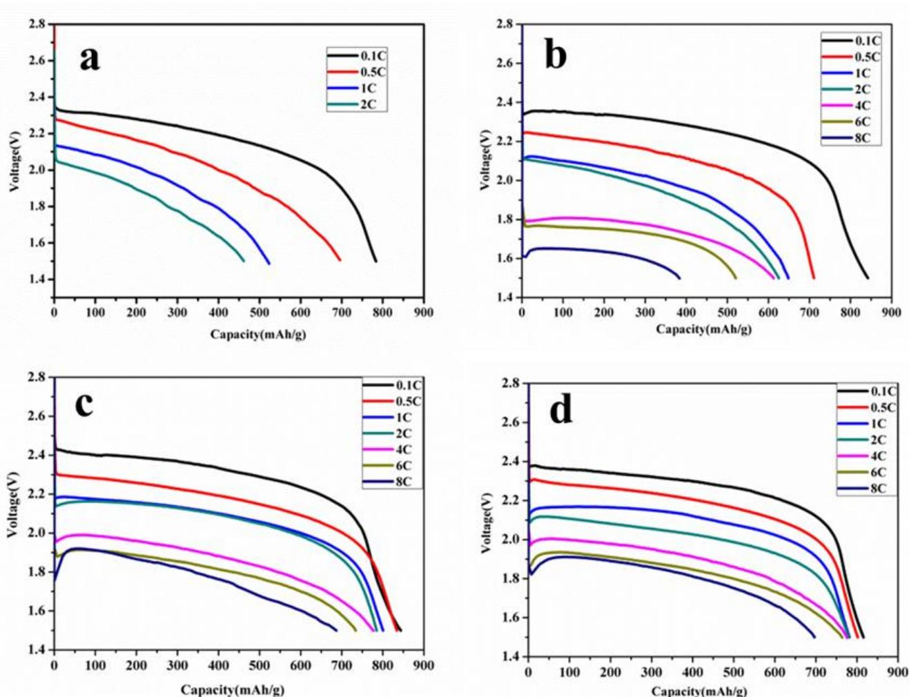
**Figure 3.** Galvanostatic discharge curves of (a) Pristine  $CF_x$ ; (b)  $CF_x$ 4:1; (c)  $CF_x$ 2:1; and (d)  $CF_x$ 4:3 obtained at different current densities.
