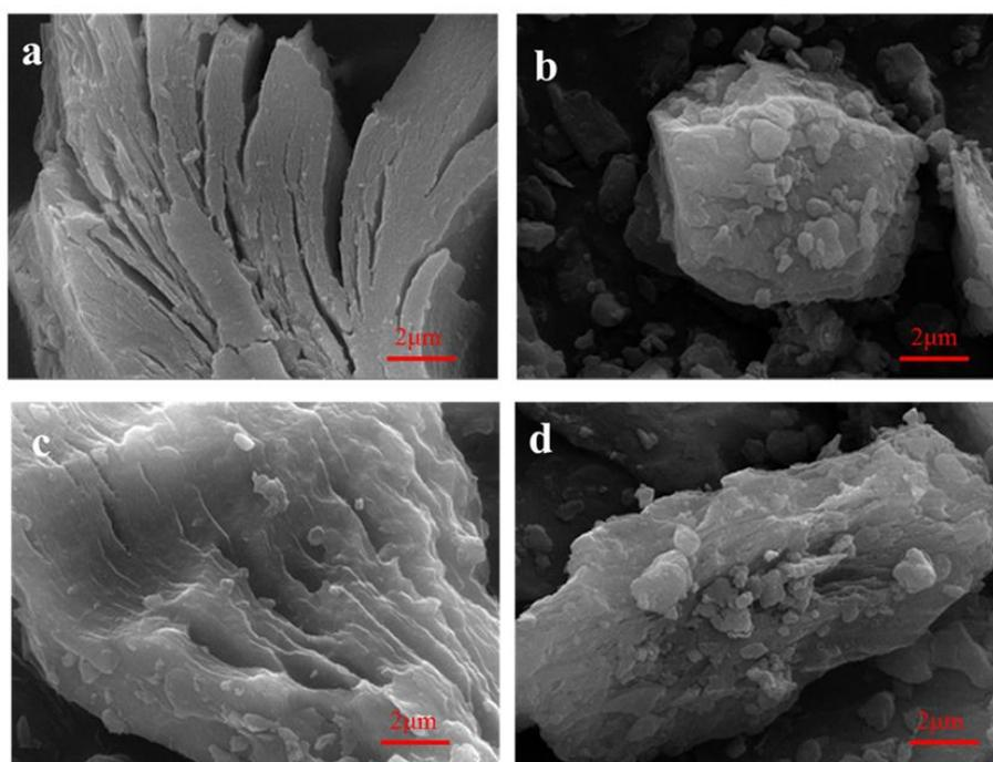
**Figure 1.** SEM images of  $\text{CF}_x$  samples before and after coated PANI (a) Pristine  $\text{CF}_x$ ; (b)  $\text{CF}_x4:1$ ; (c)  $\text{CF}_x2:1$ ; (d)  $\text{CF}_x4:3$ .
