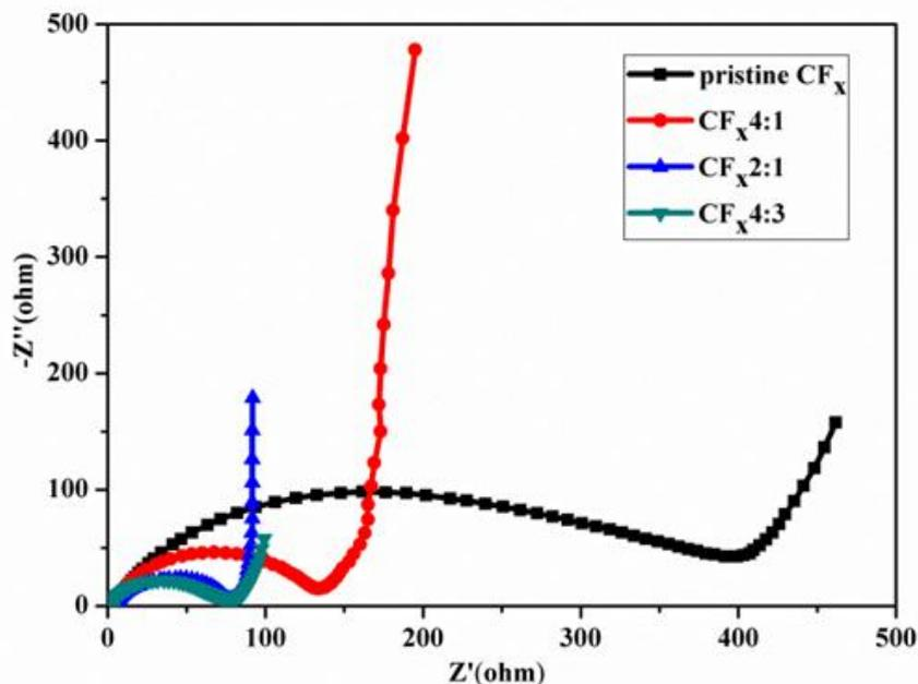
**Figure 5.** EIS patterns of pristine  $\text{CF}_x$  and  $\text{CF}_x/\text{PANI}$  composites; the EIS measurements were performed in the frequency range of 1 MHz to 0.1 Hz with an AC voltage amplitude of 5 mV at the open-circuit voltage.
