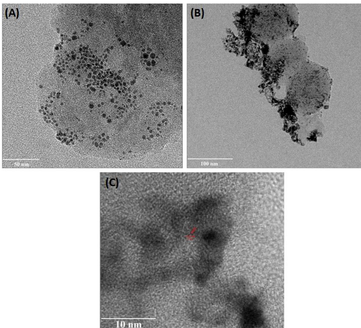
**Figure 3.** TEM images of (a) Pd-rGO, (b) Pt@Pd-rGO and (c) HRTEM image of Pt@Pd-rGO
