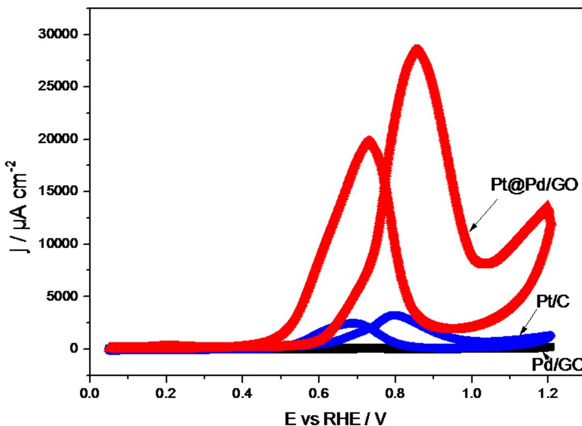
**Figure 8.** MOR activity for Pd-rGO, Pt@ Pd-rGO and 20% wt commercial Pt/C in 1M  $\text{CH}_3\text{OH}+0.1\text{M HClO}_4$  solution at 50 mVs.
