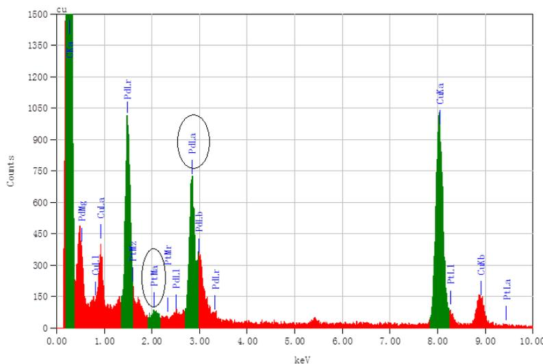
**Figure 6.** EDX analysis for Pt@Pd-rGO catalyst, which is showing presence of Pt and Pd. Atomic composition of Pd:Pt is 90.24:9.76 showing ultra-low loading of Pt.
