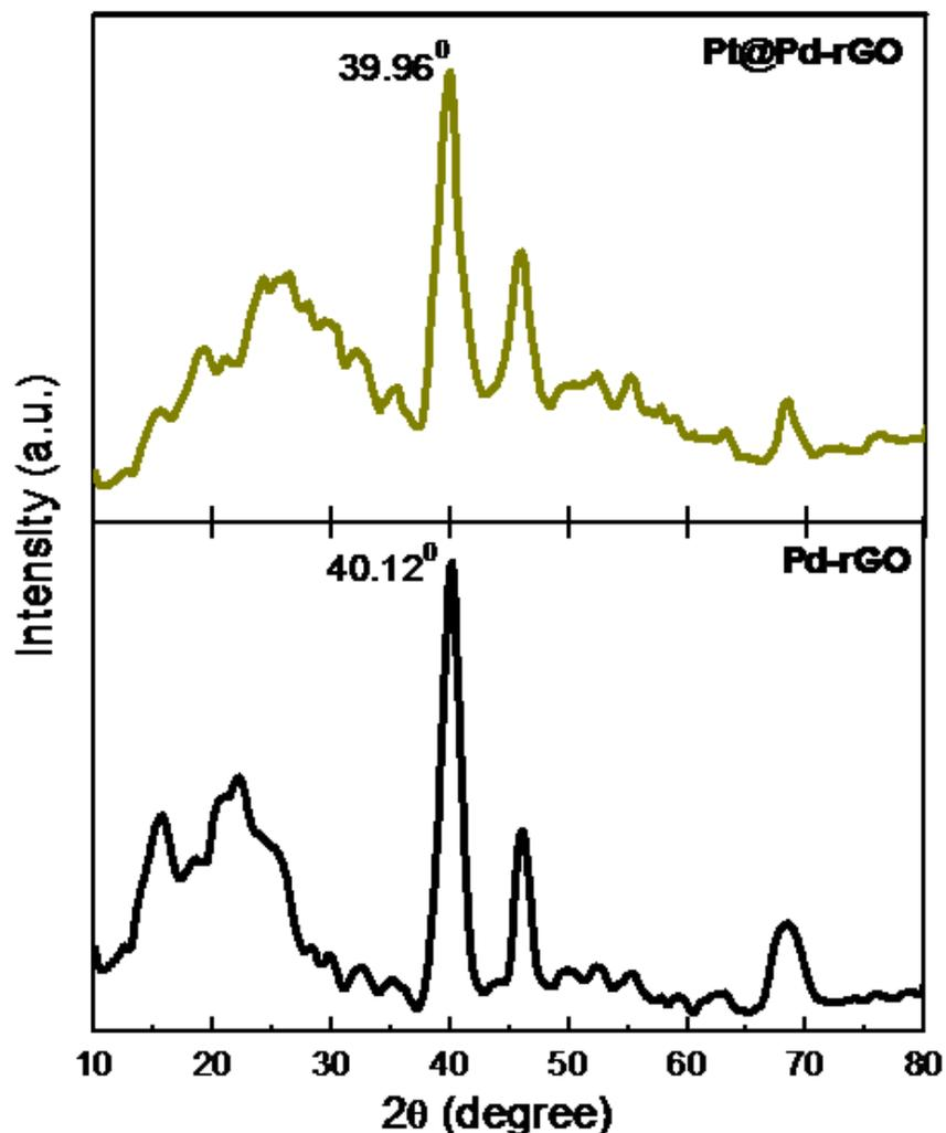
**Figure 4.** XRD spectrum of Pd/rGO and Pt@Pd/rGO catalysts.
