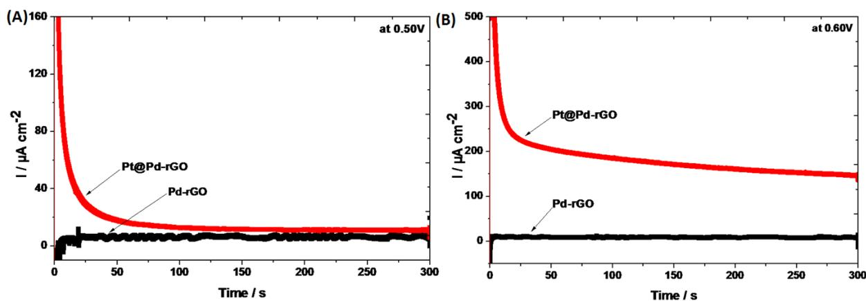
**Figure 9.** Chronoamperometric result of MOR activity for Pd-rGO and Pt@ Pd-rGO in 1M  $\text{CH}_3\text{OH}+0.1\text{M HClO}_4$  solution (A) at constant potential of 0.50V and (B) at constant potential of 0.60V
