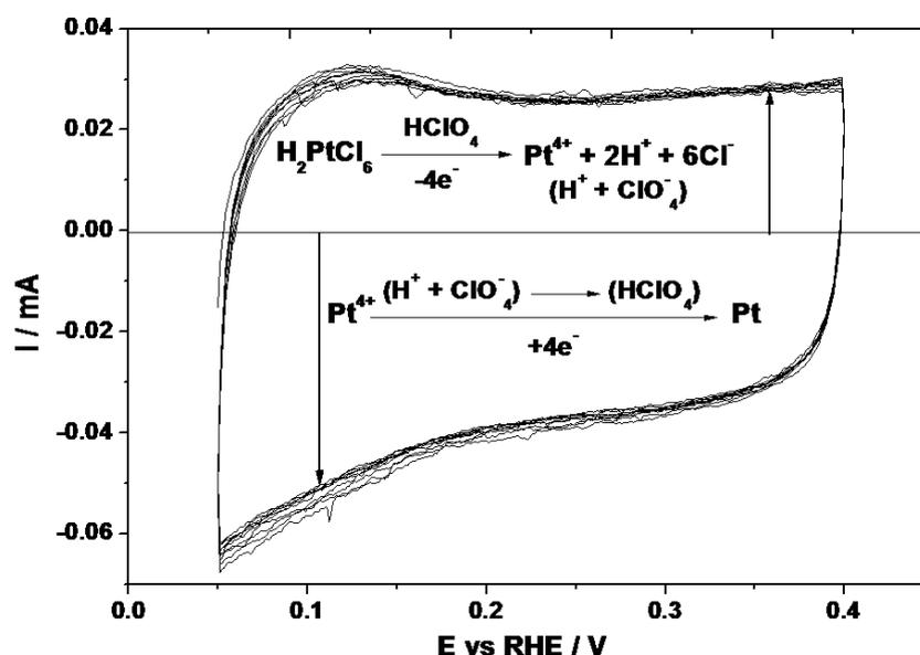
**Figure 5.** Electrochemical deposition of Pt on Pd-rGO NPs by potential cycling method in  $0.1\text{M HClO}_4+0.1\text{M H}_2\text{PtCl}_6$  solution at  $50\text{ mV/s}$ , with mechanism at positive scans and negative scans.
