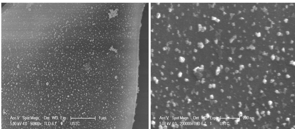
**Figure 1.** SEM images for Pd NPs supported on rGO, at two different magnifications.
