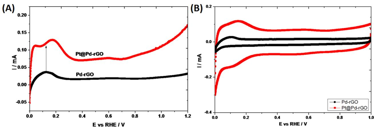
**Figure 7.** (A) LSV for Pd-rGO NPs and after deposition of Pt on them Pt@Pd-rGO NPs in 0.1M  $HClO_4$  solution at 50 mV/s and (B) Base CVs for Pd-rGO NPs and after deposition of Pt on them Pt@Pd-rGO NPs in 0.1M  $HClO_4$  solution at 50 mV/s.
