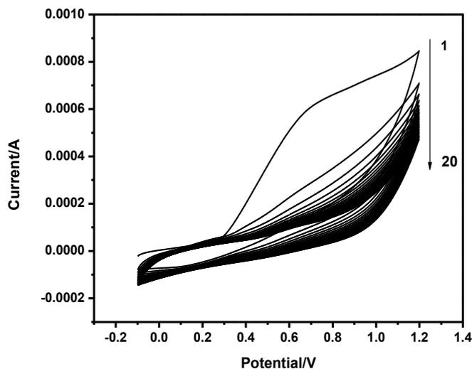
**Figure2.** Cyclic voltammograms of the copolymerization of Py and o-PD on a PGE.
