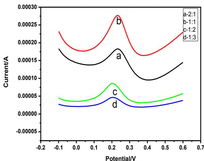
**Figure 4.** SWV curves of different ratios of Py and o-PD (a-d 2:1, 1:1, 1:2, 1:3 ).
