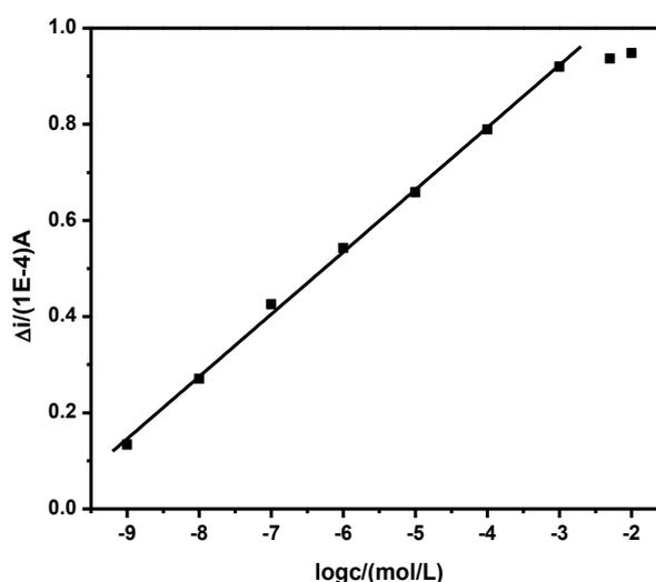
**Figure 8.** Plot of the peak current response ( $\Delta i$ ) versus logarithm of CPX concentration.
