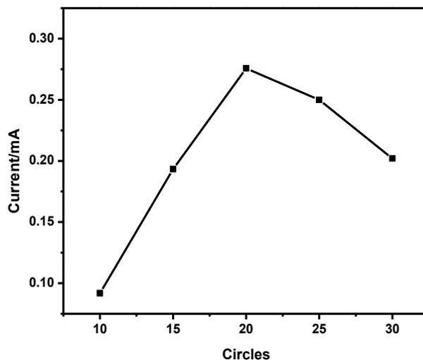
**Figure 5.** Recorded peak current of the sensor prepared with different CV cycles.
