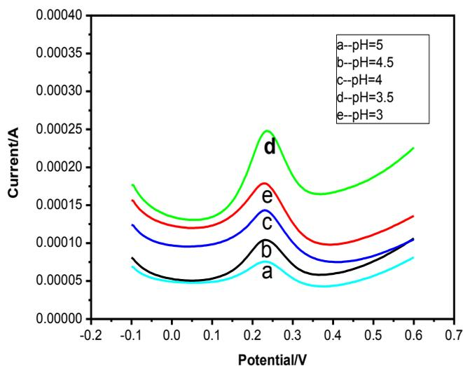
**Figure 3.** SWV curves of the MIP/PGE prepared in 0.05mol/L acetic acid buffer with different pH
