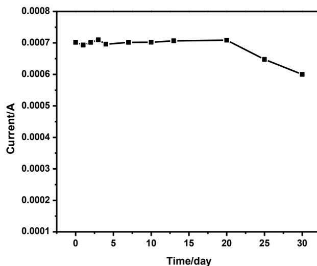
**Figure 10.** Stability of the MIP sensor stored at ambient conditions over 30 days.
