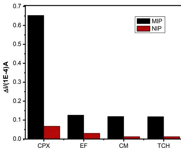
**Figure 9.** SWV responses of CPX and structural analogs on MIP and NIP sensor.
