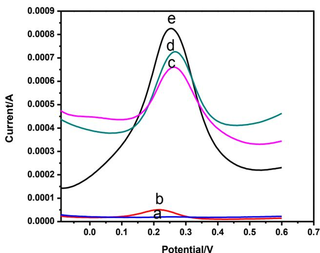
**Figure1.** SWVs of different electrodes. NIP/PGE (a), MIP/PGE with template(b), MIP/PGE rebinding template(c), MIP/PGE(d) and bare PGE(e).
