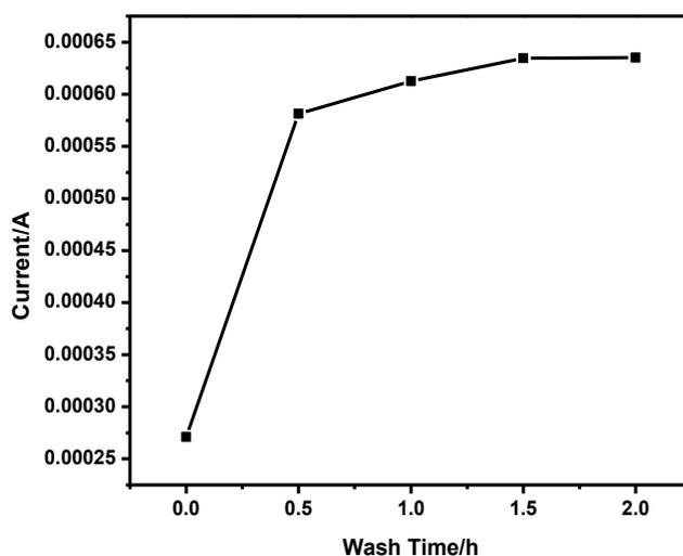
**Figure 6.** Recorded peak current from the sensor prepared under under optimized conditions immersing into the eluant for different time.
