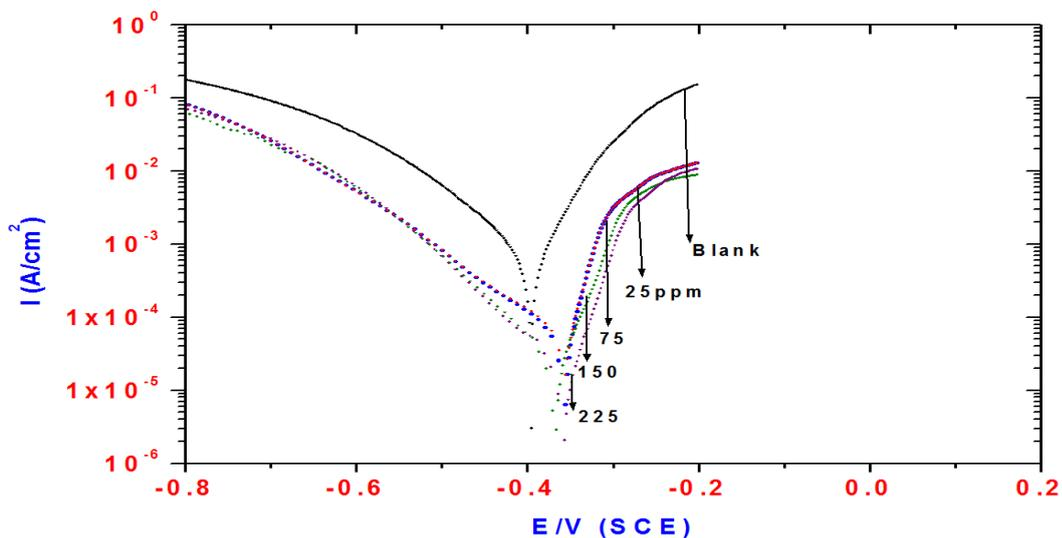
**Figure 2a.** The effect of DHMT concentration on the polarization curves of steel in acidic chloride solutions.
