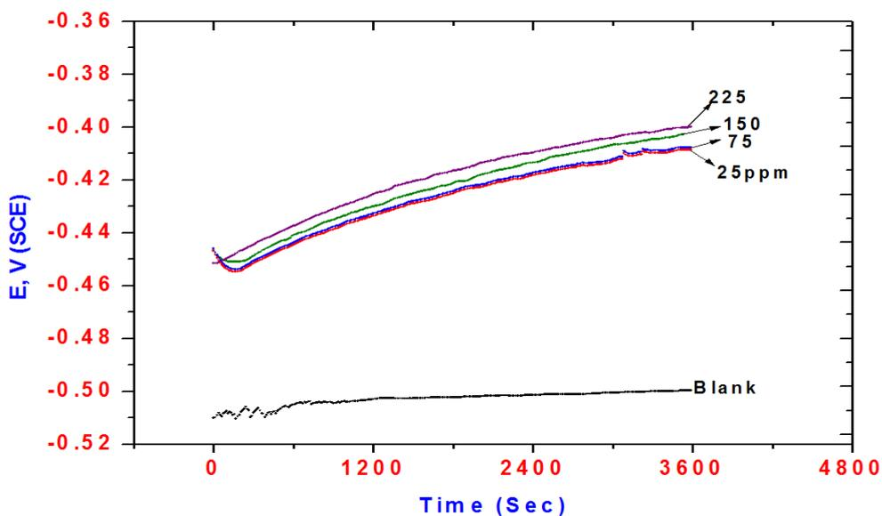
**Figure 1b.** The effect of DHPT concentration on the monitoring data of the open circuit potential of steel in the acidic chloride solution.
