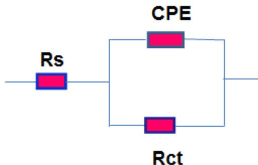
**Figure 4.** Equivalent circuit employed in fitting EIS data.
