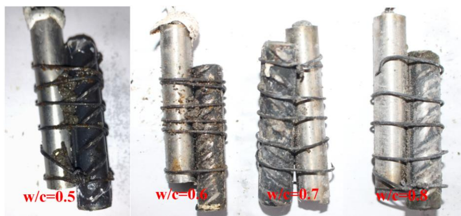
Figure 7. Corrosion states of the coupled stainless-carbon steel sample after 238 days.
