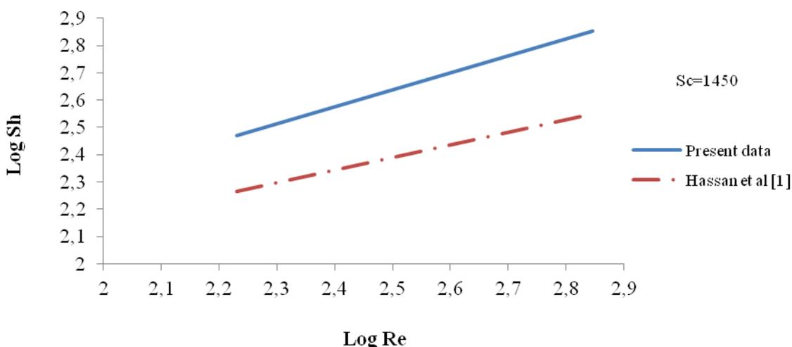
**Figure 5 .** Comparison between the present mass transfer data for Lessing rings and the data obtained by the electrochemical technique
