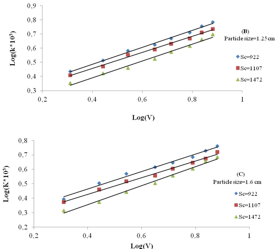
**Figure 3 .** Effect of superficial fluid velocity on the mass transfer coefficient for different Sc at different ring diameter
