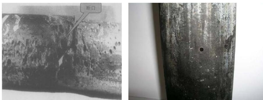
a) Tube fracture induced by corrosion    b) Corrosion perforation in the tube
