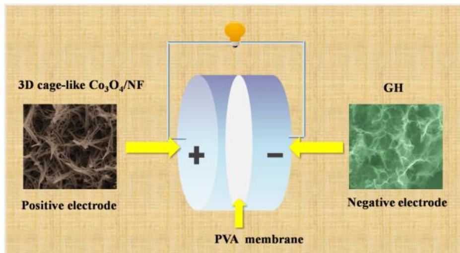
**Figure 6.** Schematic illustration of the asymmetric supercapacitor device.
