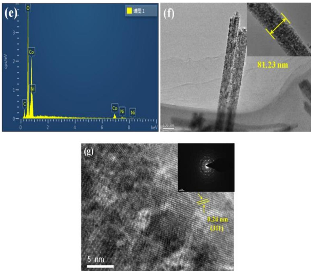
**Figure 3.** FESEM image of (a) pure nickel foam. (b-d) Low-resolution and high-resolution, (e) EDS spectrum of 3D cage-like  $\text{Co}_3\text{O}_4/\text{NF}$ . (f-g) low and high magnification TEM images (Inset in (g) the corresponding SAED pattern) of 3D cage-like  $\text{Co}_3\text{O}_4/\text{NF}$ .
