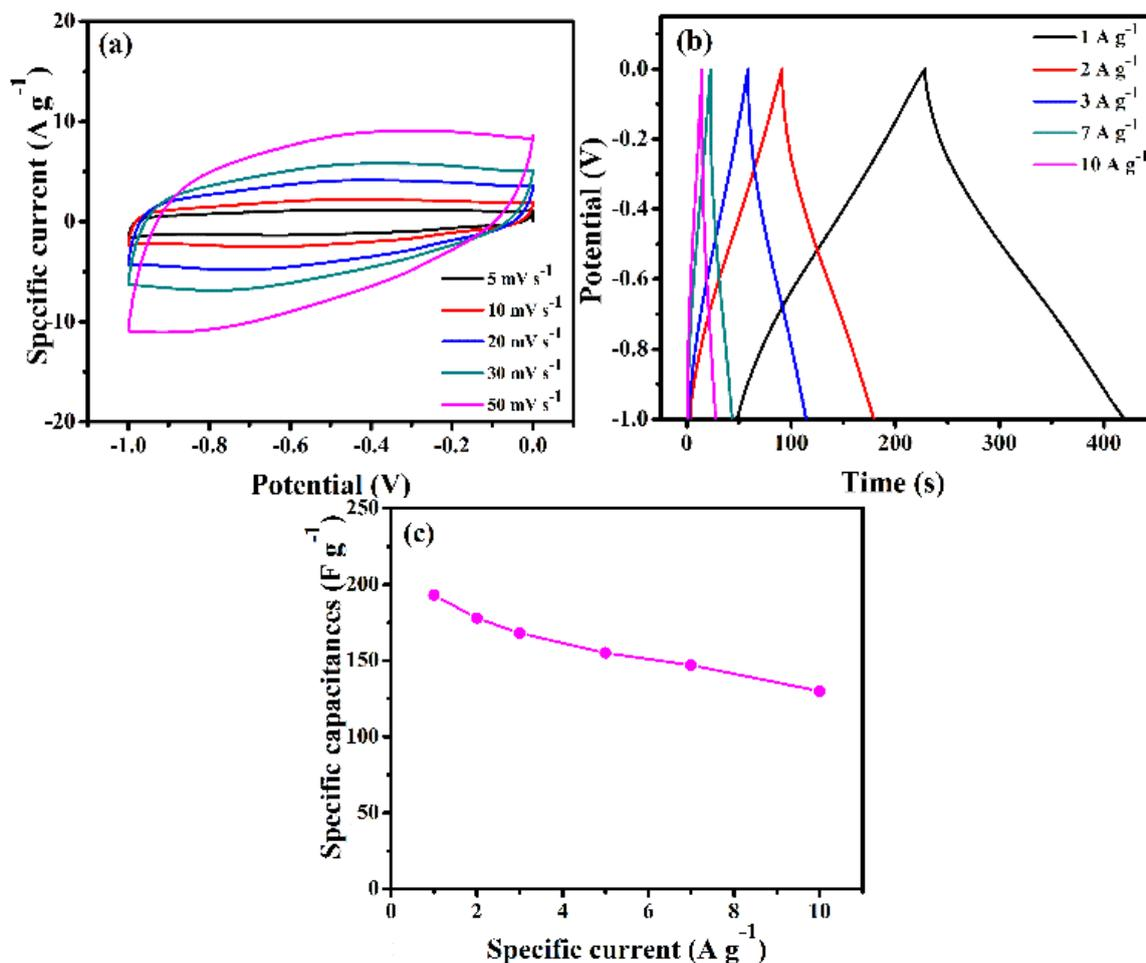
**Figure 5.** (a) Cyclic voltammograms at various scan rates. (b) Charge-discharge curves under different current density. (c) Average specific capacitance at various discharge current densities of the GH electrode.
