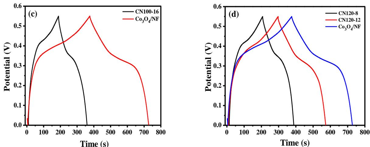
Figure S2 CV curves of (a) the pristine nickel foam, CN100-16, Co<sub>3</sub>O<sub>4</sub>/NF at 5 mV s<sup>-1</sup>. (b) the pristine nickel foam, CN120-8, CN120-12, Co<sub>3</sub>O<sub>4</sub>/NF. GCD curves of (c) the CN100-16 and Co<sub>3</sub>O<sub>4</sub>/NF, (d) the as-prepared CN120-8, CN120-12, Co<sub>3</sub>O<sub>4</sub>/NF electrodes at 1 A g<sup>-1</sup>.
