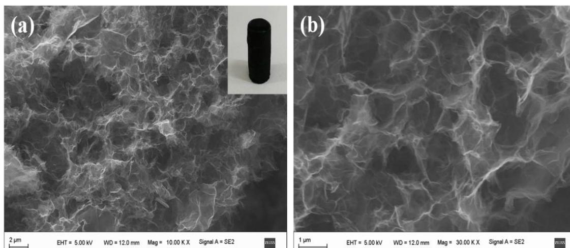
Figure S3 (a) Low-resolution (b) high-resolution of the SEM image of GH.
