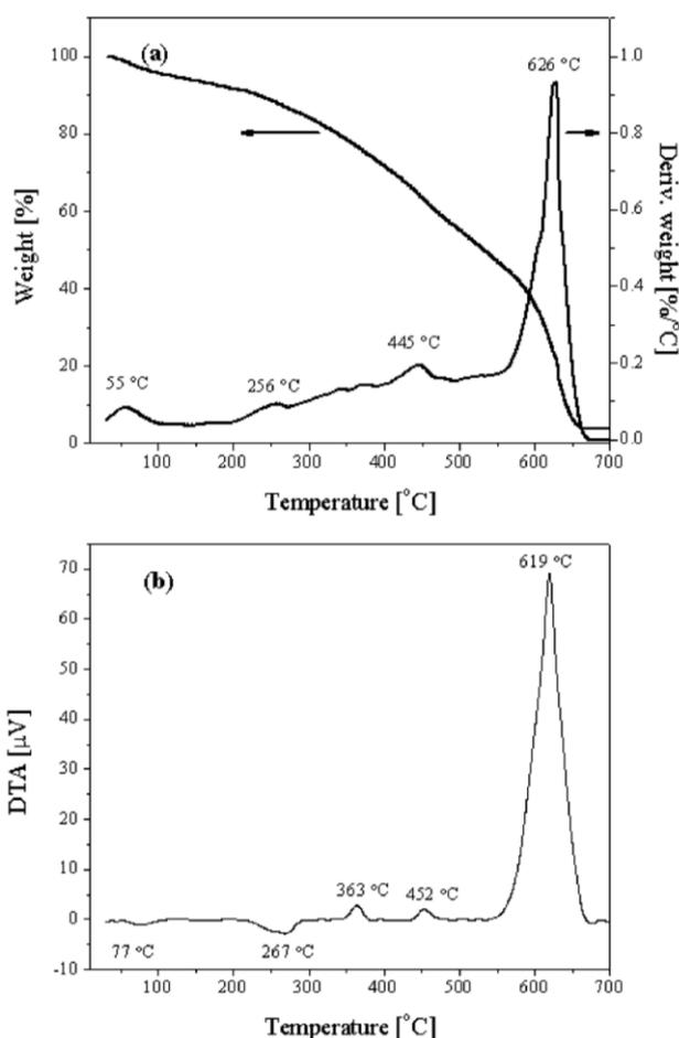
**Figure 6.** TGA (a) and DTA (b) thermograms obtained for the electrodeposited layer of PPy-sCNTs analyses at a heating rate of 10 °C/min in air flow (40 ml/min).
