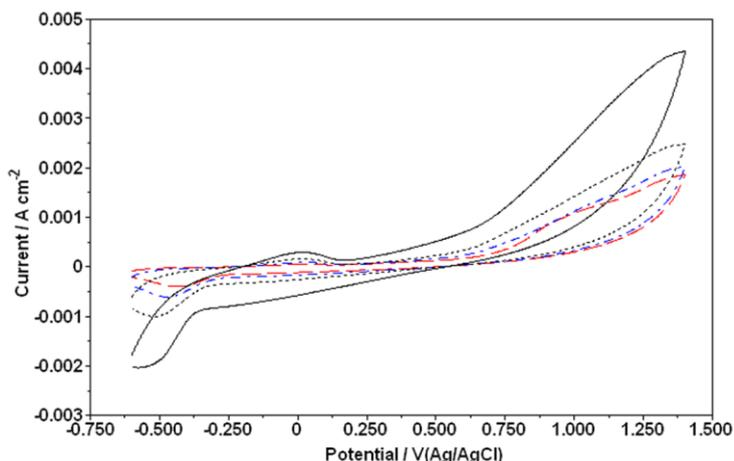
**Figure 1.** Selected successive cycles (no. 3, 10, 15, 25) of cyclic voltammetry (scan rate 50 mV s<sup>-1</sup>) of PPy on Al from 0.4M oxalic acid containing 0.2M pyrrole at room temperature.
