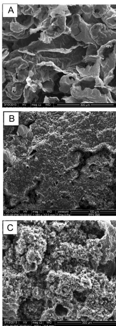
**Figure 3.** SEM micrographs at low magnification (x100) of PPy (A), PPy-sCNTs (B) and PPy-NiLa (C) after 30 cycles electrodeposition.
