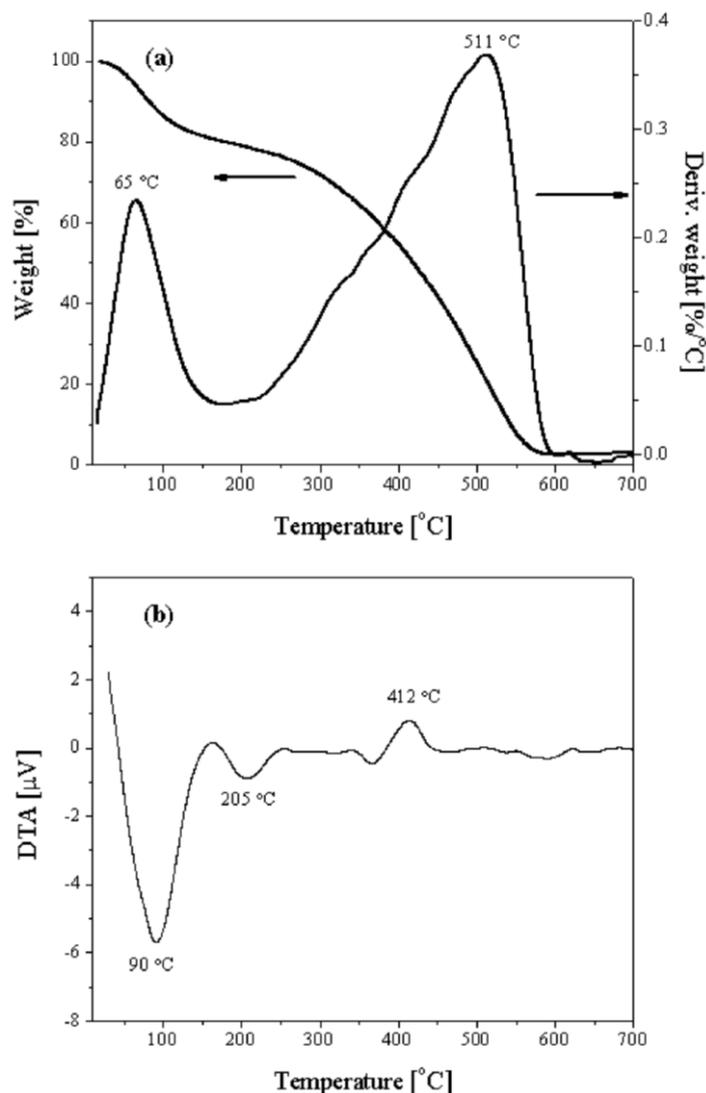
**Figure 7.** TGA (a) and DTA (b) thermograms obtained for the electrodeposited layer of PPy-NiLa analyses at a heating rate of 10 °C/min in air flow (40 ml/min).
