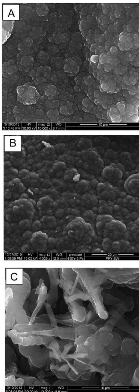
**Figure 4.** SEM high magnification micrographs at high magnification (x1500) of PPy (A), PPy-sCNTs (B) and PPy-NiLa (C) after 30 cycles electrodeposition.
