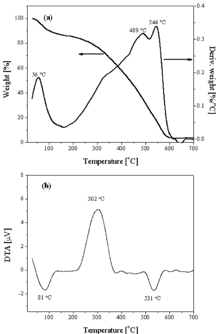
**Figure 5.** TGA (a) and DTA (b) thermograms obtained for the electrodeposited layer of PPy analyses at a heating rate of 10 °C/min in air flow (40 ml/min).
