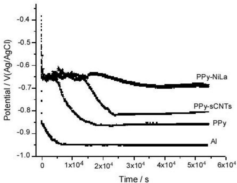
**Figure 9.** Potential-time relation of Al and different coated Al electrodes in 0.1M NaCl at room temperature.
