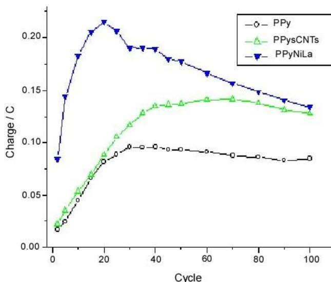
**Figure 2.** Electrodeposition rate of PPy and its nanocomposites on Al from 0.4M oxalic acid electrolyte solution containing monomer and nanoparticles at room temperature.
