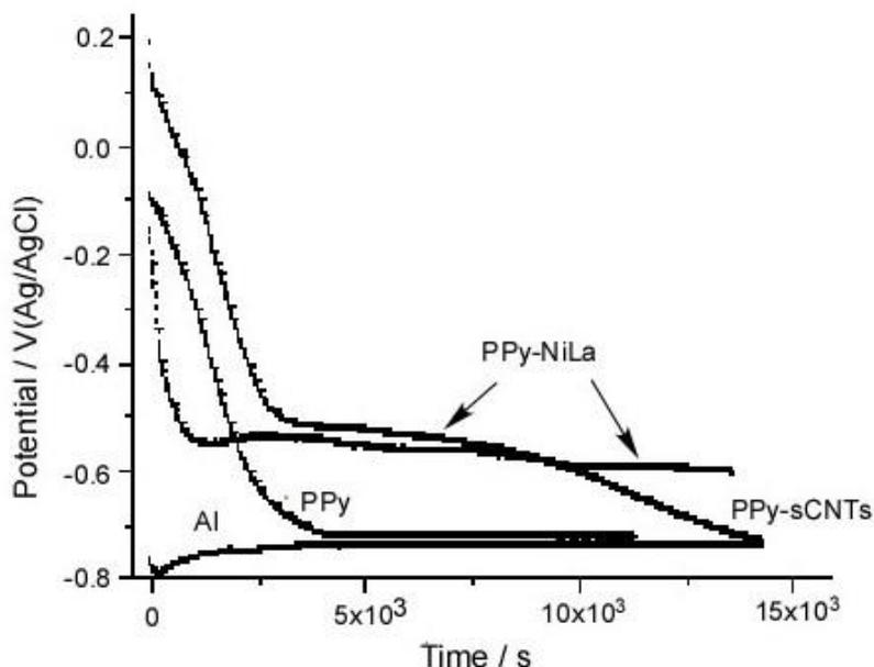
**Figure 8.** Potential-time relation of Al and different coated Al electrodes in 0.5M H<sub>2</sub>SO<sub>4</sub> at room temperature.
