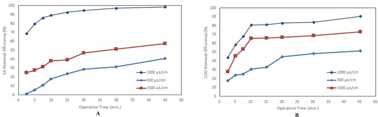
**Figure 8.** Effect of solution conductivity on removal efficiency for SA (A) and COD (B) (Operating conditions: Al-Al-Al-Al electrode, initial pH = 6, current density = 50 A/m<sup>2</sup>, air injection flow= 2L/min, and electrode connection mode = MP-P).
