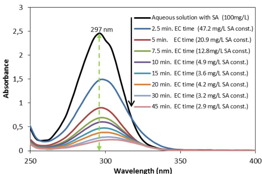
**Figure 10.** UV-Vis spectra of the raw and treated water at 2.5-45 min reaction times.
