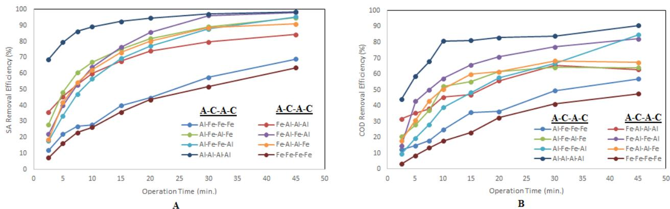
**Figure 3.** Effect of hybrid electrode types on removal efficiency for SA (A) and COD (B) (A: Anode, C: Cathode) (Operating conditions: pH = 6, current density = 50 A/m<sup>2</sup>, SA concentration = 100 mg/L, air injection flow = 2 L/min, solution conductivity = 1000μs/cm, and electrode connection mode = MP-P).
