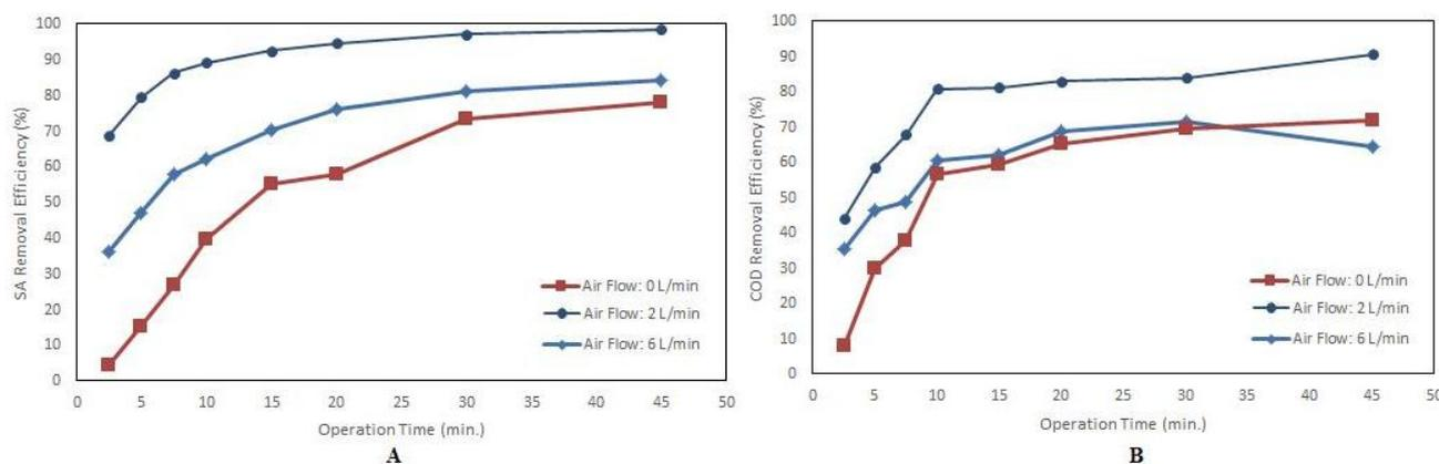
**Figure 7.** Effect of air injection flow on removal efficiency for SA (A) and COD (B) (Operating conditions: Al-Al-Al-Al electrode, initial pH = 6, current density = 50 A/m<sup>2</sup>, solution conductivity = 1000µs/cm, and electrode connection mode = MP-P).
