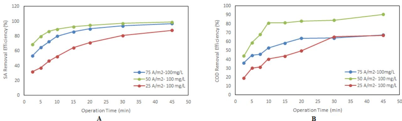
**Figure 5.** Effect of current density on removal efficiency for SA (A), and COD (B) (Operating conditions: Al-Al-Al-Al electrode, initial pH = 6, initial SA concentration: 100 mg/L, solution conductivity =  $1000\mu s/cm$ , air injection flow = 2 L/min and electrode connection mode = MP-P).
