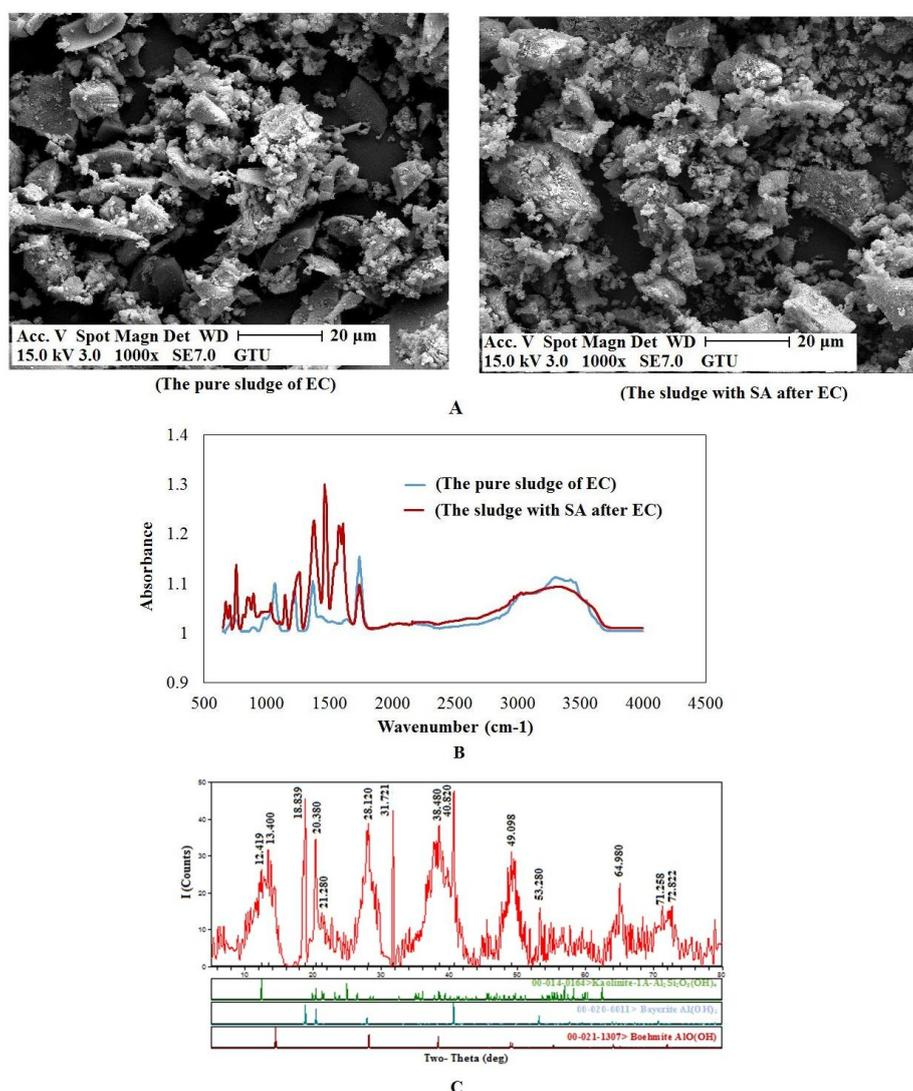
**Figure 11.** (A) SEM micrograph, (B) FT-IR spectrum and XRD analysis of EC sludge after removal of SA from aqueous water solution using Al-Al-Al-Al electrode pairs.
