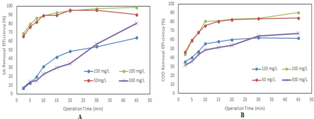
**Figure 6.** Effect of initial SA concentration on removal efficiency for SA (A) and COD (B) (Operating conditions: Al-Al-Al-Al electrode, initial pH = 6, current density = 50 A/m<sup>2</sup>, air injection flow = 2 L/min, solution conductivity = 1000µs/cm, and electrode connection mode = MP-P).
