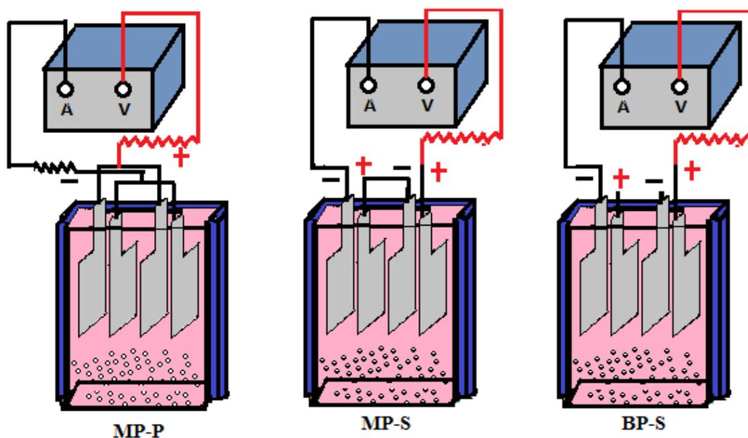
**Figure 2.** Schematic diagram of three different electrode connection modes.
