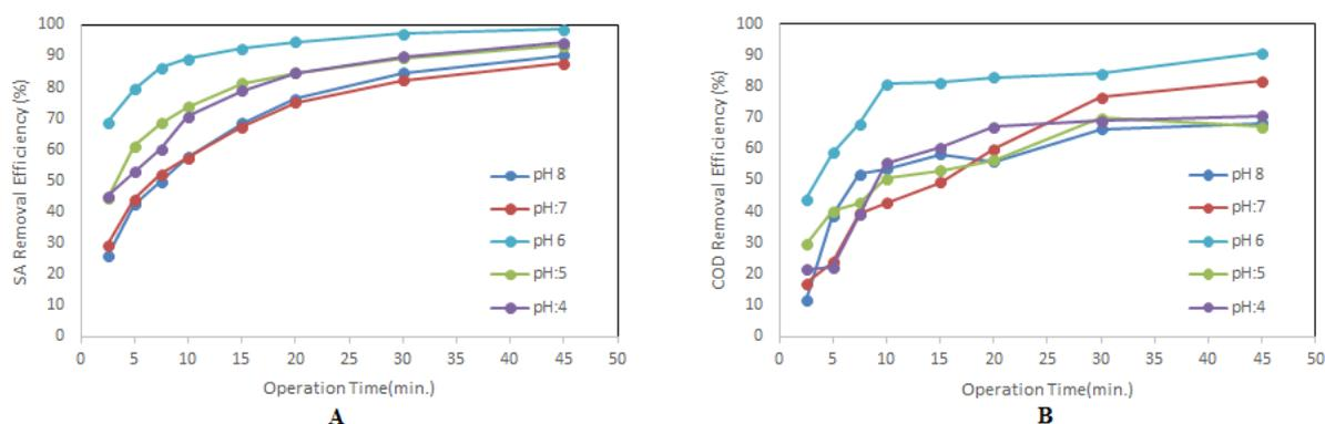
**Figure 4.** Effect of initial pH levels on removal efficiencies for SA (A), and COD (B) (Operating conditions: Al-Al-Al-Al electrode, current density =  $50 \text{ A/m}^2$ , initial SA concentration:  $100 \text{ mg/L}$ , air injection flow =  $2 \text{ L/min}$ , solution conductivity =  $1000 \mu\text{s/c}$ , and electrode connection mode = MP-P).
