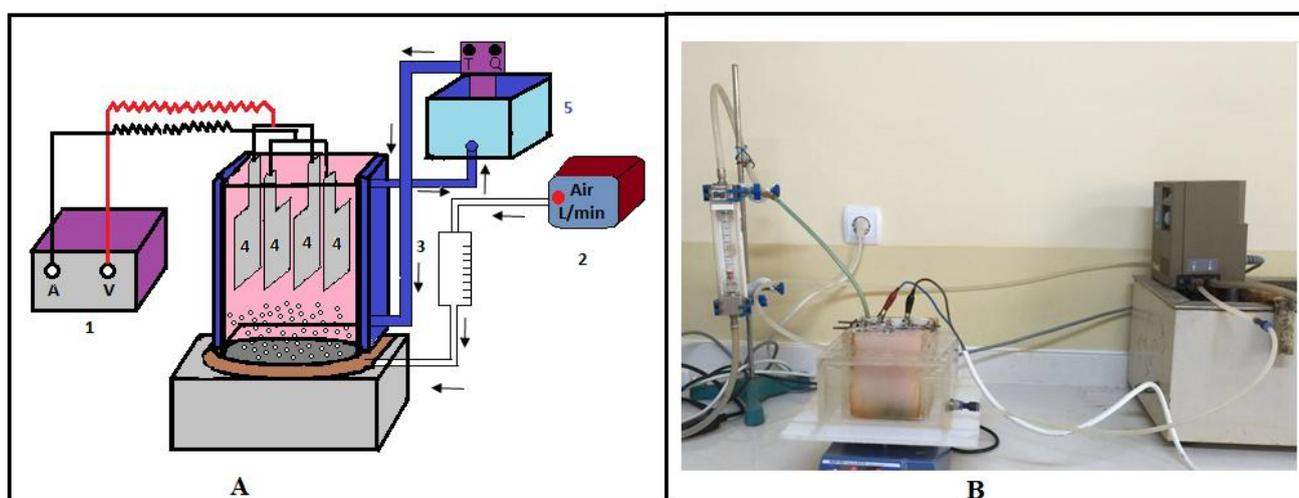
**Figure 1.** Schematic diagram (A) and photograph (B) of electrocoagulation process (1. Power supply, 2. Air flowmeter, 3. EC reactor, 4. Al, Fe or Al-Fe hybrid electrodes, 5. Water circulator).
