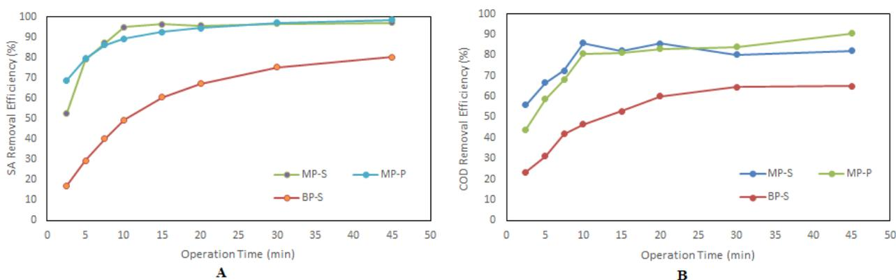
**Figure 9.** Effect of electrode connection mode on removal efficiency for SA (A), and COD (B) (Operating conditions: Al-Al-Al-Al electrode, initial pH = 6, current density = 50  $\text{A}/\text{m}^2$ , air injection flow = 2L/min. and solution conductivity = 1000  $\mu\text{s}/\text{cm}$ ).
