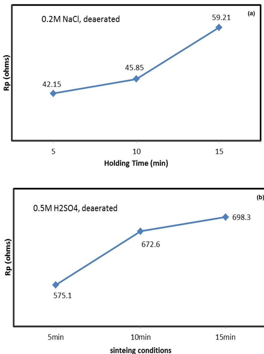
**Figure 5.** Polarization resistance ( $R_p$ ) values versus time for Fe-18Cr-2Si specimens in deaerated, (a) 0.2M NaCl solution, and ( b) 0.5M H<sub>2</sub>SO<sub>4</sub> solution at room temp respectively.
