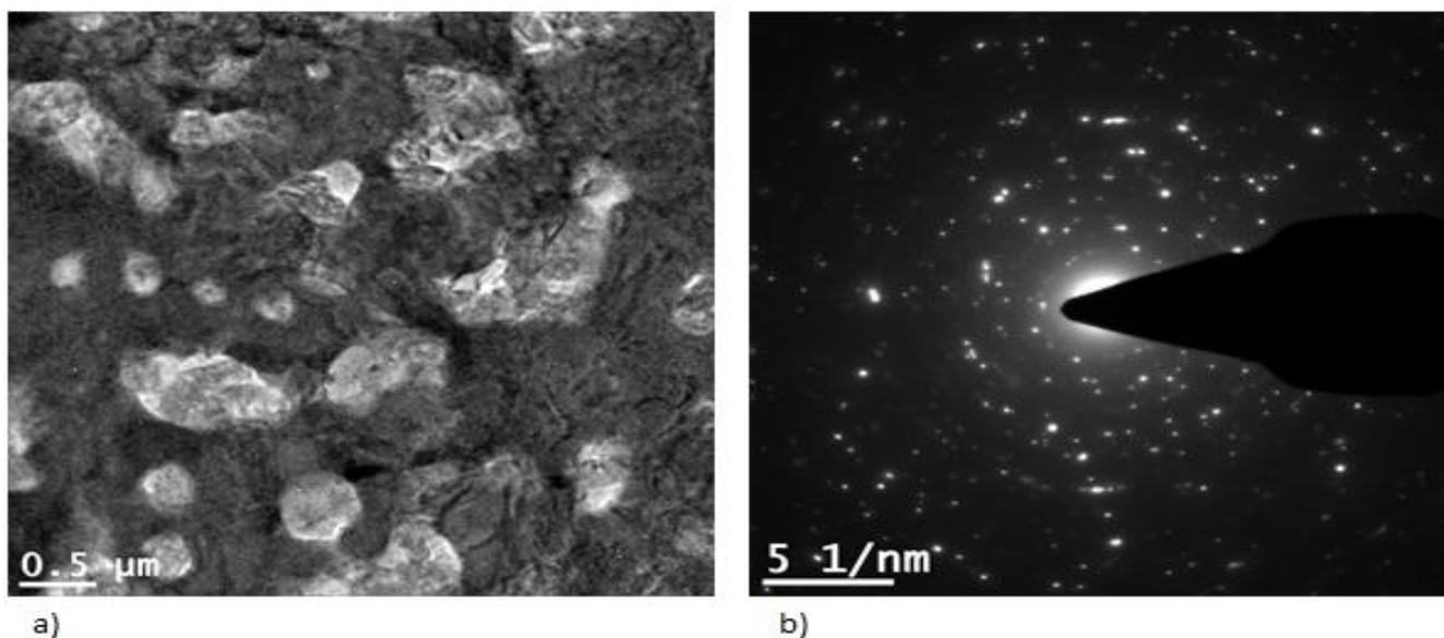
**Figure 3.** Microstructure of Fe-18Cr-2Si sintered alloy (a)FE- TEM image, (b) SAED pattern
