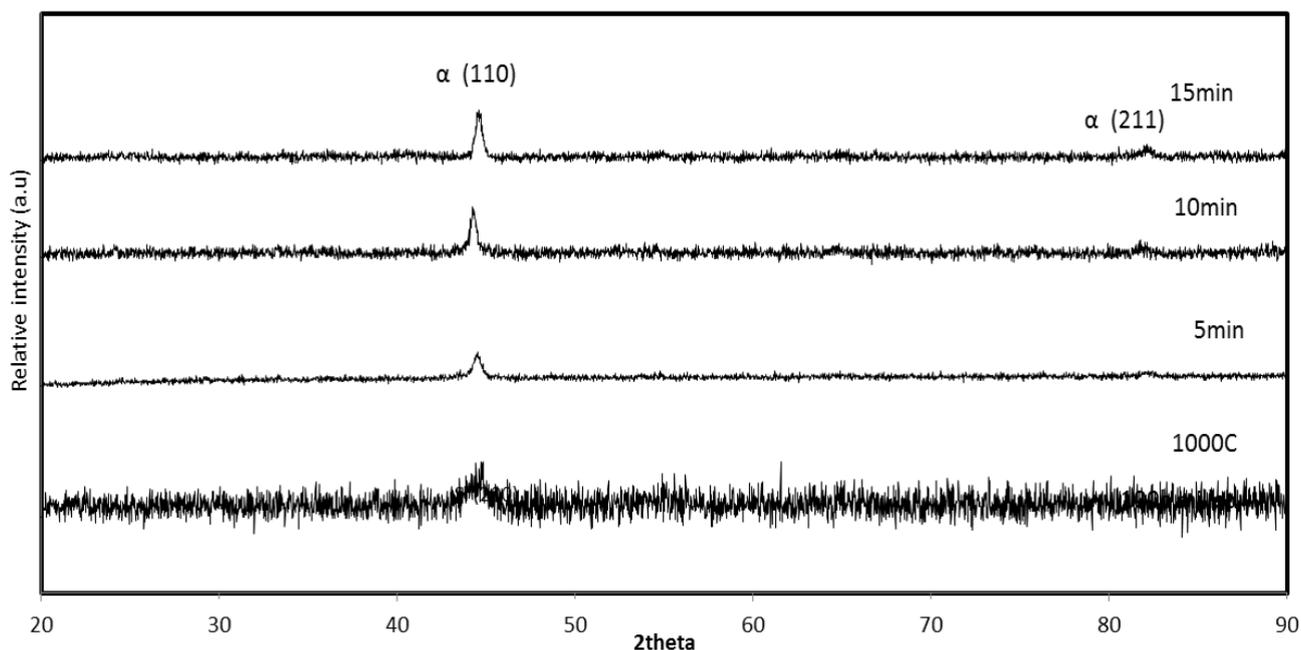
**Figure 1.** XRD patterns of spark plasma sintered Fe-18Cr-2Si powders at different sintering times, together with XRD spectra of 100 h milled powder.
