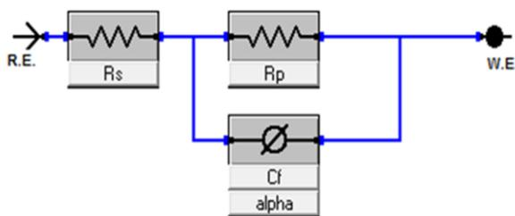
**Figure 7.** Constant phase element (CPE) model used to fit EIS data (Nyquist plot) in Figure 6
