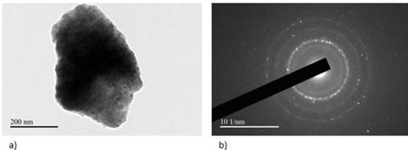
**Figure 2.** TEM bright-field images and selected area electron diffraction patterns of; (a) Fe-18Cr-2Si powder milled for 100 h (b) Micrograph of powder milled for 100 h showing the presence of BCC crystalline phase, confirmed from the diffraction pattern
