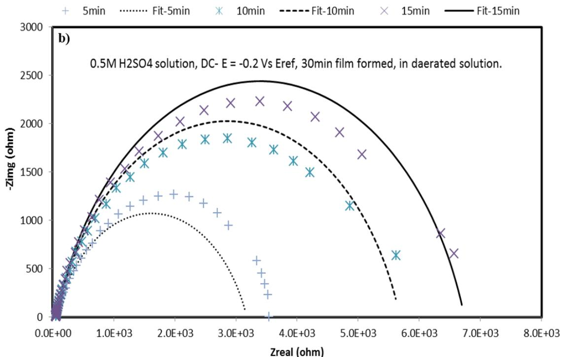
**Figure 6.** Nyquist plot of Fe-18Cr-2Si sintered specimens at different times together with CPE model curve fitting in deaerated (a) 0.2M NaCl solution, and ( b) 0.5M H2SO4 solution at room temp., respectively.
