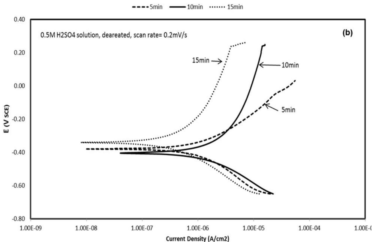
**Figure 4.** Potentiodynamic polarization response of Fe-18Cr-2Si specimens in deaerated, (a) 0.2M NaCl solution, and (b) 0.5M H<sub>2</sub>SO<sub>4</sub> solution at room temp respectively.
