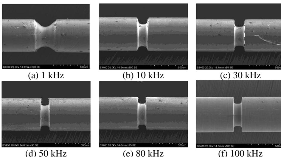
**Figure 4.** SEMs of grooves fabricated at different frequencies (applied voltage: 11 V, 10%; electrolyte: 15 g/L; spindle speed: 3000 rpm; and feed rate 0.1  $\mu\text{m/s}$ )
