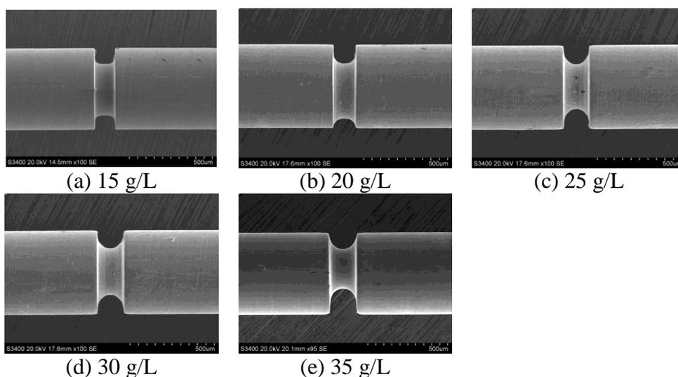
**Figure 8.** SEMs of grooves fabricated at different electrolyte concentrations (applied voltage: 11 V, 10%, 100 KHz; spindle speed: 3000 rpm; and feed rate 0.1 µm/s)
