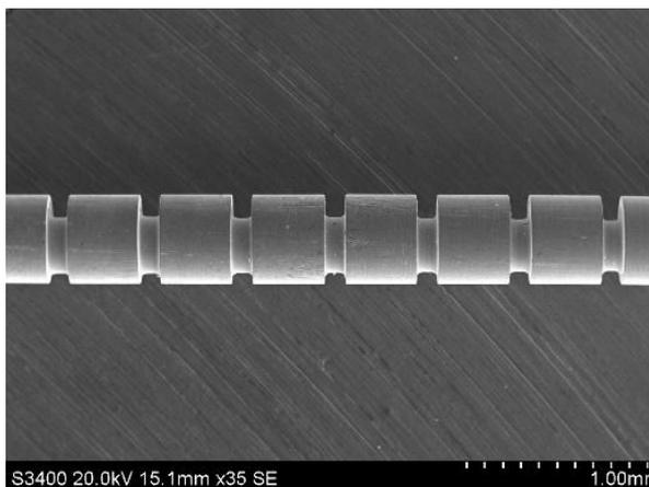
**Figure 9.** SEM image of ribbed wire electrode (applied voltage: 11 V, 10%, 100 KHz; electrolyte: 15 g/L; spindle speed: 3000 rpm; and feed rate 0.1  $\mu\text{m/s}$ )
