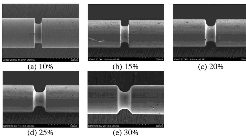
**Figure 6.** SEMs of grooves fabricated at different duty cycles (applied voltage: 11 V, 100 KHz; electrolyte: 15 g/L; spindle speed: 3000 rpm; and feed rate 0.1  $\mu\text{m/s}$ )
