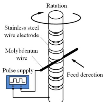
**Figure 1.** Schematic diagram of WECMM for preparing a ribbed wire electrode
