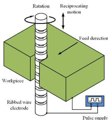
**Figure 10.** Schematic diagram of electrochemical micromachining with a ribbed wire electrode
