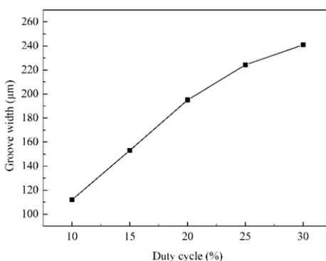
**Figure 5.** Variation of groove width with duty cycle (applied voltage: 11 V, 100 KHz; electrolyte: 15 g/L; spindle speed: 3000 rpm; and feed rate 0.1  $\mu\text{m/s}$ )
