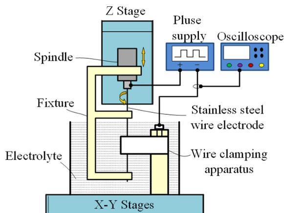
**Figure 2.** Experimental setup for WECMM
