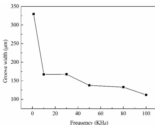
**Figure 3.** Variation of groove width with pulse frequency (applied voltage: 11 V, 10%; electrolyte: 15 g/L; spindle speed: 3000 rpm; and feed rate 0.1  $\mu\text{m/s}$ )
