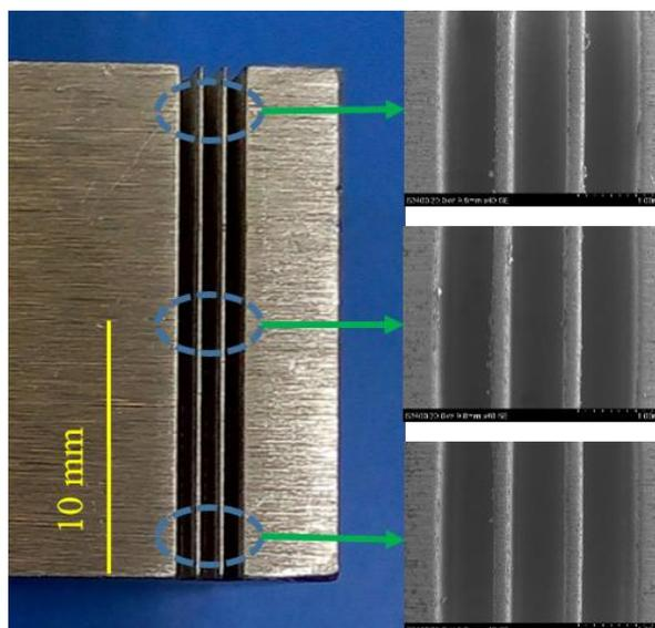
**Figure 11.** Machined high-aspect-ratio microstructure (applied voltage: 21 V, 40%, 100 KHz; electrolyte: 15 g/L; spindle speed: 5000 rpm; feed rate: 1  $\mu\text{m/s}$ ; reciprocating frequency: 1.5 Hz; and reciprocating amplitude: 20 mm)
