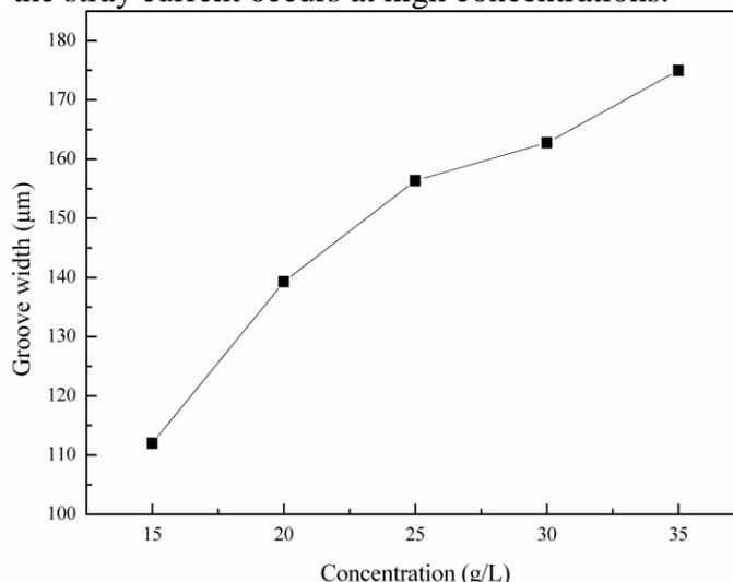
**Figure 7.** Variation of groove width with electrolyte concentration (applied voltage: 11 V, 10%, 100 KHz; spindle speed: 3000 rpm; and feed rate 0.1 µm/s)
