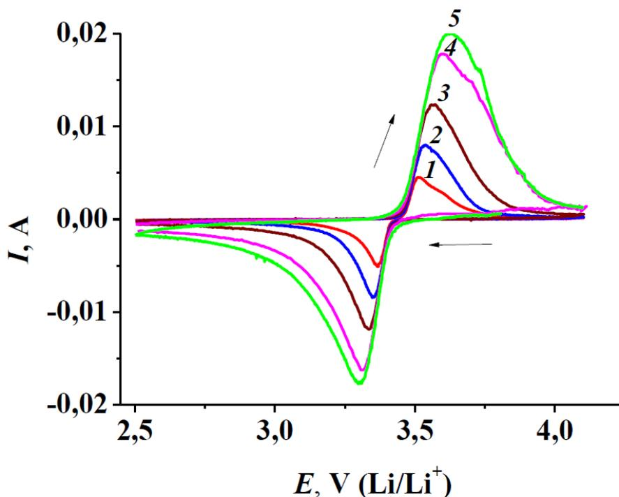
**Figure 8.** The cyclic voltammograms of  $\text{Li}_{0.99}\text{Fe}_{0.98}\text{Cr}_{0.01}\text{Ni}_{0.01}\text{PO}_4/\text{C}$  sample. Potential scan rates (V/s): 1 – 0.0001, 2 – 0.0002, 3 – 0.0004, 4 – 0.0008, 5 – 0.001. Weight of the sample is 0.015 g. Visible area of the electrode surface is  $2.25 \text{ cm}^2$ .
