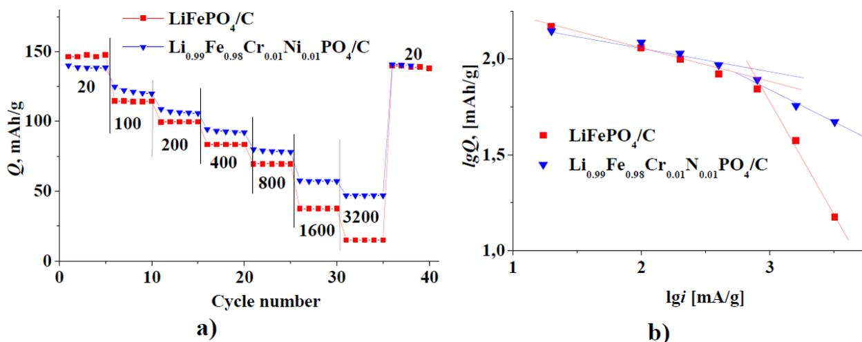
**Figure 7.** Change of discharge capacity during the cycling (a) and dependence of discharge capacity on the current density in logarithmic coordinates (b) for lithium iron phosphate samples. Current density in [mA/g] is shown in the Fig. 7a.
