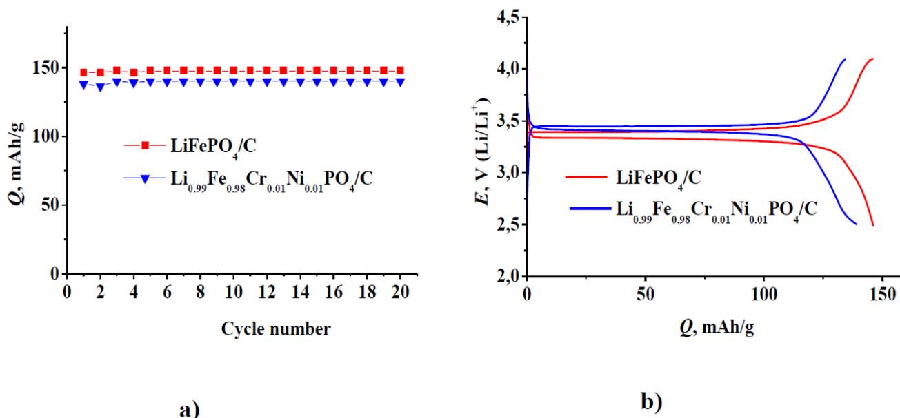
**Figure 6.** Change of discharge capacity during the cycling (a) and charge-discharge curves (b) of lithium iron phosphate samples. The current density is 20 mA/g.
