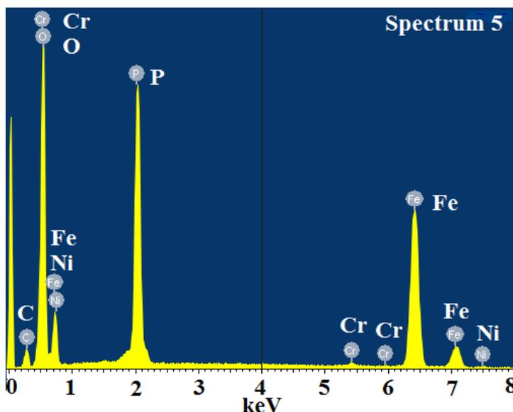
Figure 5. EDX spectrum of  $\text{Li}_{0.99}\text{Fe}_{0.98}\text{Ni}_{0.01}\text{Cr}_{0.01}\text{PO}_4/\text{C}$
