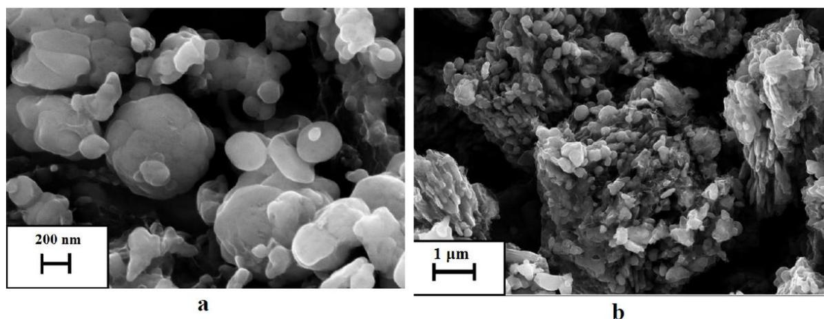
Figure 2. SEM micrographs of LiFePO<sub>4</sub>/C taken at different magnification (a, b).
