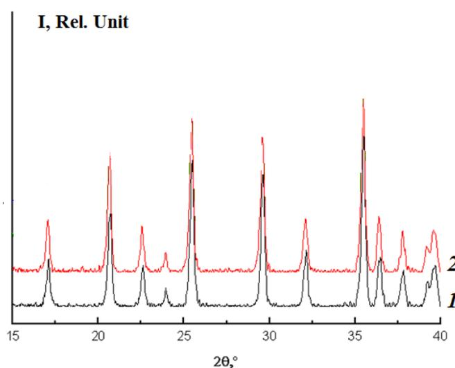
**Figure 1.** Fragments of diffraction patterns: 1 –  $\text{LiFePO}_4/\text{C}$ ; 2 –  $\text{Li}_{0.99}\text{Fe}_{0.98}\text{Ni}_{0.01}\text{Cr}_{0.01}\text{PO}_4/\text{C}$ .
