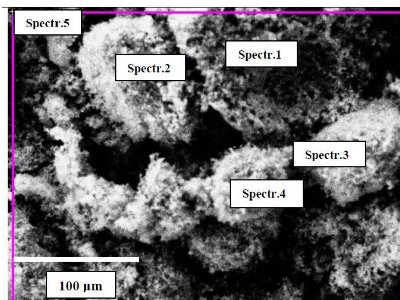
Figure 4. Electronic image of Li<sub>0.99</sub>Fe<sub>0.98</sub>Ni<sub>0.01</sub>Cr<sub>0.01</sub>PO<sub>4</sub>/C, the areas where the EDX microanalysis was performed are marked with a rectangles.
