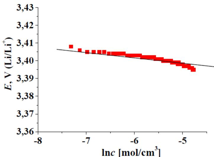
**Figure 10.** Dependence of the electrode potential based on  $Li_{0.99}Fe_{0.98}Cr_{0.01}Ni_{0.01}PO_4/C$  on the lithium concentration (cathode curve adjustment)
