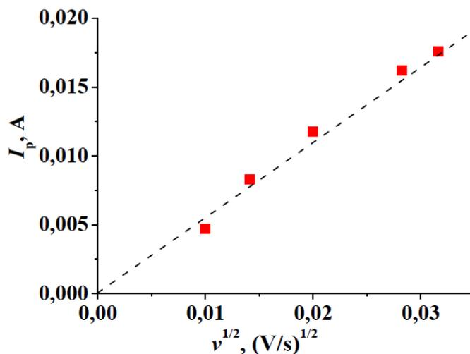
**Figure 9.** Dependence of the cathode current in the maximum of the voltamogram on the square root of the potential scan rate.
