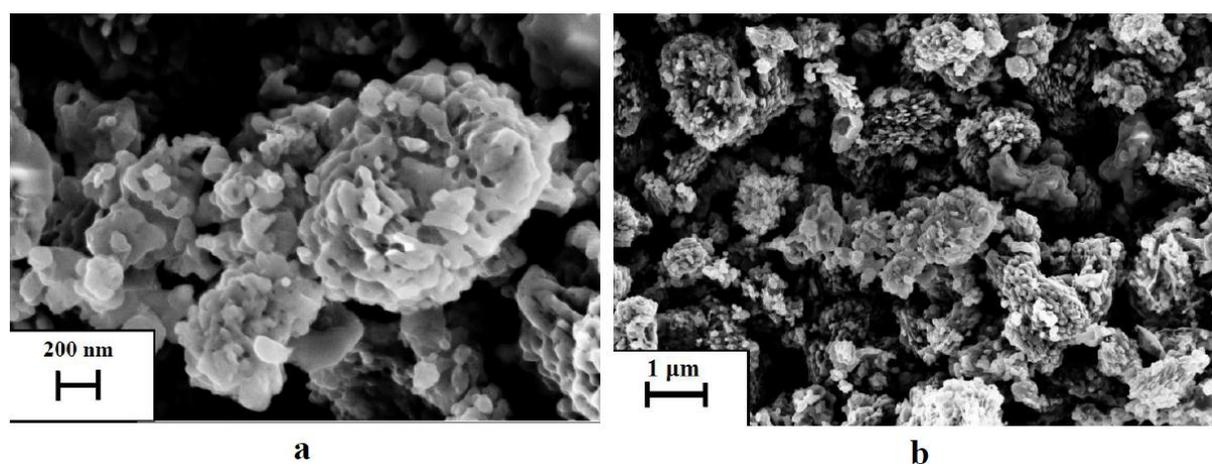
Figure 3. SEM micrographs of Li<sub>0.99</sub>Fe<sub>0.98</sub>Ni<sub>0.01</sub>Cr<sub>0.01</sub>PO<sub>4</sub>/C taken at different magnification (a, b).
