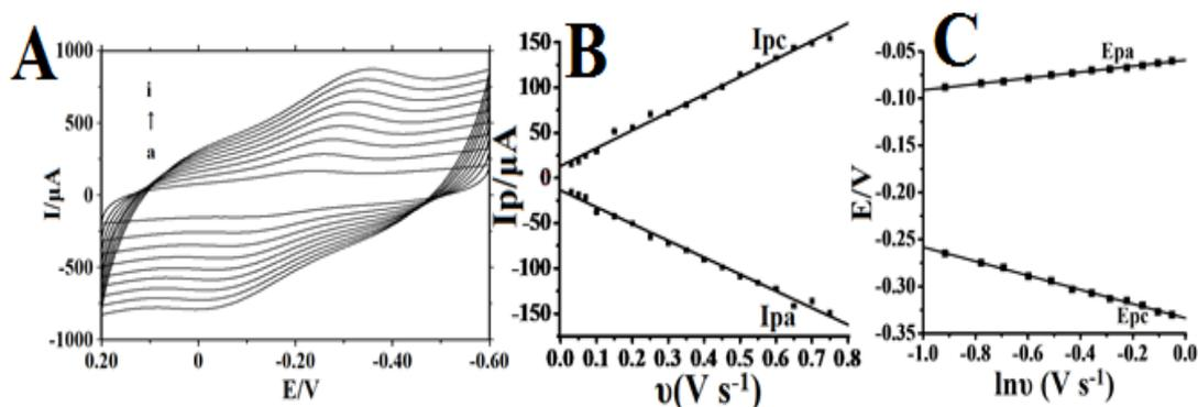
**Figure 3.** (A) Effect of scan rates ( $v$ ) (from a  $\rightarrow$  i as 100, 200, 300, 400, 500, 600, 700, 800, 900  $\text{mV s}^{-1}$ ) on electrochemical responses of Nafion/Mb/Bi/GR/CILE in pH 3.0 PBS; (B) Plot of the redox peak currents against  $v$ ; (C) Plot of the redox peak potentials against  $\ln v$ .
