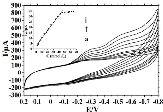
**Figure 4.** CV of Nafion/Mb/Bi/GR/CILE with 2, 4, 8, 18, 26, 30, 38, 46, 59, 65 mmol L<sup>-1</sup> TCA (curves a → j), scan rate: 0.1 V s<sup>-1</sup> (Inset was the linearity of catalytic reduction currents and TCA concentration).
