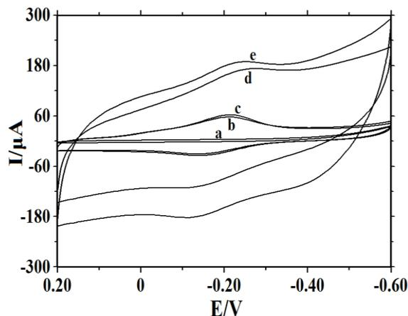
**Figure 2.** CV of (a) Nafion/CILE, (b) Nafion/Mb/CILE, (c) Nafion/Mb/Bi/CILE, (d) Nafion/Mb/GR/CILE and (e) Nafion/Mb/Bi/GR/CILE in pH 3.0 PBS, scan rate: 0.1 V s<sup>-1</sup>.
