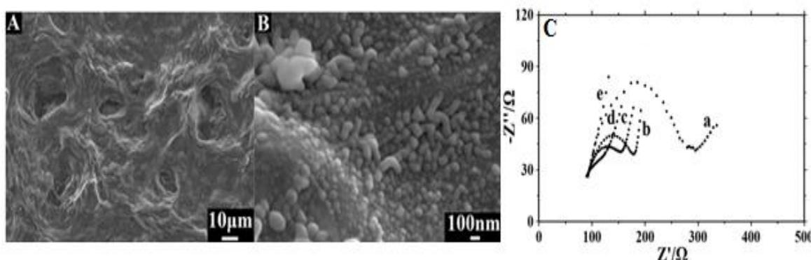
**Figure 1.** SEM images of GR/CILE (A) and Bi/GR/CILE (B); (C) EIS of (a) Nafion/Mb/CILE, (b) Nafion/CILE, (c) Nafion/Mb/Bi/CILE, (d) Nafion/Mb/GR/CILE and (e) Nafion/Mb/Bi/GR/CILE in a  $10.0 \text{ mmol L}^{-1} [\text{Fe}(\text{CN})_6]^{3-/4-}$  and  $0.1 \text{ mol L}^{-1} \text{ KCl}$  solution with the frequencies from  $10^4$  to  $10^{-1} \text{ Hz}$ .
