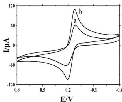
**Figure 2.** Cyclic voltammograms of  $5.0 \times 10^{-4} \text{ mol L}^{-1}$  metal on (a) CILE and (b) CTS-TiO<sub>2</sub>/CILE in pH 5.0 B-R buffer solution with the scan rate of  $100 \text{ mV s}^{-1}$ .
