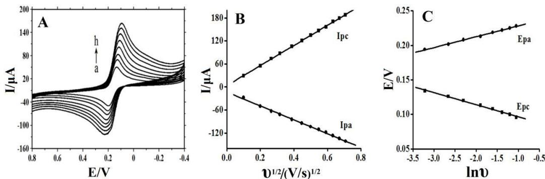
**Figure 4.** (A) Cyclic voltammograms of  $5.0 \times 10^{-4}$  mol L<sup>-1</sup> metal on CTS-TiO<sub>2</sub>/CILE with different scan rates (a–h: 40, 70, 100, 150, 200, 250, 300, 350 mV s<sup>-1</sup>) in pH 5.0 B-R; (B) Linear relationship of  $I_{pc}$  and  $I_{pa}$  with  $v^{1/2}$  in the range from 40 to 350 mV s<sup>-1</sup>; (C) Linear relationship of  $E_{pa}$  and  $E_{pc}$  with  $\ln v$ .
