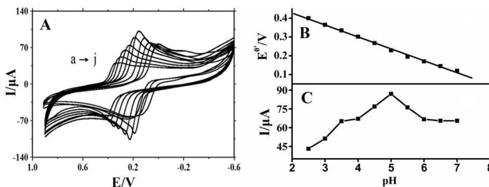
**Figure 3.** (A) Cyclic voltammograms of  $5.0 \times 10^{-4} \text{ mol L}^{-1}$  metal on CTS-TiO<sub>2</sub>/CILE with different pH values (from a to j are 2.5, 3.0, 3.5, 4.0, 4.5, 5.0, 5.5, 6.0, 6.5, 7.0) at the scan rate of  $100 \text{ mV s}^{-1}$ ; (B) Relationship between the formal peak potential ( $E^0$ ) and buffer pH; (C) Relationship of the oxidation peak current ( $I_{\text{pa}}$ ) with buffer pH.
