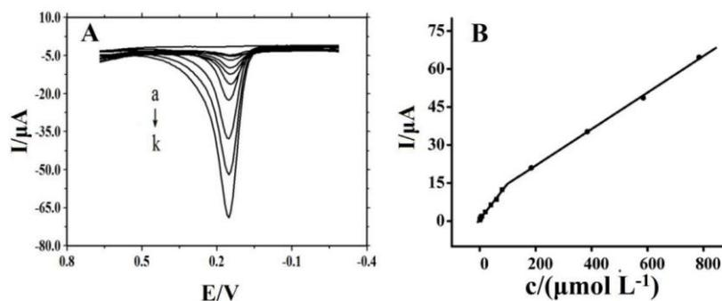
**Figure 5.** (A) DPV of metal with increasing concentration (a–k: 0.0, 6.0, 8.0, 20.0, 40.0, 60.0, 80.0, 200.0, 400.0, 600.0, 800.0 μmol L<sup>-1</sup>); (B) The relationship of the oxidation peak current with metal concentration.
